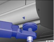
Fig. 137 Lifting points at front for the lifting platform or vehicle jack
