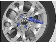
Fig. 156 Changing a wheel: removing the wheel bolts with the screwdriver handle
