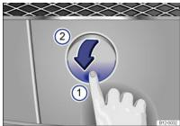
Fig. 173 On the right-hand side of the front bumper: releasing and removing the cover
