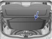
Fig. 146 In the luggage compartment: floor covering held in upright position
