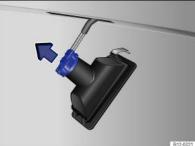
Fig. 168 Number plate light: removing the bulb holder
