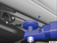
Fig. 138 Lifting points at rear for the lifting platform or vehicle jack
