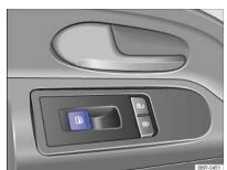
Fig. 30 In the front doors: buttons for the electric window
