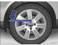
Fig. 152 Changing a wheel: loosening the wheel bolts
