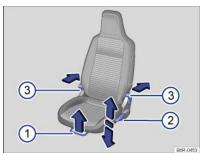
Fig. 37 Front left-hand seat controls
