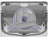
Fig. 76 In the luggage compartment: fastening rings
