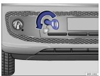
Fig. 174 Front bumper, right-hand side: screwing in the towing eye
