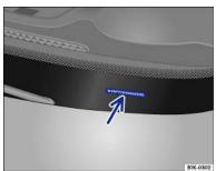
Fig. 14 Vehicle identification number
