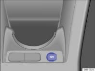
Fig. 92 Front centre console: 12-volt socket in the stowage compartment
