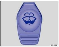
Fig. 68 In the engine compartment: cap of washer fluid reservoir
