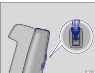
Fig. 60 Example of a fastened top tether
