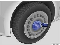
Fig. 149 Pulling off the centre cover on a steel wheel
