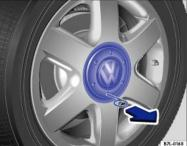
Fig. 148 Pulling off the centre cover on an alloy wheel
