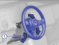
Fig. 40 Adjusting the steering wheel position mechanically
