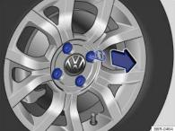
Fig. 151 Removing the wheel bolt caps
