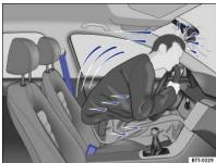
Fig. 46 An unbelted driver is thrown forwards
