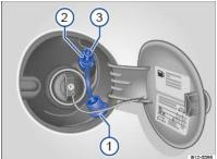
Fig. 118 With the tank flap open: tank cap ①, gas filler neck ②, gas filler neck seal ③
