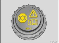
Fig. 101 In the engine compartment: cap on the brake fluid container
