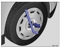
Fig. 150 Removing the wheel covers
