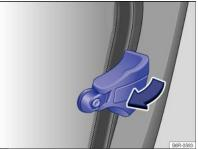
Fig. 31 In the rear doors: opening the hinged windows
