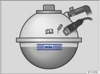
Fig. 123 In the engine compartment: marking on the coolant expansion tank
