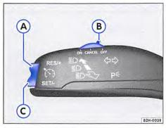
Fig. 236 On the left of the steering column: buttons and switch for setting the CCS in the turn signal and main beam lever (vehicles without multifunction steering wheel).
