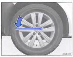
Fig. 297 Loosening the wheel bolts for changing the wheels.
