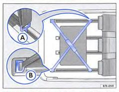
Fig. 109 Load secured correctly using 2 securing straps
