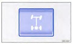
Fig. 229 On the dash panel: button for rear axle differential lock
