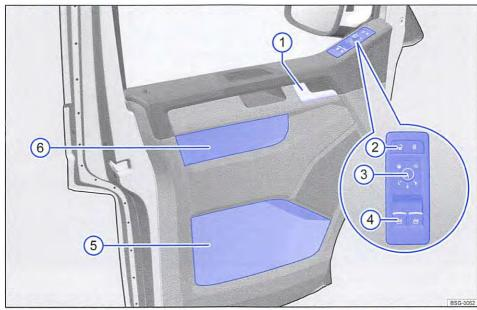
Fig. 5 Overview of the controls in the driver door (left-hand drive vehicles). The controls are mirrored in right-hand drive vehicles.
