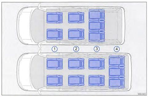
Fig. 41 Overview of seats: short wheelbase (top), long wheelbase (bottom).
