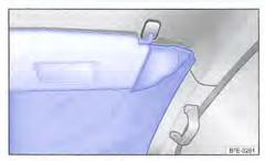
Fig. 179 On the sun visor: attaching the removable opaque shades for the windscreen.
