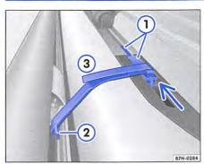
Fig. 187 On the pop-up roof: fully secured manually with Velcro straps (right side of vehicle).
