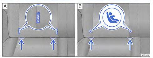
Fig. 79 On vehicle seat: different markings identifying the ISOFIX anchoring points for child seats.
