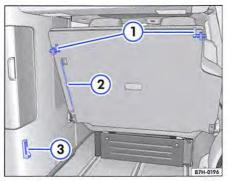
Fig. 158 In the luggage compartment: lever ①, support rod ② and retainer ③.
