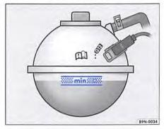
Fig. 277 In the engine compartment: markings on the coolant expansion tank.
