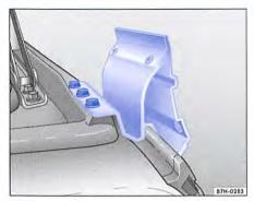
Fig. 191 Three bolts on top in the awning bracket.
