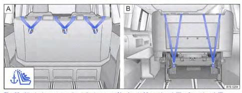
Fig. 80 Attached upper strap (top tether) on rear of backrest of 3-seat bench A or 2-seat bench B.
