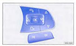
Fig. 16 Right-hand side of the multifunction steering wheel: controls for the menus in the instrument cluster.
