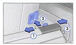
Fig. 106 In the luggage compartment: retainer for the luggage compartment cover
