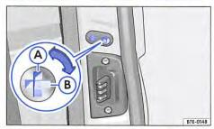
Fig. 29 In the left sliding door: childproof lock - (A) switched off, (B) switched on
