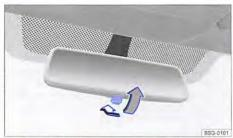
Fig. 99 On the windscreen: manual anti-dazzle interior mirror.
