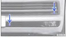
Fig. 231 In the front bumper: ParkPilot sensors.
