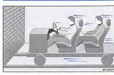
Fig. 60 Unbelted occupants in a vehicle heading for a brick wall.
