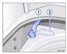
Fig. 203 In the rear stowage compartment under the shelve: closed ① or opened ② valve of the fresh water tank.
