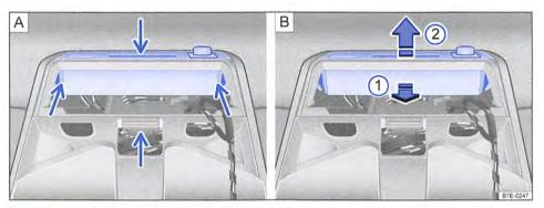
Fig. 185 Removing the central control panel
