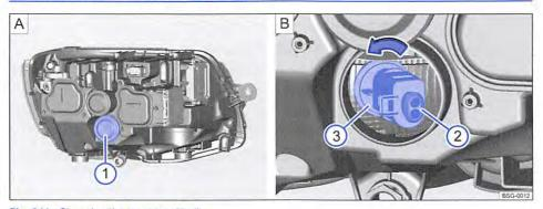
Fig. 311 Changing the turn signal bulb.
