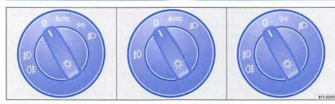
Fig. 86 Next to the steering wheel: examples of the various light switches.
