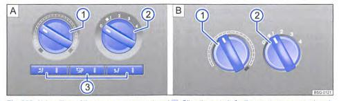
Fig. 255 In headliner of the passenger compartment A: Climatic controls for the passenger compartment. In the centre console B: controls of the heating and fresh air system for the passenger compartment.
