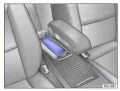
Fig. 152 In the armrest of the 2-seat arrangement: telephone handset for the rear-seat telephony system.
