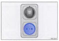
Fig. 211 At the side behind the left front seat: 230-volt grounded safety socket.
