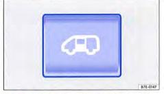
Fig. 28 On the dash panel: button for locking the electric sliding door(s)
