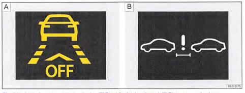
Fig. 244 In the instrument cluster display: A Front Assist deactivated. B Distance warning lamp.
