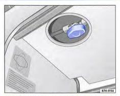
Fig. 201 Open gas shut-off valve in the kitchen unit underneath the gas cooker
