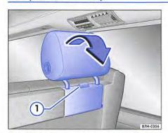
Fig. 156 Folding down the head restraint of the bench seat/bed.
