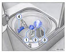
Fig. 199 Connected gas bottle with bottle safety valve and pressure regulator
