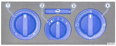
Fig. 258 In the centre console: controls for the heating and fresh air system.
