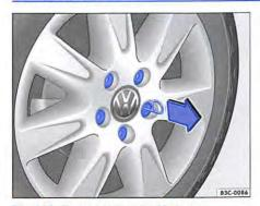
Fig. 296 Removing the wheel bolt caps.
