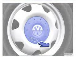
Fig. 294 Removing the centre covers by pulling.
