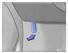
Fig. 272 The bonnet release lever is located in the driver side footwell.
