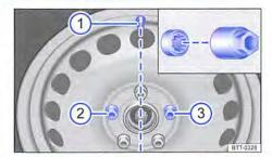
Fig. 298 Tyre valve 1 and locations of the antitheft wheel bolt 2 or 3
