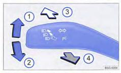
Fig. 85 Turn signal and main beam lever in the basic position.
