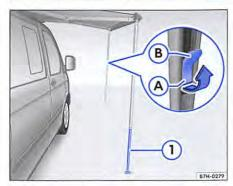
Fig. 189 Secure fitting of the open awning
