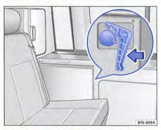
Fig. 194 In the living area: work table in stowed position and release lever (close-up).
