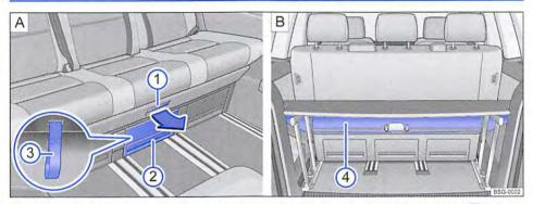
Fig. 162 In the living area and the luggage compartment: controls on the 3-seat bench at front A and on the multi-flex board B.
