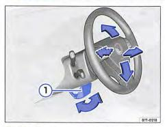
Fig. 46 Below the steering wheel: lever for mechanical adjustment in the steering column trim.
