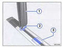
Fig. 110 T-shaped fastening ring fitted correctly in the seat rail
