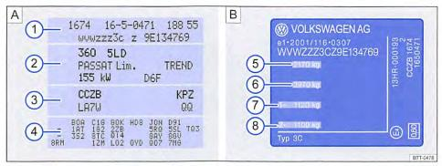
Fig. 322 A: Vehicle data sticker: example shows a vehicle with engine code CCZB 3. B: type plate.
