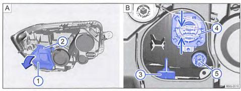
Fig. 309 Changing the dipped beam bulb, the side light bulb and the turn signal bulb.
