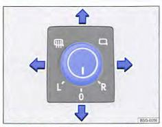
Fig. 100 In the driver door: rotary knob for the exterior mirrors.
