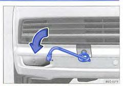
Fig. 321 Front bumper, right-hand side: screwing in the towing eye.
