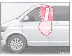
Fig. 75 Schematic diagram: deployment range of the combined curtain and side airbag on left side of vehicle
