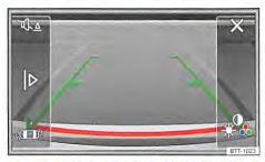
Fig. 234 Infotainment system: screen display from the switched on reversing camera.
