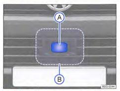
Fig. 240 In the ventilation grille under the Volkswagen badge: radar sensor (A) and area around the radar sensor to be kept clear (B).
