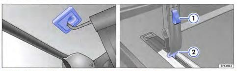
Fig. 112 Correctly fitted net partition in the headliner and in the seat rail
