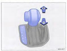
Fig. 222 Selector lever in Tiptronic position (lefthand drive). The controls are mirrored for righthand drive vehicles.
