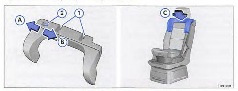
Fig. 83 Fit the lateral head restraint for the integrated child seat for goup 2 children.
