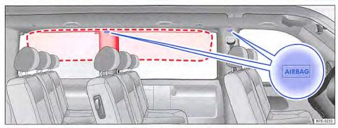
Fig. 76 Location and deployment zone of the curtain airbags on the left side of the vehicle.
