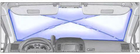
Fig. 140 Fitted opaque shade for the windscreen
