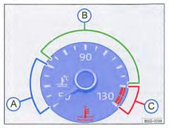
Fig. 276 In the instrument cluster: coolant temperature display with cold range (A), normal range (B) warning range (C).
