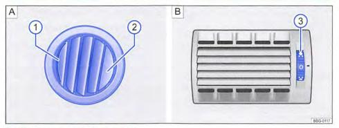
Fig. 260 Types of vents in the headliner
