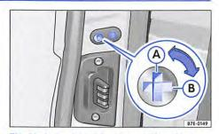
Fig. 30 In the right sliding door: childproof lock - (A) switched off, (B) switched on
