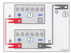
Fig. 318 How to connect the jump leads in starting vehicles without start/stop system: discharged battery ① and battery providing assistance ②.
