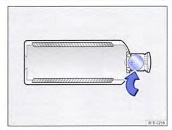
Fig. 134 Replacing the battery of the remote control.
