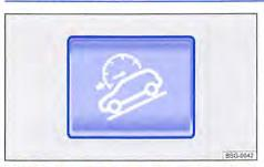
Fig. 228 In the centre console: button for switching the Hill Descent Assist on and off.
