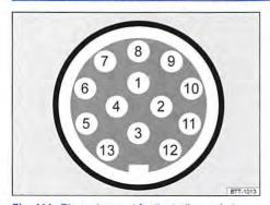
Fig. 114 Pin assignment for the trailer socket.
