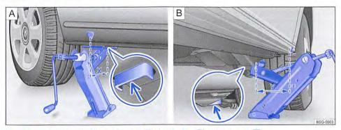
Fig. 300 On the left side of the vehicle: jack fitted at the front A and at the rear B.
