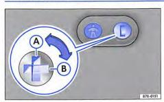
Fig. 36 In the left-hand wing door: childproof lock - (A) switched off. (B) switched on
