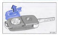
Fig. 20 Opening the battery case cover
