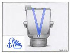
Fig. 81 Attached upper strap (top tether) on rear of backrest of single seat.
