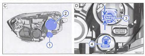
Fig. 310 Changing the main beam bulb and daytime running light bulb.
