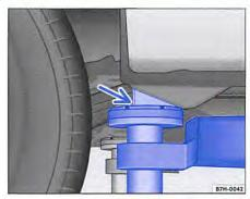
Fig. 288 Lifting points at rear for the lifting platform or vehicle jack.
