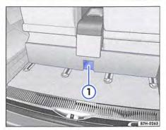
Fig. 148 In the luggage compartment: release lever of the 2-seat arrangement.
