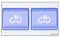
Fig. 262 On the dash panel: buttons for the roof ventilator
