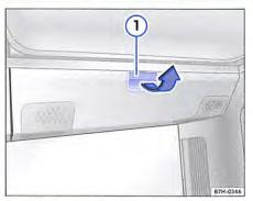
Fig. 176 Opening the stowage compartment in the headliner
