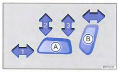
Fig. 43 On the outer side of the left front seat: adjusting the backrest and the seat cushion for height and tilt.
