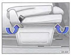
Fig. 54 Holding points for removal and installation on 3-seat bench.
