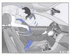
Fig. 63 The unbelted rear passenger is thrown forwards, hitting the belted driver.
