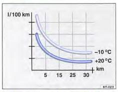
Fig. 226 Fuel consumption in litres per 100 km at two different outside temperatures.
