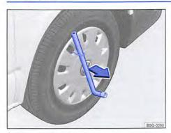
Fig. 295 Removing the wheel covers,
