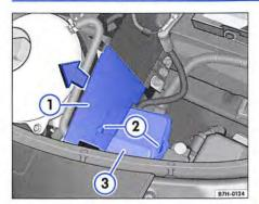
Fig. 304 In the engine compartment: fuse box cover.
