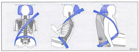
Fig. 67 Correct seat belt routing and head restraint adjustment.
