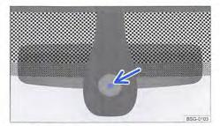
Fig. 96 On the inside of the windscreen above the interior mirror: sensitive surface of the rain sensor
