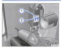
Fig. 212 Under the rear side trim panel: switched on residual current circuit breaker with test button
