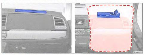
Fig. 72 Location and deployment zone of the front passenger front airbag.
