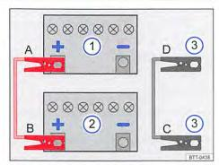
Fig. 319 How to connect the jump leads in starting vehicles with start/stop system: discharged battery (1) and battery providing assistance (2).
