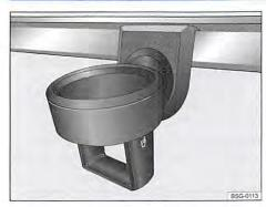
Fig. 178 In the living area: drink holder attached in aluminium rail.
