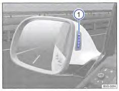
Fig. 248 Display in the exterior mirror
