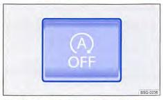
Fig. 227 In the centre console: button for the start/stop system.
