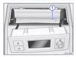
Fig. 186 Manual closing of the pop-up roof with the central control panel removed
