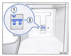
Fig. 213 In the rear left stowage area: switched on residual current circuit breaker with test button and bridge connection 2 on vehicles with cupboards.
