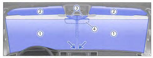
Fig. 180 On the windscreen: attaching the integrated opaque shade.
