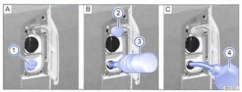
Fig. 271 Behind the tank flap: filler cap of the AdBlue tank unscrewed (a) and attached in holder (b) (2). Fill the AdBlue tank using a filler bottle (b) (a) or a filler nozzle (c) (4).
