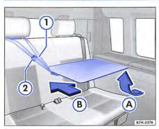
Fig. 196 Loop strap of the work table.
