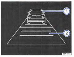
Fig. 238 On the instrument cluster display; adaptive cruise control (ACC) deactivated temporarily; vehicle detected ahead, time interval set
