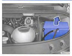
Fig. 279 Engine compartment: pushing up the vehicle battery sleeve.
