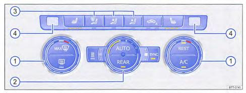
Fig. 256 In the centre console: Climatronic controls.
