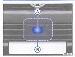
Fig. 246 In the bumper under the Volkswagen badge: radar sensor (A) and area around the radar sensor to be kept clear (B).
