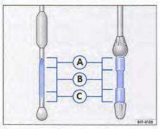
Fig. 274 Oil dipstick with markings.
