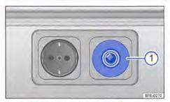
Fig. 207 There is a 12-volt socket ① on the side of the kitchen unit
