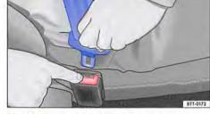
Fig. 66 Removing the latch plate from the buckle.
