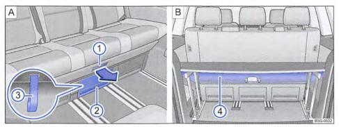
Fig. 161 In the living area and the luggage compartment: controls on the 3-seat bench at front A and on the multi-flex board B.
