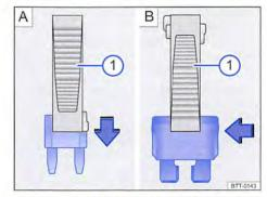
Fig. 306 Removing or fitting a fuse using the plastic pliers ①.
