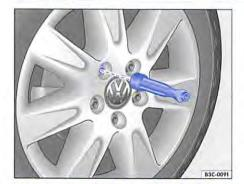
Fig. 301 removing the wheel bolts with the screwdriver handle.
