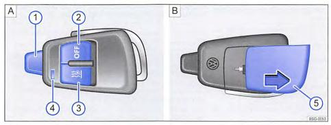
Fig. 266 Remote control for the auxiliary air heater.
