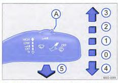
Fig. 92 Next to the steering wheel: wiper lever for operating the front wipers.
