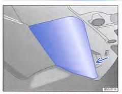
Fig. 303 At the bottom of the centre console: fuse box cover.
