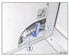
Fig. 205 In the kitchen unit; closed ① or opened ② valve of the fresh waste water tank.
