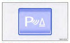
Fig. 230 In the centre console: button for switching the ParkPilot on and off
