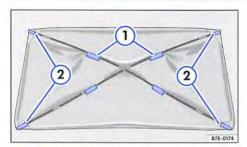
Fig. 138 Assembled opaque shade for the windscreen
