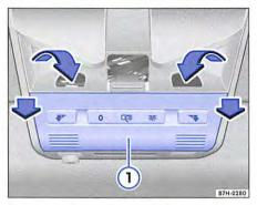
Fig. 184 Removing the cover on the interior lights control panel
