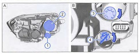
Fig. 308 Changing the daytime running light bulb and the turn signal bulb.
