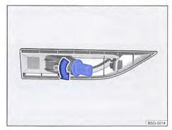
Fig. 317 Changing the bulbs in the turn signal repeater.
