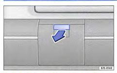
Fig. 122 In the rear side panel: folding table cover
