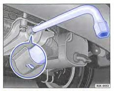
Fig. 283 Underneath the vehicle: spare wheel bracket with box spanner inserted
