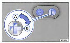
Fig. 34 On the front of the tailgate: childproof lock - (A) switched off, (B) switched on
