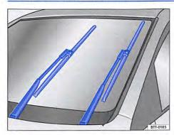
Fig. 94 Wiper blades in service position.
