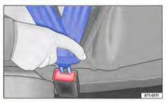
Fig. 65 Inserting the seat belt latch plate into the buckle.
