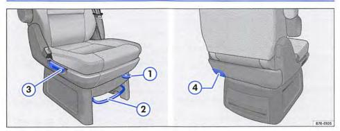
Fig. 51 In the passenger compartment: controls on the front left and the rear right of the single seat.
