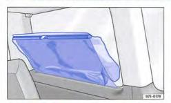
Fig. 142 Fitting the opaque shades to the side windows
