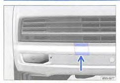
Fig. 320 On the right side of the front bumper: cover for towing eye on unpainted bumper.
