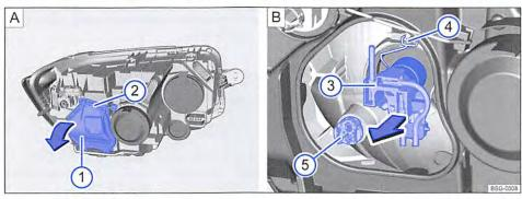
Fig. 307 Changing the dipped beam and main beam bulb and the side light bulb.
