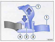
Fig. 101 Fastening the buckle strap
