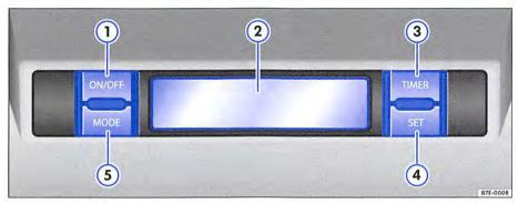
Fig. 264 In the headliner: controls of the supplementary heating system
