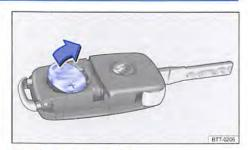
Fig. 21 Removing the battery
