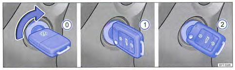
Fig. 217 Positions of the vehicle key in the ignition lock.
