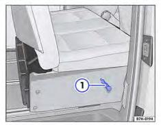
Fig. 155 Locking mechanism in the bench seat/ bed blocked by a screwdriver (1).
