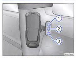
Fig. 151 In the passenger compartment: telephone holder for rear-seat telephony system.
