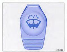
Fig. 97 In the engine compartment: cap of washer fluid reservoir.
