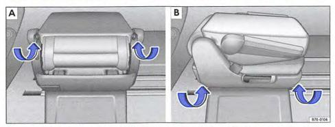
Fig. 52 Holding points for removal and installation on rotating single seat A and on non-rotating single seat B
