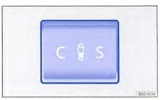
Fig. 252 In centre console: button for setting the adaptive chassis control.
