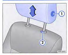
Fig. 45 Adjusting the head restraint
