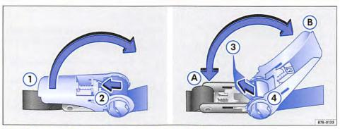
Fig. 103 Releasing and tightening the lever on the ratchet strap.
