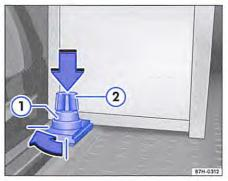
Fig. 175 In the luggage compartment: fixing the stowage box with handle (1) and thumb wheel (2)
