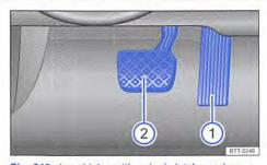
Fig. 219 In vehicles with a dual clutch gearbox, accelerator pedal ① and brake pedal ②.
