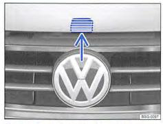
Fig. 273 On the front edge of the bonnet: release lever for opening.
