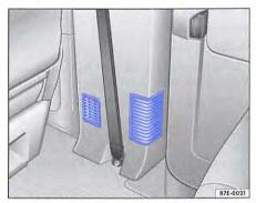
Fig. 265 In the passenger compartment: vent for auxiliary air heater.
