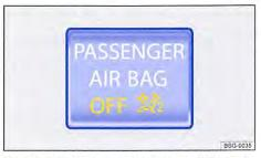
Fig. 70 Indicator lamp in the dash panel for deactivated front passenger front airbag
