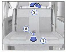
Fig. 157 Converting the bench seat/bed to a bed.
