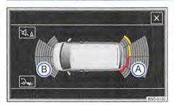
Fig. 232 ParkPilot screen display (colour display).
