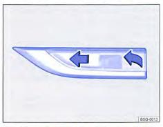
Fig. 316 On the side of the vehicle: removing the turn signal repeater.
