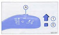
Fig. 95 Next to the steering wheel: adjusting rain sensor (A) in wiper lever.
