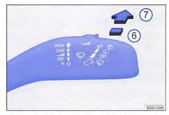
Fig. 93 Next to the steering wheel: wiper lever for operating the rear wiper.
