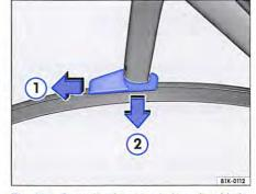
Fig. 286 Changing the rear window wiper blade.
