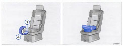
Fig. 82 Fold out the seat padding of the integrated child seat.
