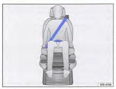
Fig. 84 Seat belt routing on the integrated child seat.
