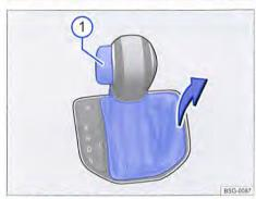
Fig. 292 Removing the cover of the gearshift gate.
