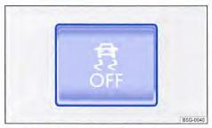
Fig. 224 In the centre console: button for switching the TCS on and off manually.
