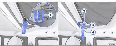
Fig. 181 In the headliner: detach the hook of the retaining strap (left) and release the catches of the roof shell (right).
