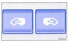
Fig. 27 On the dash panel and in the remote control key: button for opening and closing an electric sliding door
