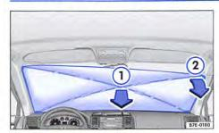
Fig. 144 Removing the opaque shade from the windscreen
