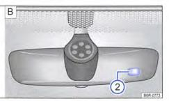
Fig. 98 On the windscreen: automatic anti-dazzle interior mirror.
