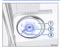
Fig. 204 In the rear stowage compartment under the shelve: opening for cleaning the fresh water tank.
