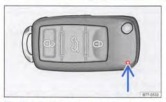
Fig. 19 Indicator lamp in remote control key
