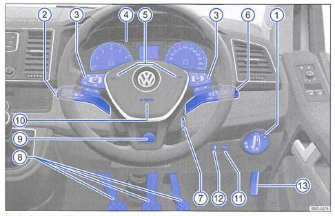
Fig. 7 Overview of the driver side (right-hand drive vehicles with comfort dash panel).
