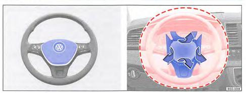
Fig. 71 Location and deployment zone of the driver front airbag.
