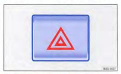
Fig. 289 In the middle of the dash panel: hazard warning light switch.
