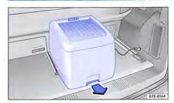
Fig. 126 Removing the cool box.
