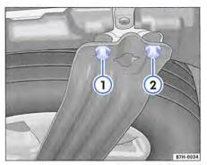
Fig. 282 Underneath the vehicle: retaining bolt 1 and securing bolt 2 on the spare wheel bracket
