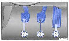
Fig. 218 In vehicles with a manual gearbox, accelerator pedal ①, brake pedal ② and clutch pedal ③.
