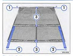
Fig. 111 Folding out the net partition
