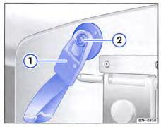
Fig. 197 Securing the work table to the head restraint.
