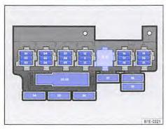
Fig. 214 Under the left front seat: fuse box.
