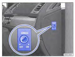
Fig. 73 On the front of the dash panel: key switch for disabling and enabling the front airbag on the front passenger side
