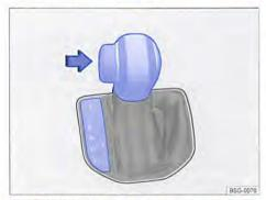
Fig. 221 Selector lever for automatic gearbox with lock button (arrow) in left-hand drive vehicles. The controls are mirrored for right-hand drive vehicles.
