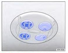
Fig. 263 In the headliner: roof ventilator
