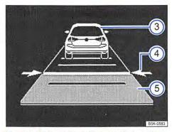
Fig. 239 On the instrument cluster display: adaptive cruise control (ACC) active: vehicle detected ahead, time interval is being set
