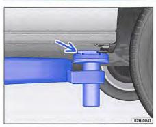
Fig. 287 Lifting points at front for the lifting platform or vehicle jack.
