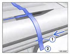
Fig. 188 On the pop-up roof: preparation to fully secure the pop-up roof manually from the outside (right side of vehicle).
