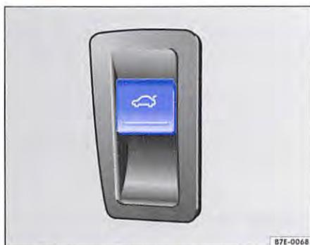
**Fig. 33** Inside tailgate: button in vehicles with central locking and electrical unlocking for the tailgate
