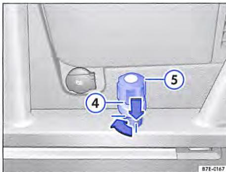
Fig. 57 In the luggage compartment: multi-flex board in right seat rail with handle 4 and thumb wheel 5
