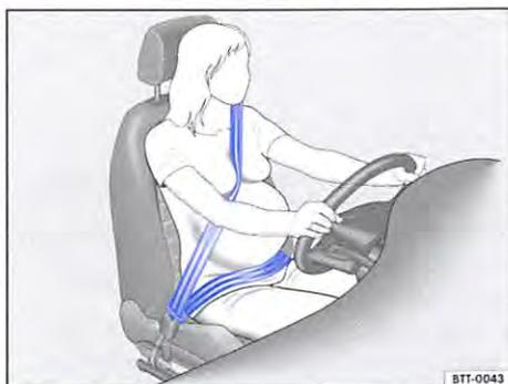
Fig. 68 Correct seat belt routing during pregnancy.
