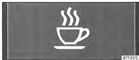
Fig. 251 On the instrument cluster display: Driver Alert System.
