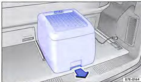
Fig. 126 Removing the cool box.
