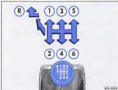
Fig. 220 Gear shift pattern of a 5 or 6-speed manual gearbox
