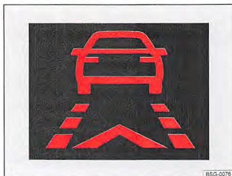
Fig. 245 The display in the instrument cluster: advance warning display.
