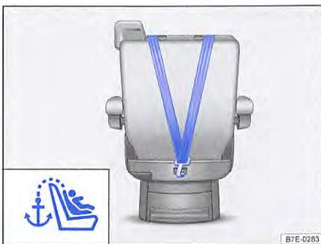
Fig. 81 Attached upper strap (top tether) on rear of backrest of single seat.
