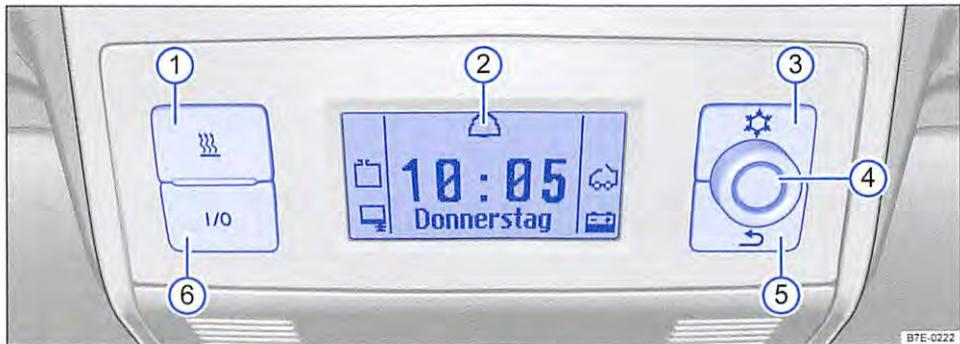
Fig. 168 In the headliner: central control panel with the initial screen
