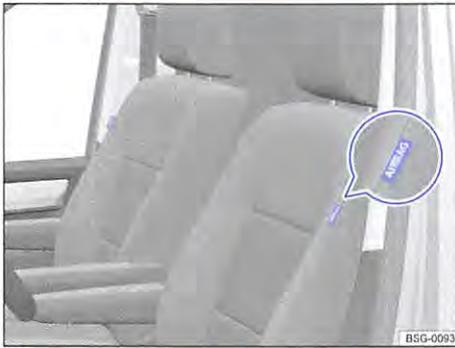
**Fig. 74** On the side of the front seat: location of the combined curtain and side airbag.
