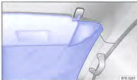
**Fig. 179** On the sun visor: attaching the removable opaque shades for the windscreen.
