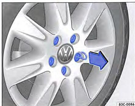
Fig. 296 Removing the wheel bolt caps.
