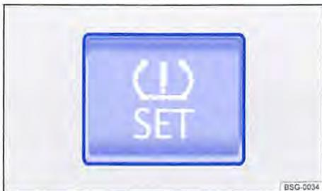
**Fig. 253** In the stowage compartment on the front passenger side: button for the tyre monitoring system.
