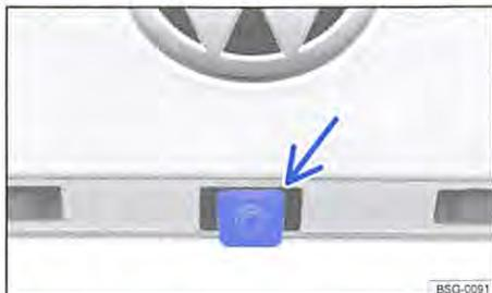
**Fig. 233** In the tailgate: location of the rear view camera system.
