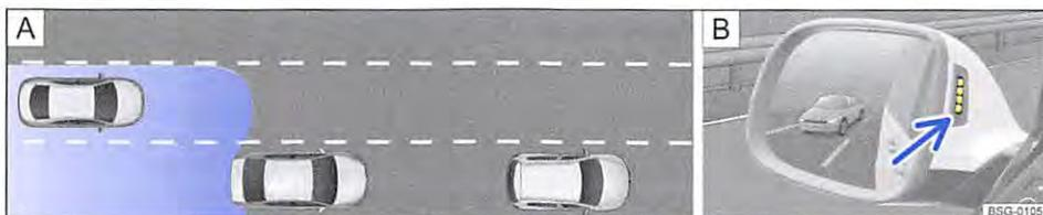
**Fig. 249** **A** Driving situation when overtaking with traffic behind the vehicle **B** Visual display in the left-hand exterior mirror.
