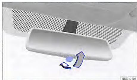
Fig. 99 On the windscreen: manual anti-dazzle interior mirror.
