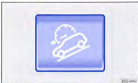
**Fig. 228** In the centre console: button for switching the Hill Descent Assist on and off.
