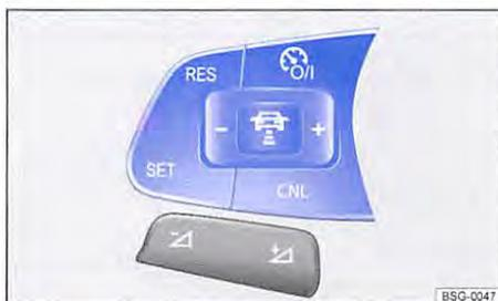
Fig. 237 Left-hand side of the multifunction steering wheel: buttons for operating the CCS.
