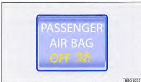
**Fig. 70** Indicator lamp in the dash panel for deactivated front passenger front airbag
