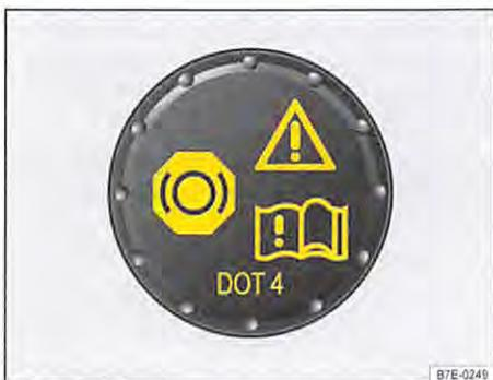
Fig. 225 In the engine compartment: cap on the brake fluid container.
