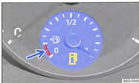
Fig. 269 In the instrument cluster: fuel gauge for petrol and diesel.
