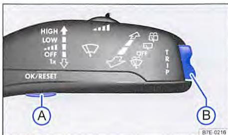
**Fig. 15** In wiper lever: control buttons for menus in the instrument cluster (vehicles without multifunction steering wheel).
