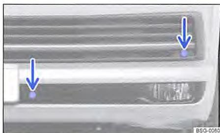
**Fig. 231** In the front bumper: ParkPilot sensors.
