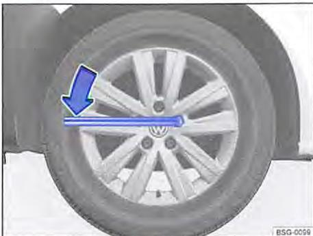
Fig. 297 Loosening the wheel bolts for changing the wheels.
