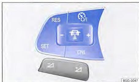
**Fig. 241** Left-hand side of the multifunction steering wheel. buttons for operating the adaptive cruise control (ACC)
