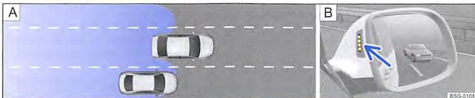
**Fig. 250** **A** Driving situation when overtaking and pulling in. **B** Visual display in the right-hand exterior mirror.
