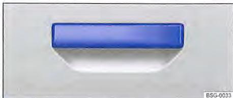
Fig. 31 Opening the tailgate from the outside.
