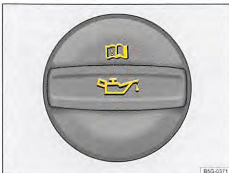
Fig. 275 In the engine compartment: engine oil filler cap (illustration).
