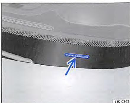
Fig. 323 In the windscreen: vehicle identification number.
