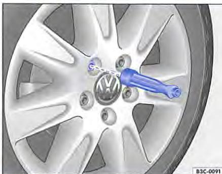
Fig. 301 removing the wheel bolts with the screwdriver handle.
