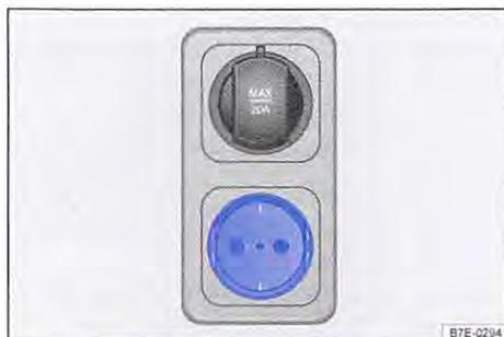
**Fig. 211** At the side behind the left front seat: 230-volt grounded safety socket.
