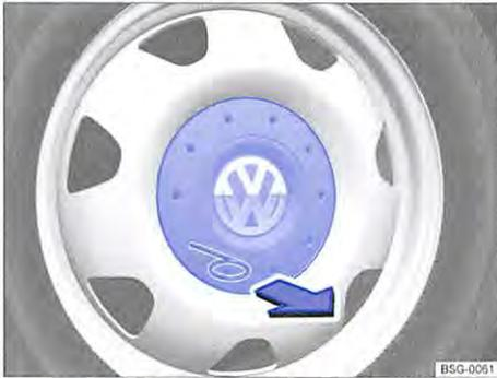
Fig. 294 Removing the centre covers by pulling.
