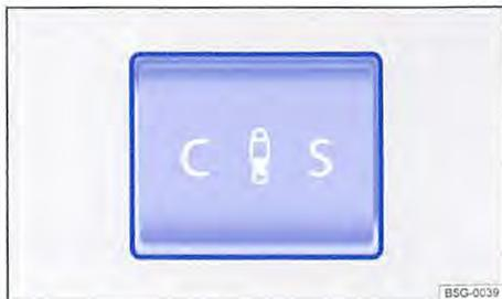
Fig. 252 In centre console: button for setting the adaptive chassis control.
