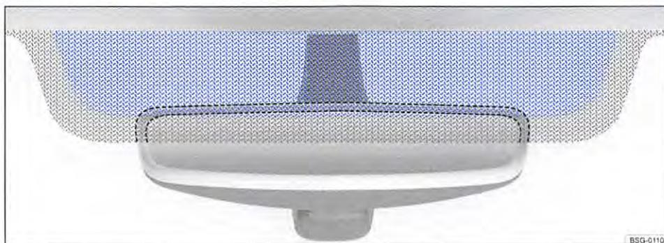
Fig. 91 Metal-coated windscreen for infrared reflection with communication window (blue area).
