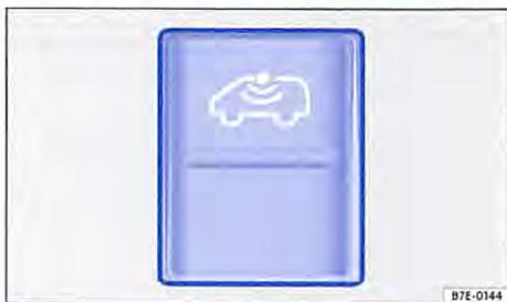
**Fig. 25** Next to the driver seat: button for switching off the interior monitoring system and anti-tow alarm.
