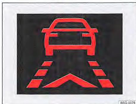
Fig. 247 The display in the instrument cluster: advance warning display.
