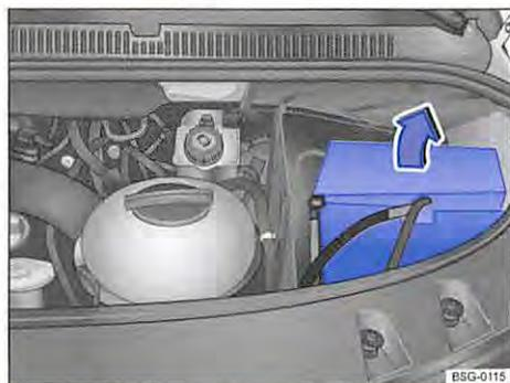
**Fig. 279** Engine compartment: pushing up the vehicle battery sleeve.
