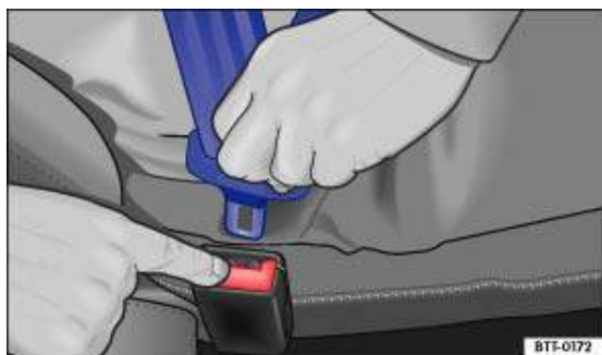
Fig. 55 Removing the latch plate from the buckle
