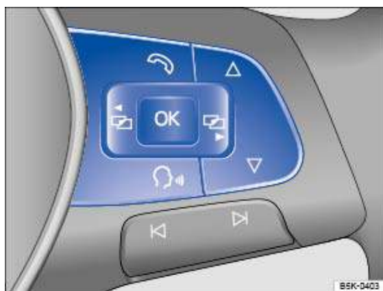
Fig. 16 Right-hand side of the multifunction steering wheel: controls for using the menus and information displays in the instrument cluster
