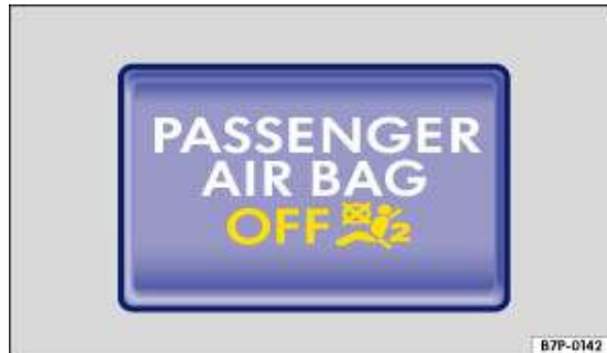
Fig. 59 In the upper section of the centre console: indicator lamp for disabled front passenger front airbag
