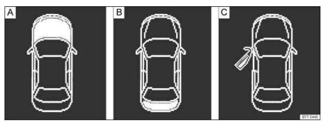
Fig. 12 In the instrument cluster display: A: Open engine hood, B: Open luggage compartment lid, C: Open
