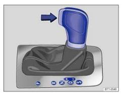
Fig. 128 Side view: Automatic transmission selector lever with shift lever release button (arrow).
