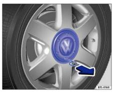
Fig. 180 Pulling the hubcap off.
