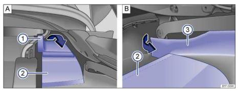
Fig. 169 Right side of luggage compartment: Remove cover.
