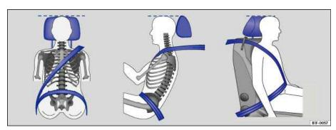
Fig. 61 Proper safety belt positioning and head restraint adjustment.
