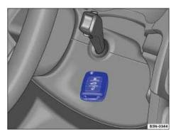
Fig. 126 Hold the remote control vehicle key to the right of the steering column: Emergency starting feature
