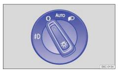
Fig. 83 Headlight switch next to the steering wheel.
