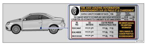
Fig. 104 On the driver door jamb: Location of the tire inflation pressure label.
