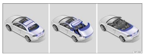
Fig. 31 The CSC roof folds down into the luggage compartment when you open the roof (put the roof down).
