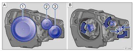
Fig. 192 In the engine compartment: Covers in the left headlight assembly. 1 Low beam, 2 Turn signal indicator, 3 High beam and parking light as well as daytime running light.
