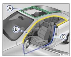
Fig. 160 Care of rubber seals: A power sunroof seals; B power window seals; C seals on the doors.
