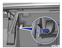
Fig. 98 Removing the inside luggage compartment cover.
