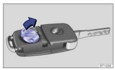
Fig. 22 Remote control vehicle key: Remove old battery.
