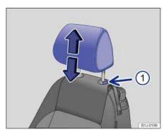
Fig. 46 Adjusting the front head restraints.
