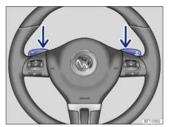
Fig. 131 Steering wheel with optional Tiptronic shift paddles.
