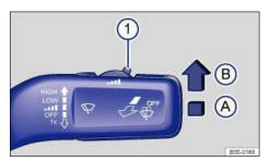
Fig. 89 Windshield wiper lever: Adjusting rain sensor 1.
