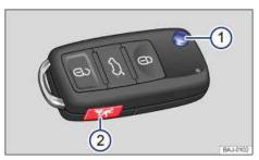
Fig. 18 Remote control vehicle key with panic button.
