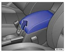
Fig. 113 In the front center armrest: Storage compartment.
