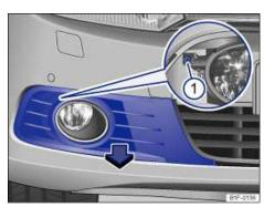
Fig. 193 In front right bumper: Removing the light assembly.
