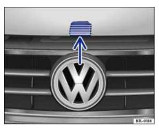
Fig. 151 Above the radiator grille: Outside engine hood release.
