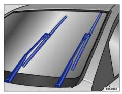
Fig. 88 Windshield wiper in service position.
