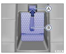
Fig. 100 From the passenger compartment: Opening the pass-through panel into the luggage compartment.
