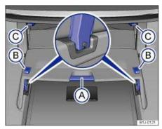
Fig. 97 Lifting up the inside luggage compartment cover.
