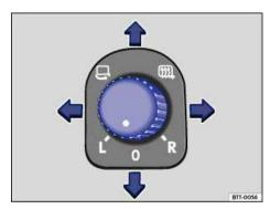
Fig. 94 In the driver door: Adjusting knob for the outside mirrors.
