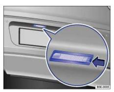
Fig. 195 In the rear bumper: License plate light.
