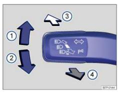
Fig. 82 Turn signal lever and high beam switch.
