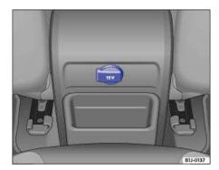
Fig. 123 Rear center console: 12 Volt socket.
