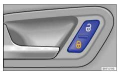
Fig. 24 In the vehicle doors: Power locking button.
