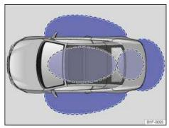
**Fig. 25** Ranges of the Keyless Access locking and starting system. Outside the vehicle: Unlocking range. Inside the vehicle: Starting range.
