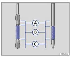
Fig. 152 Oil dipstick with engine oil level marks.
