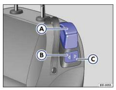
**Fig. 45** On the left side of the driver seat: Controls in the backrest for electrical Easy Entry. On the front passenger side, controls are on the right side of the seat backrest.
