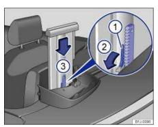
Fig. 174 Deployed rollover protection support behind the rear seat backrest.
