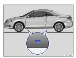
Fig. 185 Lift points for the jack.
