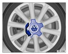
Fig. 181 Twisting the hubcap off.
