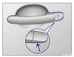
Fig. 164 Door handle on driver door: Concealed lock cylinder.
