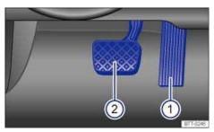
Fig. 127 Pedals: 1 Accelerator pedal, 2 Brake pedal.
