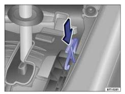
Fig. 176 Releasing the selector lever lock.
