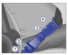
Fig. 63 A safety belt extender properly attached to the factory-installed safety belt.
