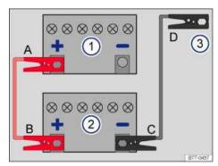
Fig. 197 Diagram for attaching the jumper cables: Dead battery 1 and booster battery 2.
