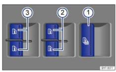
Fig. 30 In the driver door: Switches for the power windows.
