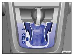
Fig. 175 Removing the selector gate cover.
