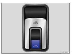
Fig. 35 In the center console: Switch for the power sunroof.
