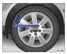
Fig. 184 Changing a wheel: Loosening wheel bolts.
