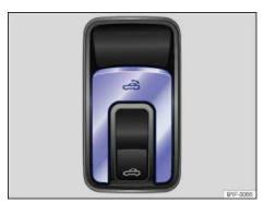
Fig. 172 CSC roof switch in the center console.
