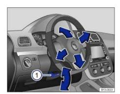
Fig. 48 Manual adjustment for the steering wheel position.
