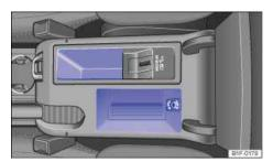
Fig. 114 Inside the front center armrest storage compartment: Jacks for MDI and AUX-IN.
