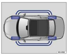
Fig. 103 Tire rotation diagram.
