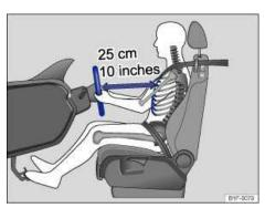
Fig. 40 The driver should never sit closer than 10 inches (25 cm) of the steering wheel.
