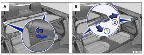
Fig. 33 A. Push tabs (spacers) on wind blocker into slots. B. Align and engage the spring-loaded locking pins.
