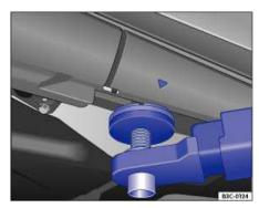
Fig. 162 Rear lift point for workshop hoist or floor jack.
