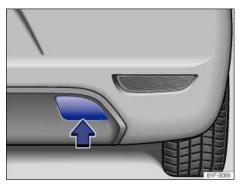
Fig. 200 In right rear bumper: Remove cover.
