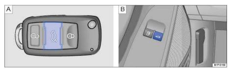
Fig. 27 A: In the remote control vehicle key: Button to unlock and open the luggage compartment lid. B: In the driver door: Switch to unlock and open the luggage compartment lid.
