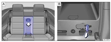
Fig. 167 A: In the seat backrest: Opening the pass-through cover. B: In the luggage compartment: Release ring for luggage compartment lid.
