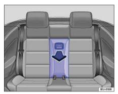
Fig. 99 In the rear backrest: Opening the luggage compartment pass-through cover.
