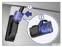
Fig. 196 License plate light: Removing the bulb holder.
