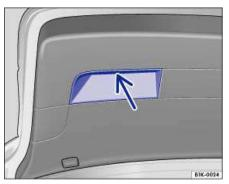
Fig. 29 Opened luggage compartment lid: Recessed grip for closing.
