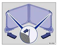
Fig. 34 Unfolding the wind blocker.
