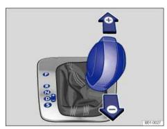
Fig. 130 Selector lever in Tiptronic position.
