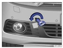
Fig. 199 In right front bumper: Screwing in towing eye.
