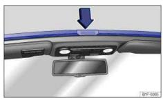
Fig. 36 Wind deflector in the windshield frame.
