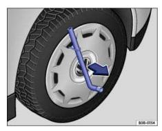
Fig. 183 Pulling the wheel cover off.
