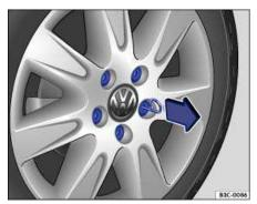
Fig. 182 Pulling cover caps off wheel bolts.
