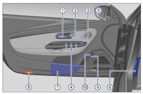
Fig. 4 Overview of controls in the driver door.
