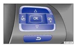
Fig. 15 Right side of the multi-function steering wheel: Controls for menus in the instrument cluster.
