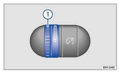
Fig. 84 To the left of the steering wheel: Thumbwheel to adjust instrument panel lighting 1.
