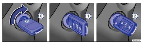
Fig. 124 In the ignition switch: Vehicle key positions.
