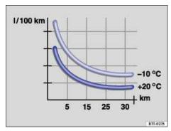
Fig. 136 Fuel consumption in I/100 km at 2 different outside air temperatures.
