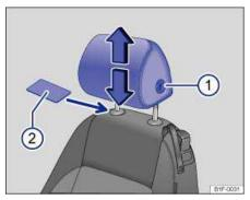
Fig. 47 Removing front head restraints.
