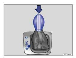
Fig. 129 Automatic transmission selector lever with shift lever release button (arrow).
