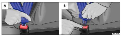
Fig. 59 A: Inserting the safety belt buckle tongue into the belt buckle. B: Releasing the buckle tongue from the belt buckle.
