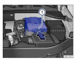
Fig. 157 In the engine compartment: Remove the cover from the vehicle battery.
