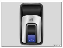
Fig. 171 In the center console: Switch for the power sunroof.
