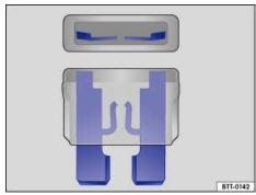
Fig. 190 Illustration of a blown fuse.
