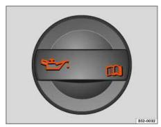
Fig. 153 In the engine compartment: Engine oil filler cap.
