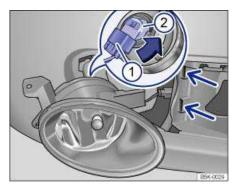
Fig. 194 Replacing a light bulb in the fog light.
