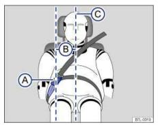
Fig. 64 Positioning of the safety belt extender.
