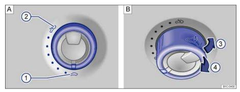
Fig. 33 In the headliner: Rotary switch for the power sunroof. A: Turn the rotary switch to slide the sunroof open or closed. B: Press or pull the switch to tilt open or to close.
