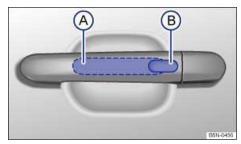
Fig. 28 Keyless Access system: Sensor for unlocking A on the inside of the front door handles. Sensor for locking B on the outside of the door handles.
