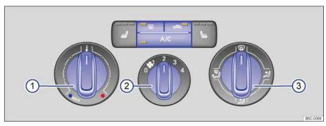
Fig. 132 In the center console: Manual air conditioning controls.
