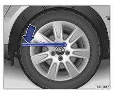
Fig. 165 Changing a wheel: Loosening the wheel bolts.
