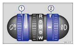
Fig. 74 To the left of the steering wheel: Thumbwheel to adjust instrument panel lighting 1 and headlight range adjustment 2 (if equipped).
