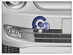
Fig. 175 In the right front bumper: Screwing in the towing eye.
