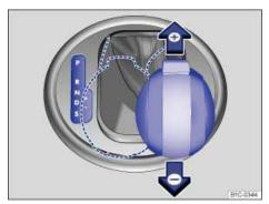
Fig. 120 Selector lever in Tiptronic position.
