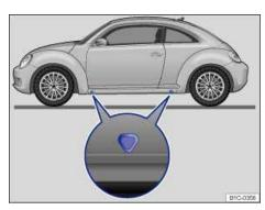
Fig. 166 Lift points for the jack.
