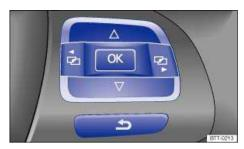
Fig. 17 Right side of the multi-function steering wheel (if equipped): Controls for the menus in the instrument
