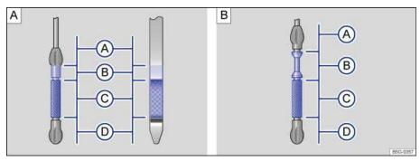
Fig. 142 Engine oil dipstick with oil level marks. A: For vehicles with gasoline engines. B: For vehicles with diesel engines.
