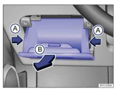
Fig. 169 On the driver side in the instrument panel: Storage compartment in front of the fuse box.
