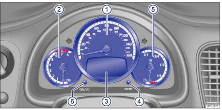
Fig. 11 Instrument cluster in the instrument panel.
