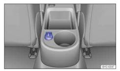
Fig. 110 Rear center console: 12 Volt socket.
