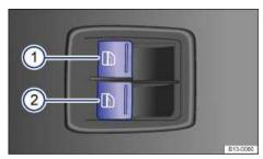
Fig. 32 In the driver door: Switches for the power windows.
