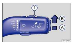
Fig. 80 Windshield wiper lever: Adjusting the rain sensor 1 (if equipped).
