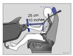
Fig. 35 The driver should never sit closer than 10 inches (25 cm) of the steering wheel.
