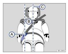
Fig. 56 Positioning of the safety belt extender.
