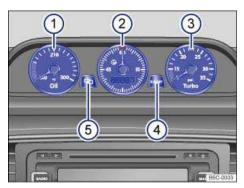
Fig. 12 Above the center console: Engine oil temperature indicator 1, stopwatch 2, and boost pressure indica-
