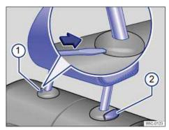
Fig. 40 Removing the rear head restraints.
