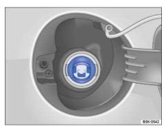
Fig. 137 With open fuel cap: Misfueling guard in the fuel filler neck.
