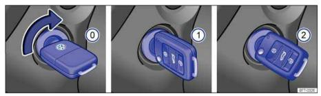
Fig. 111 In the ignition switch: Vehicle key positions.
