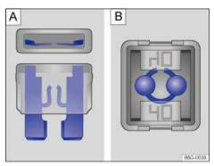
Fig. 171 Blown fuse: A: Blade fuse. B: Cartridge fuse.
