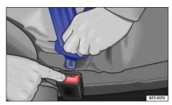
Fig. 52 Releasing the buckle tongue from the belt buckle.
