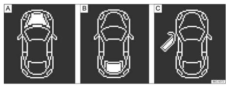
Fig. 14 In the instrument cluster display: A: Open engine hood, B: Open rear hatch, C: Open driver door.
