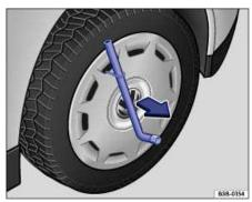
Fig. 163 Pulling the wheel cover off (Version 1).
