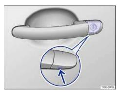
Fig. 153 Door handle on driver door: Concealed lock cylinder.
