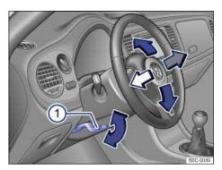
Fig. 41 Manual adjustment for the steering wheel position.
