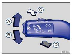
Fig. 70 On the left side of the steering column: Turn signal lever and high beam switch.
