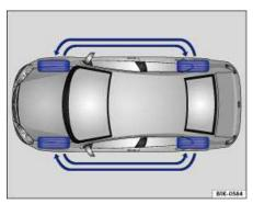
Fig. 92 Tire rotation diagram.
