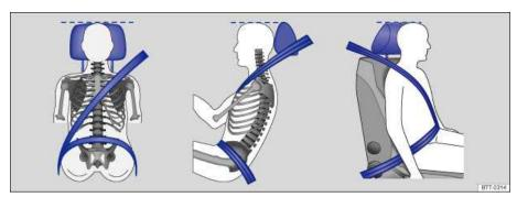
Fig. 53 Proper safety belt positioning and head restraint adjustment.
