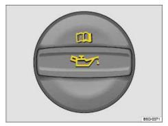
Fig. 143 In the engine compartment: Engine oil filler cap.
