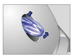
Fig. 30 Opening rear hatch from the outside.
