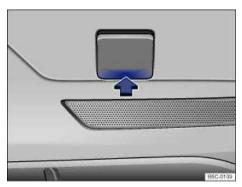
Fig. 178 In the right rear bumper: Removing the cover.
