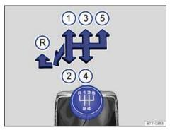
Fig. 117 Gearshift pattern of a 5-speed manual transmission.
