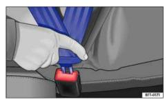
Fig. 51 Inserting the buckle tongue into the belt buckle.
