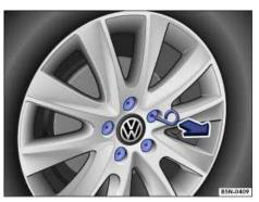
Fig. 162 Pulling cover caps off wheel bolts.
