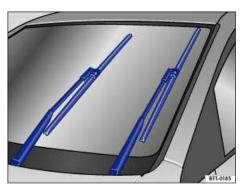
Fig. 79 Windshield wiper in service position.
