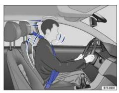
Fig. 50 Belted driver secured by the correctly worn safety belt in the event of a sudden braking maneuver.
