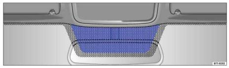
Fig. 77 Heat-reflective windshield with communications window (blue shaded area).
