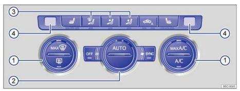
Fig. 133 In the center console: Climatronic controls.
