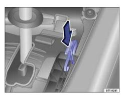
Fig. 157 Releasing the selector lever lock.
