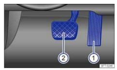
Fig. 116 Pedals in vehicles with automatic transmission: 1 Accelerator pedal, 2 Brake pedal.
