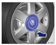
Fig. 160 Pulling the hubcap off.
