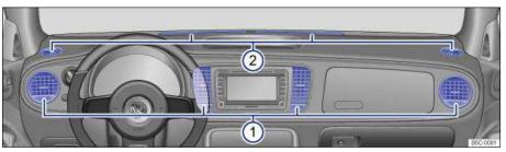
Fig. 134 In the instrument panel: Air vents.
