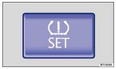
Fig. 97 In the glove compartment: SET button for the Tire Pressure Monitoring System.
