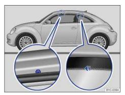
Fig. 91 Attachment points for the base carrier and roof rack.
