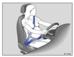
Fig. 54 Proper safety belt positioning for expectant mothers.
