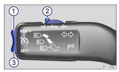
Fig. 126 On the left side of the steering column: Cruise control buttons and switches (if equipped).
