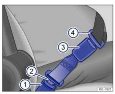
Fig. 55 A safety belt extender properly attached to the factory-installed safety belt.
