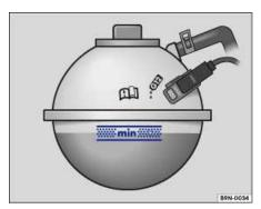
Fig. 144 Coolant expansion tank in the engine compartment.
