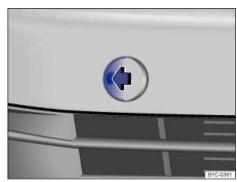
Fig. 174 In the right front bumper: Removing the cover.
