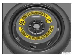
Fig. 95 In the luggage compartment: Compact spare wheel.
