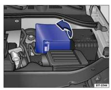
Fig. 146 In the engine compartment: Open the sleeve covering of the vehicle battery.
