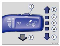
Fig. 78 Operating the front windshield wipers.
