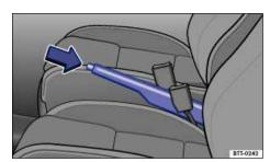
Fig. 122 Between the front seats: Parking brake.
