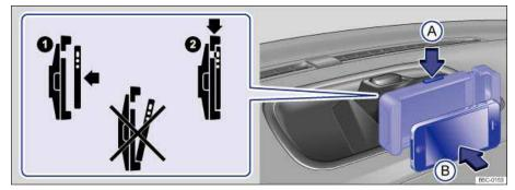
Fig. 149 On the center console: Inserting the iPhone®.
