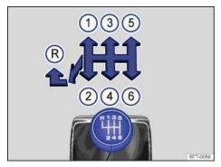
Fig. 118 Gearshift pattern of a 6-speed manual transmission.
