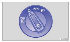
Fig. 72 Headlight switch next to the steering wheel (with fog lights and automatic headlights, if equipped).
