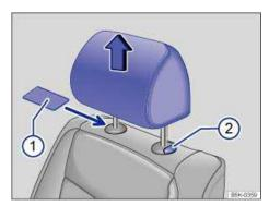
Fig. 39 Removing the front head restraints.
