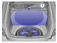
Fig. 158 In the luggage compartment: Floor covering raised and 1 secured.
