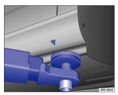
Fig. 150 Front lift point for workshop hoist or floor jack.
