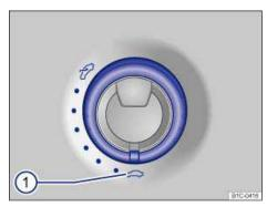
Fig. 34 In the headliner: Sunroof rotary switch.
