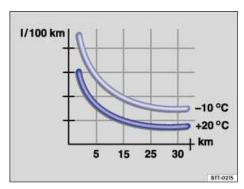
Fig. 125 Fuel consumption in I/100 km at 2 different outside air temperatures.
