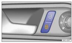
Fig. 26 In the vehicle doors: Power locking button.
