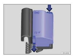
Fig. 170 In the engine compartment: Fuse box cover.
