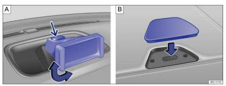
Fig. 148 On the center console. A: Removing the iPhone® holder, B: Installing the cover for the mount.
