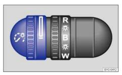
Fig. 73 To the left of the steering wheel: Thumbwheel to adjust instrument panel lighting (vehicles without manual headlight range adjustment).
