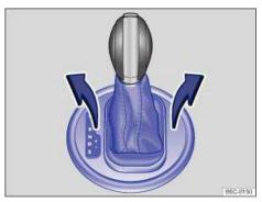
Fig. 156 Removing the selector gate cover.
