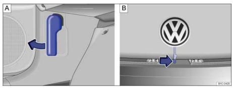
Fig. 140 A: In the footwell on the driver side: Inside engine hood release lever. B: Above the radiator grille:
