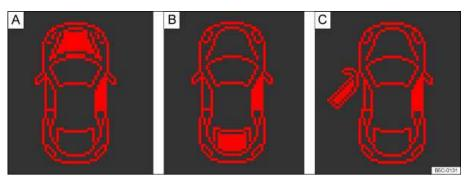
Fig. 13 In the instrument cluster display (examples): A: Open engine hood, B: Open rear hatch, C: Open driver door.
