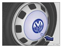
Fig. 164 Pulling the wheel cover off (Version 2).
