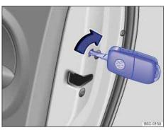
Fig. 154 On the edge of the passenger door: Manually locking the door with the vehicle key.
