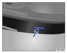
Fig. 20 Vehicle identification number (VIN).
