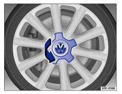
Fig. 161 Twisting the hubcap off.
