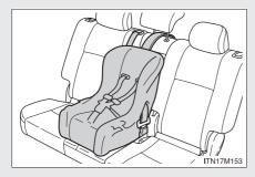
Seat belts equipped with a child restraint locking mechanism (ALR/ELR belts on the second seats)
