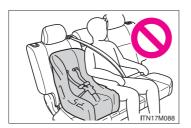
When using the right side lower anchors for the child restraint system, do not sit in the center seat.
