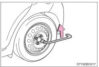
4 Turn the tire jack until the notch of the jack is in contact with the jack point.
