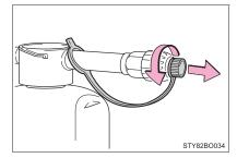
Screw the end of the nozzle clockwise as far as possible.
