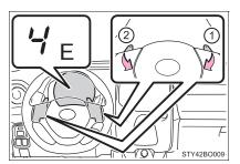
The Gear Shift Indicator is a guide to help the driver achieve improved fuel economy and reduced exhaust emissions within limits of engine performance.
