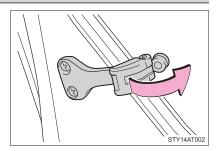
2 Push the latch handle to securely lock the latch as shown in the illustration.
