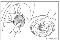
2 Install the spare tire and loosely tighten each wheel bolt by hand by approximately the same amount.
