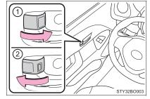
The front doors can be opened by pulling the inside handle even if the lock button is in the lock position.
