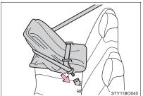
Install a locking clip near the tab of the lap and shoulder belt by inserting the lap and shoulder webbing through the recesses of the locking clip. Buckle the belt again. If the belt has any slack, release the buckle and reinstall the locking clip.
