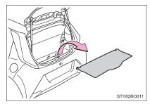
2 Remove the tool tray, then loosen the center fastener.
