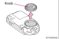
3 Remove the depleted battery.
