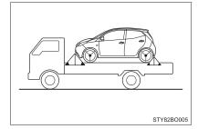
A driver must be in the vehicle to steer and operate the brakes. The vehicle's wheels, drive train, axles, steering and brakes must be in good condition.
