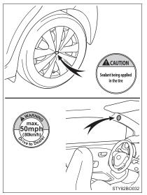
3 Remove the valve cap from the valve of the punctured tire.
