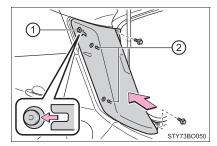
1 Disengage the claws and remove the license plate lights.
