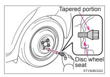
When replacing an aluminum wheel with a steel wheel, tighten the wheel bolts until the tapered portion comes into loose contact with the disc wheel seat.
