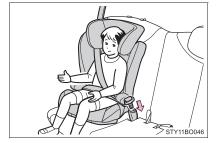
Check that the shoulder belt is correctly positioned over the child's shoulder and that the lap belt is as low as possible. ( $\rightarrow$ P. 30)
