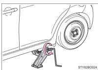
Firmly tighten each wheel bolts two or three times in the order shown in the illustration.
