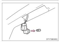
4 Set the new light bulb and turn the bulb base clockwise.
