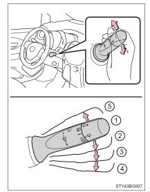
Washer/wiper dual operation Wiper will automatically operate a couple of times after the washer squirts.
