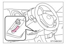
2 Adjust to the ideal position by moving the steering wheel vertically.
