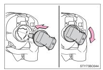
After installing the connector, shake the bulb base gently to check that it is not loose, turn the fog lights on once and visually confirm that no light is leaking through the mounting.
