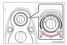
If A/C is not pressed, the system will blow ambient temperature air or heated air.
