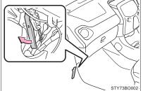
2 Push the auxiliary catch lever to the left and lift the hood.
