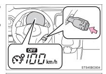
2 Pull the lever towards you to setting the speed limiter.
