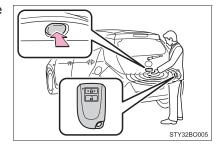
Press the button to lock the back door.
