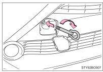
Tighten down the towing eyelet securely using a wheel bolt wrench or hard metal bar.
