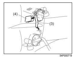
2) Remove the wire of the rear turn signal light (3) from a clamp (4).
