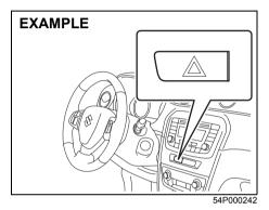
Push in the hazard warning switch to activate the hazard warning lights. All turn signal lights and both turn signal indicators will flash simultaneously. To turn off the lights, push the switch again.
