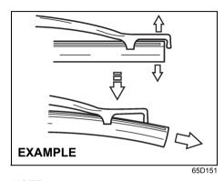
NOTE: Do not flex the wiper blade frame end more than necessary. If you do, it can break off.
