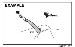
Remove the head restraint before anchoring the top tether strap. After anchoring the top tether strap, check that the top tether strap passes as shown in the illustration. Follow the above procedure in reverse when removing the top tether strap. Please refer to "Seat belts and child restraint systems" section in "BEFORE DRIVING" section for details on securing your child.
