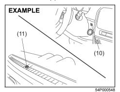
Be careful not to cover the interior temperature sensor (10) located between the steering wheel and the climate control panel, or the solar sensor (11) located at
