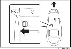
To remove the key from the remote controller, push the button (A) in arrow direction and pull the key out from the remote controller
