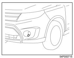
Start the engine. Turn the steering wheel to the opposite side of the fog light to be replaced the bulb easily. Then turn off the engine.
