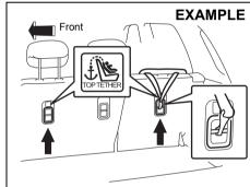
Some child restraint systems require the use of a top tether strap. Top tether anchorage brackets are provided in your vehicle at the locations shown in the illustrations.
