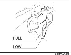
If the coolant level is below "LOW" mark. more coolant should be added. Remove the reservoir tank cap and add coolant until the reservoir tank level reaches "FULL" mark. Never fill the reservoir tank above "FULL" mark.
