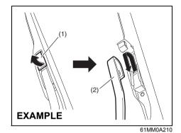
Open the lock (1), slide the wiper frame and remove it from the arm (2) as shown.
