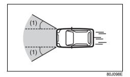
Crash such as above at an angle of about 30 degrees (1) or less from the front Conditions of front air bags may inflate Receiving a strong impact to the lower body of your vehicle, the front air bags will inflate in many cases.
