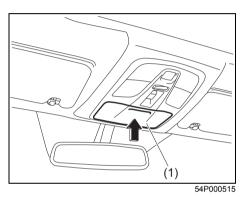
Use this stowage to keep small articles. You can open the lid (1) by pressing the raised portion on it.
