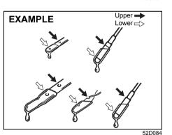
Pull out the oil dipstick, wipe oil off with a clean cloth, insert the dipstick all the way into the engine, and then remove it again. The oil on the stick should be between the upper and lower limits shown on the stick. If the oil level indication is near the lower limit, add enough oil to raise the level to the upper limit.
