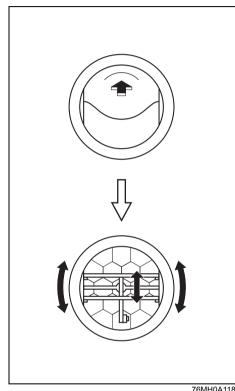
When each outlet is open, air comes out regardless of the air flow selector position.
