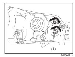
Open the engine hood. To remove the bulb holder of the front turn signal light (1) or the front position light (2) from the light housing, turn the holder counterclockwise and pull it out.
