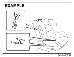
Your vehicle is equipped with the top tether anchorages. Use the top tether strap of the child restraint according to the instructions provided by the child restraint system manufacturer.
