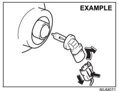
5) Disconnect the coupler by pushing the lock release. Turn the bulb holder counterclockwise and remove it.
