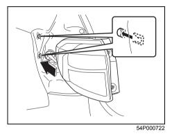
NOTE: When reinstalling the light housing, check that the clips are properly attached.
