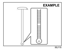
Check that there is washer fluid in the tank by looking at the washer fluid level gauge which is attached to the cap of the washer fluid tank. If the fluid level is near empty, refill it. Use a good quality windshield washer fluid, diluted with water as necessary.
