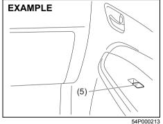
The passenger's door has a switch (5) to operate the passenger's window.
