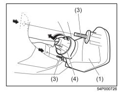
2) Remove the light housing (1) by pushing the bolts (3). To remove the bulb holder of the rear fog light (4), turn the holder counterclockwise and pull it out.
