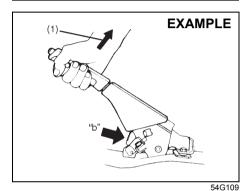
Ratchet tooth specification "b": 4th – 9th Lever pull force (1): 200 N (20 kg, 45 lbs)
