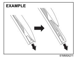
3) Pull the locked end of the wiper blade firmly to unlock the blade and slide the blade out as shown.
