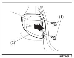
1) Remove the bolts (1) and pull the light housing (2) straight.
