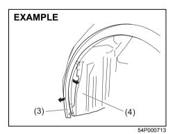
4) Remove the end of the front fender splash guard (3), and open the end of the cover (4) inside the fender.
