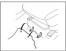
To prevent the driver's side floor mat from sliding forward and possibly interfering with the operation of the pedals, genuine SUZUKI floor mats are recommended. Whenever you put the driver's side floor mat back in the vehicle after it has been removed, hook the floor mat grommets to the fasteners and position the floor mat properly in the footwell.
