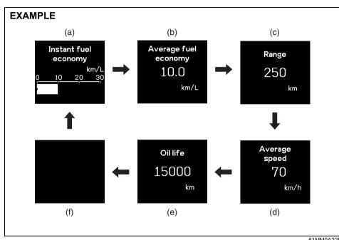
To switch the display indication, push the indicator selector knob (2) quickly.
