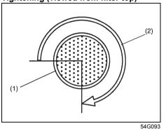
(1) Oil filter (2) 3/4 turn (For diesel engine model)
