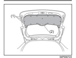
1) Open the tailgate. Remove 15 clips (1), and then pull out the trim (2).
