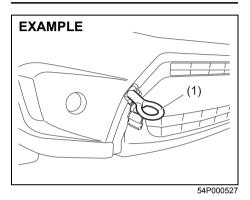
The towing hook (1) is provided on the front of the vehicle for use in emergency situations only.
