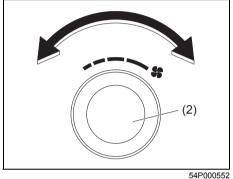
The blower speed selector (2) is used to turn on the blower and to select blower speed.
