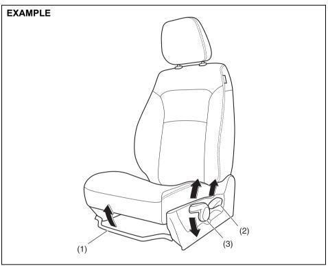
**Seat position adjustment lever (1)** Pull the lever up and slide the seat.
