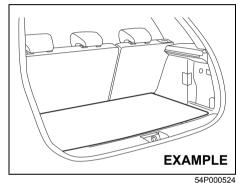
Your vehicle is equipped with the luggage compartment board in the luggage compartment. You can place luggage or other cargos on the board or under the board. You can also place tall luggage by removing the board from the luggage compartment.
