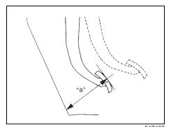
Minimum distance between brake pedal and floor carpet "a": 59 mm (2.3 in.)
