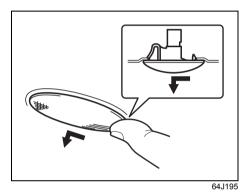
Since the bulb is built-in type, replace it as the light assembly. Remove the light assembly by sliding the light housing leftward with your finger.
