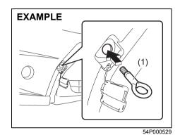
3) Install the towing hook (1) by hand.
