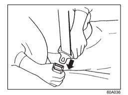
To fasten the seat belt, sit up straight and far back into the seat, pull the latch plate attached to the seat belt across your body and press it straight into the buckle until you hear a click.
