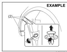
3) Remove the clips (2) by prying them off with a flat-bladed screwdriver as shown in the illustration.
