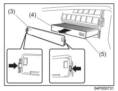
3) Remove the cover (3) and pull out the air conditioner filter (4).
