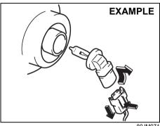
Open the engine hood. Disconnect the coupler by pushing the lock release. Turn the bulb holder counterclockwise and remove it.
