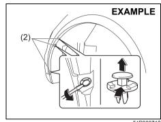
3) Remove the clips (2) by prying them off with a flat-bladed screwdriver as shown in the illustration.
