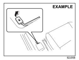
A fuel filler cap is located on the left rear side of the vehicle. The fuel filler door can be unlocked by pulling up the opener lever located on the outboard side of the driver's seat and locked by simply closing the door.
