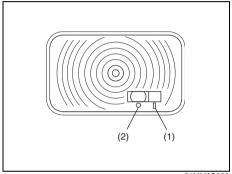
When you open the tailgate with the luggage compartment light switch in ON position (1), the light comes on and remains on as long as you keep the tailgate open. When the luggage compartment light switch is in OFF position (2), the light remains off regardless of whether the tailgate is open or close.
