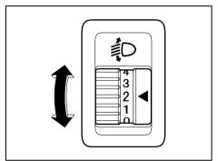
Level the headlight beam according to the load condition of your vehicle by turning this switch. The chart below shows the appropriate switch position for different vehicle load conditions.
