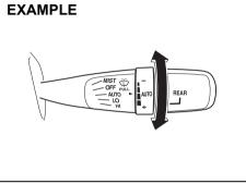
If the control lever has on "AUTO" position, you can change the system's sensitivity to rain/snow by turning the knob of the control lever increased sensitivity or backward for decreased sensitivity.
