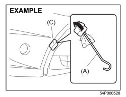
Remove the cover (C) by using a jack handle (A) covered with a soft cloth as shown in the illustration.
