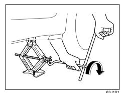
6) Position the jack at an angle as shown in the illustration and raise the jack by turning the jack handle clockwise until the jack-head groove fits around the jacking bar beneath the vehicle body.  Continue to raise the jack slowly and smoothly until the tire clears the ground. Do not raise the vehicle more than necessary.
