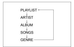
3) Press "TUNE/FLD PUSH SOUND" knob (2) to select the desired mode.
