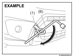
4) To tighten the towing hook (1), turn it clockwise by using a wheel brace (B) until the hook (1) is securely installed.
