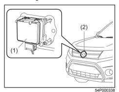
If dirt is detected on the radar sensor cover, the radar brake support system will stop functioning and the radar brake support system warning light (3) will come on, and "RADAR BRAKE SUPPORT: NOT ACTIVE BY SENSOR." message (4) will appear.
