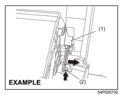
2) To remove the glove box, remove the damper (if equipped) (1) by shifting it to the right side while pressing the tab (2).
