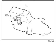
(1) Loosen (2) Tighten 5) Tighten the filter as specified below from the point of contact with the mounting surface (or to the specified torque) using an oil filter wrench.
