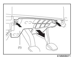
NOTE: To approach the fuses, remove the screws and remove the cover (1).
