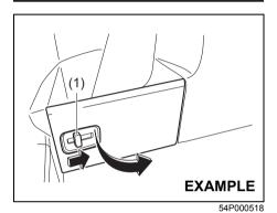
To open the lid, slide the lever (1) and pull the lid.
