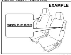
Side air bags are located in the part of the front seatbacks closest to the doors. The "SRS AIRBAG" labels are attached to the seatbacks to identify the location of the side air bags.
