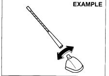
The radio antenna on the roof is removable. To remove the antenna, turn it counterclockwise. To reinstall the antenna, turn it clockwise firmly by hand.
