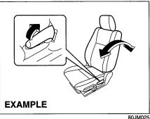
To adjust the seatback angle of front seats, pull up the lever on the outboard side of the seat, move the seatback to the desired position, and release the lever to lock the seatback in place.
