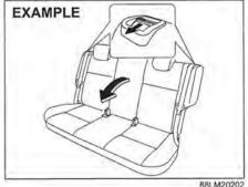
For the split seat, pull the release lever on the top of each split seat, and fold the seatbacks forward.
