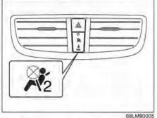
The front passenger's front air bag must be deactivated if a child restraint system is to be installed on the front passenger's seat.
