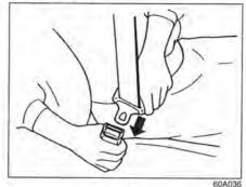
To fasten the seat belt, sit up straight and well back in the seat, pull the latch plate attached to the seat belt across your body and press it straight into the buckle until you hear a "click".
