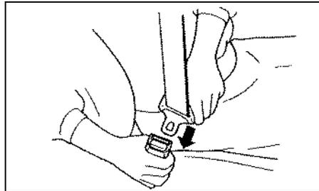
To fasten the seat belt, sit up straight and well back in the seat, pull the latch plate attached to the seat belt across your body and press it straight into the buckle until you hear a "click".
