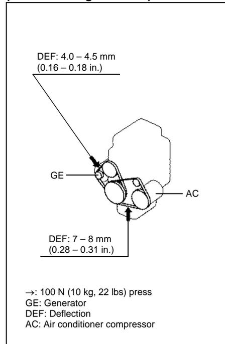
**(For Diesel Engine Model)**
