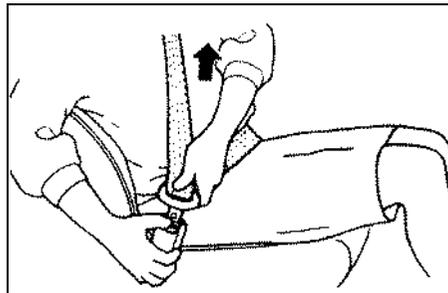
To unfasten the seat belt, push the button on the buckle and retract the belt slowly while attaching a hand to the belt or/and the latch plate.
