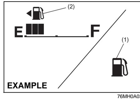
When the ignition switch is in the “ON” position, this gauge gives an approximate indication of the amount of fuel in the fuel tank. “F” stands for full and “E” stands for empty.
