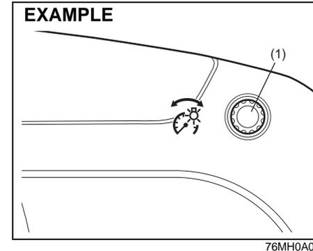
When the ignition switch is turned to the “ON” position, the pointer lights come on.
