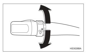
When the headlight switch is in the "  $\verb"=oos"$  " or "  $\verb"\equiv"$  " position, you can adjust brightness of the instrument panel illumination for better visibility.
