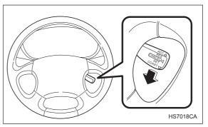
2. Push the control lever downward in the "SET, COAST" direction once. Now the desired speed is set and the vehicle will keep running at that speed without depressing the accelerator pedal.
