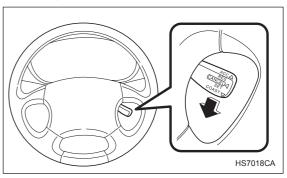
2. When the speed decreases to the desired speed, press the control lever downward in the "SET, COAST" direction once. Now the desired speed is set and the vehicle will keep running at that speed without depressing the accerelator pedal.
