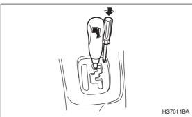
4. Insert the screwdriver into the hole.
