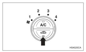
ON (Recirculation): Interior air recirculates inside the passenger compartment. Push the air inlet selection button to the ON position for fast cooling with the air conditioner or when driving on a dusty road. The indicator light comes on when the "Recirculation" mode is selected.
