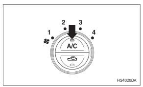
If the windshield starts to fog when the climate control system is operated in the AUTO mode, push the air conditioner switch "A/C" to defog and dehumidify. When this switch is pushed, the air conditioner compressor turns on and the indicator light comes on. After eliminating the fogging from the windshield, set the system back to the AUTO mode by pushing the "AUTO" switch.
