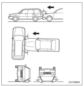
The SRS frontal airbag is basically not designed to deploy if the vehicle is struck from side or from behind, or if it rolls onto its side or roof, or if it is involved in a low-speed frontal collision.
