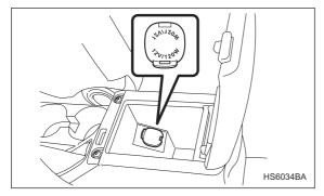
Accessory power outlets are provided in the center console and in the cargo area.
