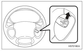
To resume the cruise control after it has been temporarily canceled and with vehicle speed of about 20 mph (32 km/h) or more, push the control lever upward in the "ACCEL, RESUME" direction to return to the original cruising speed automatically.
