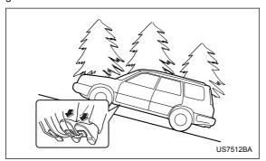
On an uphill grade, when the clutch pedal is depressed while the brake pedal is also depressed, braking power is maintained temporarily by the Hill holder when the brake pedal is released. The driver is therefore able to start the vehicle the same way as on a level grade, just using the clutch and accelerator pedal.
