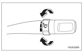
When the wiper switch is in the " \( \overline{\nabla} \) " position, turn the dial to adjust the operating interval of the wiper.
