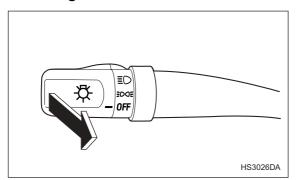
To flash the headlights, pull the lever toward you and then release it. The high beam will stay on for as long as you hold the lever. The headlight flasher works even though the lighting switch is in the "OFF" position.
