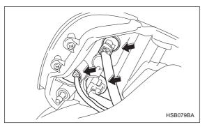
5. Pull the headlight assembly slightly toward you, then hold down the lock release tabs on the connectors for the front turn signal light, parking light, and front side marker light and pull out the headlight assembly completely.
