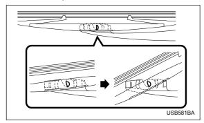
2. Turn the wiper blade assembly counterclockwise.
