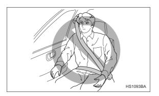
Do not rest your arm on either front door or its internal trim. It could be injured in the event of SRS side airbag deployment.
