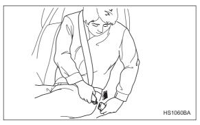
5. Insert the center seatbelt tongue plate in the center seatbelt buckle marked "CENTER" on the left-hand side until it clicks.
