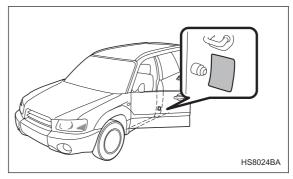
Check the tire pressures when the tires are cold. Use
