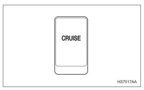
Cruise control enables you to maintain a constant vehicle speed without holding your foot on the accelerator pedal and it is operative when the vehicle speed is 25 mph (40 km/h) or more. Make sure the main switch is turned "OFF" when the cruise control is not in use to avoid unintentionally setting the cruise control.
