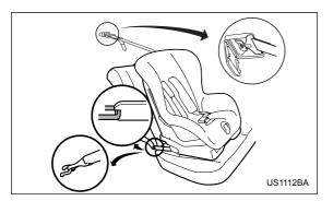
Some types of child restraint systems can be installed on the rear seat of your vehicle without use of the seat-belts. Such child restraint systems are secured to the designated anchorages provided on the vehicle body. The lower and tether anchorages are sometimes referred to as the LATCH system (Lower Anchors and Tethers for CHildren).
