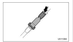
To connect the extender to the seatbelt, insert the tongue plate into the seatbelt buckle so that the "PRESS" signs on the buckle-release buttons of the extender and the seatbelt are both facing outward as shown in the diagram. You will hear a click when the tongue plate locks into the buckle.
