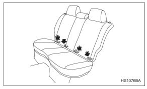
The lower anchorages (bars) are used for installing a child restraint system only on the rear seat window-side seating positions. For each window-side seating position, two lower anchorages are provided.
