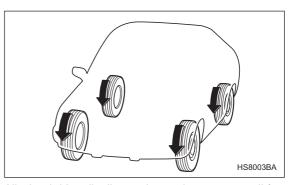
All wheel drive distributes the engine power to all four wheels. AWD vehicles provide better traction when driving on slippery, wet or snow-covered roads and when moving out of mud, dirt and sand. By shifting power between the front and rear wheels, SUBARU AWD can also provide added traction during acceleration and added engine braking force during deceleration.
