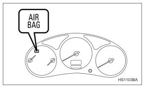
A diagnostic system continually monitors the readiness of the SRS airbag system while the vehicle is being driven. The SRS airbag system warning light "AIR-BAG" will show normal system operation by lighting for about 6 seconds when the ignition key is turned to the "ON" position.
