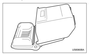
Particles of ash and tobacco will accumulate around the hinges of the ashtray's inner lid. Clean them off using a toothbrush or other narrow-ended implement. ■ Climate control panel, audio panel, instrument panel, console panel, switches, combination meter, and other plastic surfaces
