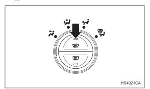
To defrost or dehumidify the windshield and side windows, push the defroster switch " \( \overline{\pm} \) ". When the " \( \overline{\pm} \) " switch is pushed, regardless whether the air conditioner is operating or not, outside air is drawn into the passenger compartment, the air conditioner compressor turns on, air flow is directed towards the windshield and side windows, and the indicator light on the switch comes on.
