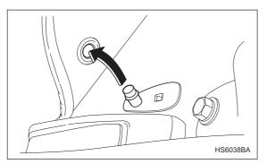
A retaining pin is located on the driver's side of the vehicle next to the fuel filler door release.
