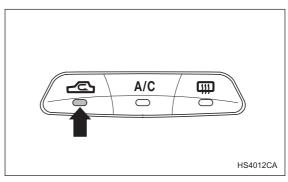
ON position (Recirculation): Interior air is recirculated inside the vehicle. Push the air inlet selection button to the ON position. The indicator light will come on. Place the air inlet selection button to the ON position for fast cooling with the air conditioner or when driving on a dusty road.
