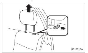
1. Remove the headrest at the seating position where the child restraint system has been installed with the lower anchorages or seatbelt; lift up the headrest while pressing the release button. Store the headrest in the cargo area. Avoid placing the headrest in the passenger compartment to prevent it from being thrown around in the passenger compartment in a sudden stop or a sharp turn.
