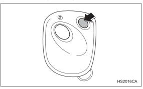
1. Press "UNLOCK/DISARM" button to disarm the security system. (If your vehicle is equipped with the optional security system.)
