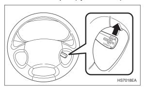
Push the control lever upward in the "ACCEL, RE-SUME" direction and hold it until the vehicle reaches the desired speed. Then, release the control lever. The vehicle speed at that moment will be memorized and treated as the new set speed.
