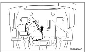
4. Open the access cover by removing the six clips and turning the access cover counterclockwise. The drain plug will be exposed.
