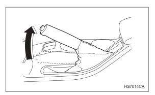
Check the parking brake stroke according to the maintenance schedule in the "Warranty and Maintenance Booklet". When the parking brake is properly adjusted, braking power is fully applied by pulling the lever up seven to eight notches gently but firmly (about 44 lb, 196 N, 20 kg). If the parking brake lever stroke is not within the specified range, have the brake system checked and adjusted at your SUBARU dealer.
