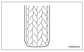
Roadholding is good, and steering is responsive. Rolling resistance is low, so fuel consumption is also lower.
