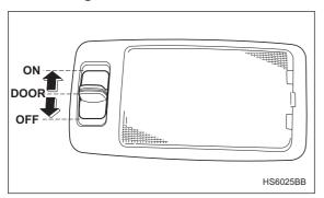
The dome light switch has three positions:
