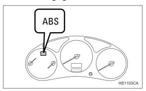
The ABS warning light comes on when the ignition switch is turned to the "ON" position and goes out after about two seconds.
