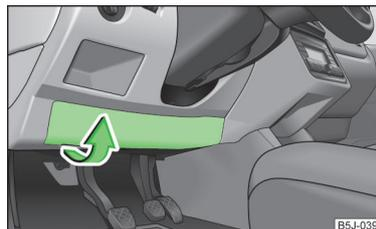
Fig. 150 Underside of the dash panel: Distribution board cover.
