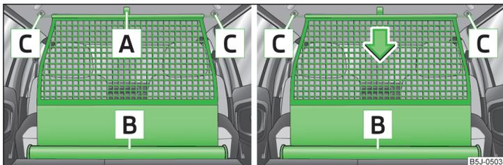
Fig. 71 Extending/retracting the net partition
