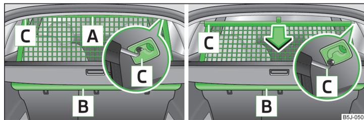
Fig. 70 Extending/retracting the net partition
