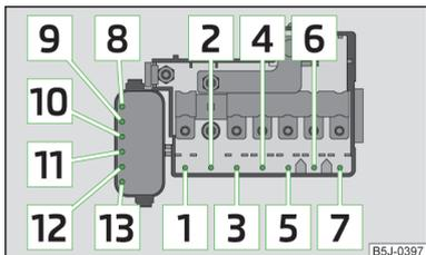
Fig. 153 Schematic representation of fuse box in engine compartment
