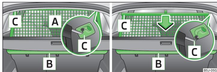
Fig. 70 Extending/retracting the net partition
