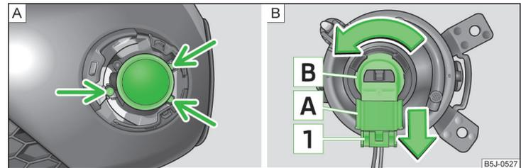
Fig. 160 Front bumper: Fog lights/fog lights: Replacing the light bulb
