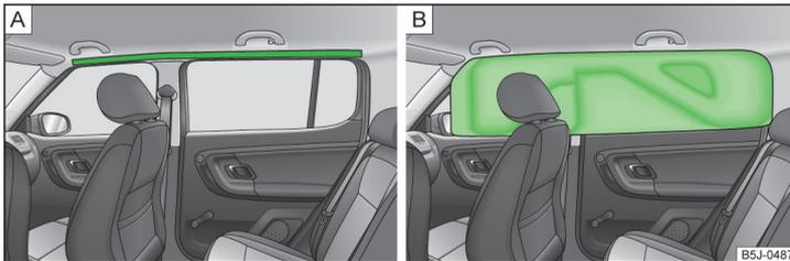
Fig. 11 Location of the head airbag/gas-filled head airbag
