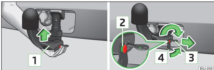
Fig. 120 Insert the ball head/lock the lock, and put the lock cover on
