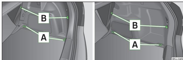
Fig. 61 Boot: Lashing eyes and fastening elements
