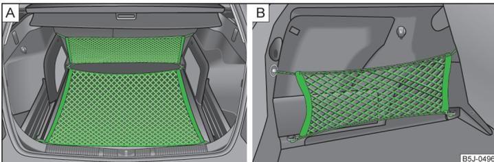
Fig. 63 Fixing net: double horizontal pocket, floor fixing net/double vertical pockets
