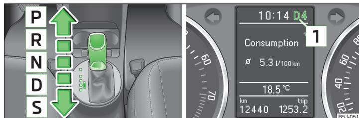
Fig. 105 Selector lever /MAXI DOT display: Selector lever positions
