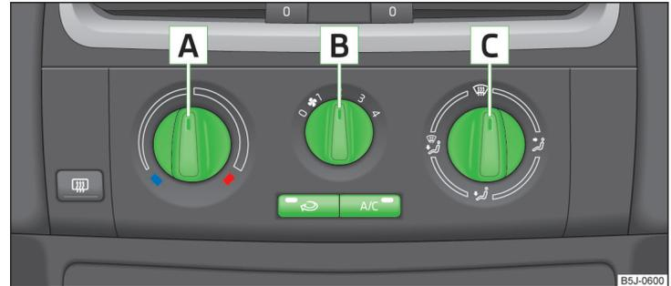
Fig. 96 The air conditioning system: Control elements
