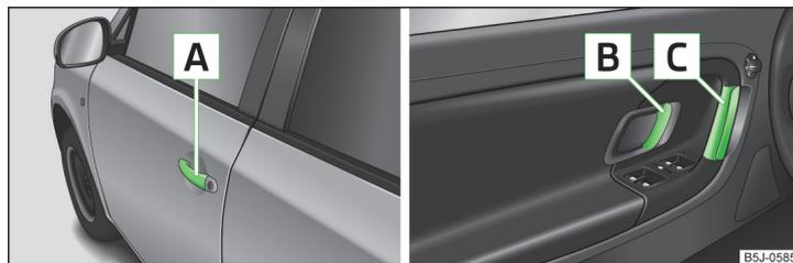
Fig. 28 Door handle/door opening lever
