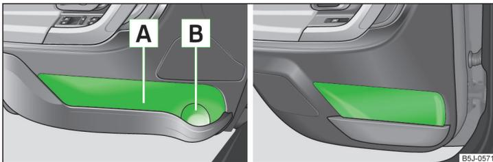
Fig. 91 Storage compartment: in the front door/in the rear door
