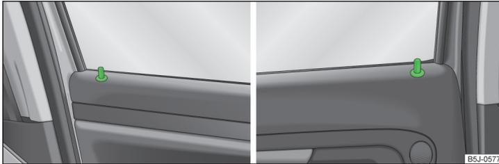
Fig. 29 Securing knob in the front door/rear door
