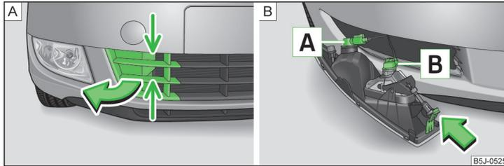
Fig. 158 Front bumper: Protective grille/removing the fog light
