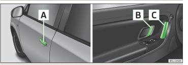
Fig. 28 Door handle/door opening lever
