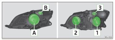
Fig. 154 Bulb arrangement: Halogen headlights/halogen projector head-lights
