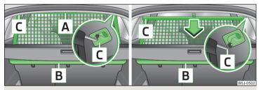
Fig. 70 Extending/retracting the net partition
