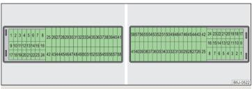
Fig. 151 Schematic representation of the fuse box for vehicles with lefthand steering/right-hand steering
