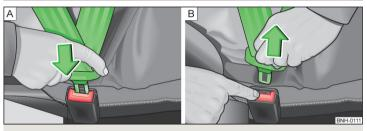
Fig. 5 Fastening/unfastening the seat belt
