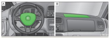
Fig. 8 Driver airbag in the steering wheel/front passenger airbag in the dashboard
