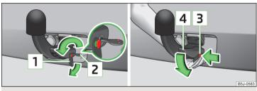
Fig. 122 Unlock the operating lever of the ball head/removing the ball head
