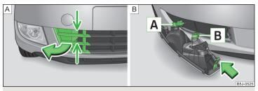
Fig. 158 Front bumper: Protective grille/removing the fog light
