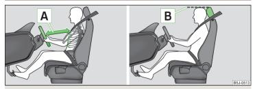
Fig. 1 The correct distance of the driver to the steering wheel/correctly adjusted head restraint
