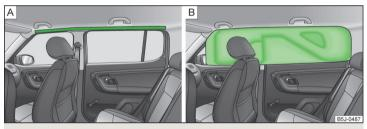
Fig. 11 Location of the head airbag/gas-filled head airbag
