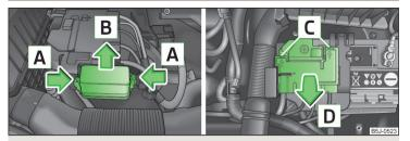
Fig. 152 Vehicle battery: Distribution board cover.
