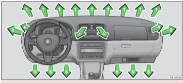
Fig. 94 Air outlet vents
