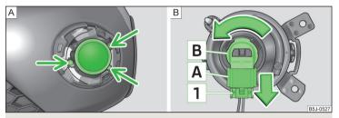
Fig. 160 Front bumper: Fog lights/fog lights: Replacing the light bulb
