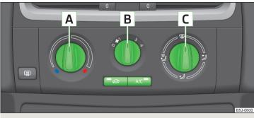
Fig. 96 The air conditioning system: Control elements
