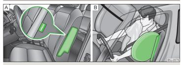
$\mathsf{Fig. 10}$   $\,$  Location of the side airbag in the driver's seat/gas-filled side airbag  $\,$
