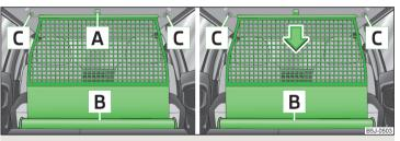
Fig. 71 Extending/retracting the net partition
