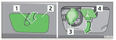
Fig. 117 Remove cover cap: on the rear bumper / for the receiving shaft
