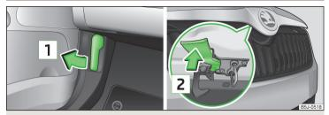
Fig. 124 Bonnet release lever/release lever
