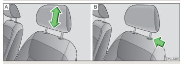
Fig. 59 Head restraint: adjusting/removing
