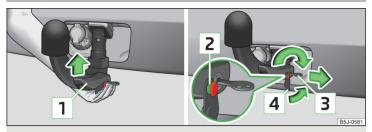
Fig. 120 Insert the ball head/lock the lock, and put the lock cover on
