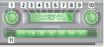
Fig. 97 Climatronic: Control elements
