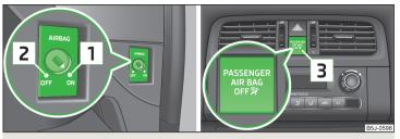
Fig. 12 Key-operated switch for the front passenger airbag/warning light for front seat passenger airbag deactivation
