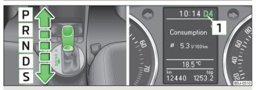
Fig. 105 Selector lever /MAXI DOT display: Selector lever positions
