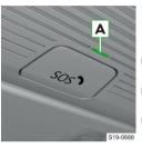
The system status is displayed after the ignition is switched on, by the illumination of warning lamp A.
