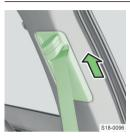
Move the seat belt height adjuster upwards to increase the height.
