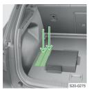
A storage compartment for the Cargo elements is located under the variable loading floor.
