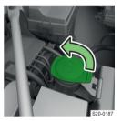
Sealing cap of the tank - variant 1
