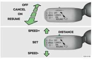
Activate ACC (condition for the subsequent activation of ON the limiter)
