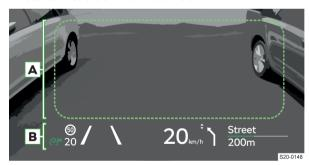
A Display area with information that is projected directly onto objects in the driver's field of vision
