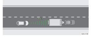
ACC detects a narrow or staggered vehicle only when it is in the area covered by the radar.
