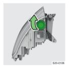
> Remove the protective cap from the headlight.
