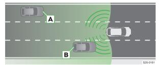
Your vehicle is being overtaken by vehicle  $\boxed{\mathbf{A}}$ . The faster vehicle  $\boxed{\mathbf{A}}$  approaches, the sooner the warning is given by the indicator light.
