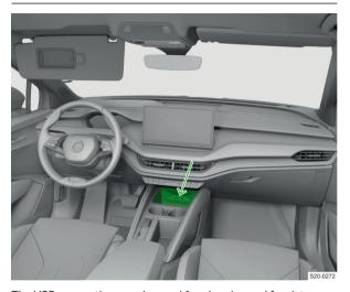
The USB connections can be used for charging and for data transfer.
