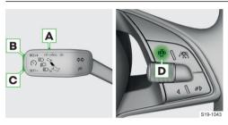
ON Activate cruise control (condition for the subsequent activation of the limiter).
