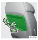
Press the safety button and fold the table up to the desired position.
