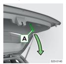
> Grasp the fixture A and pull the lid down.
