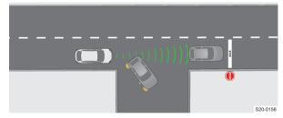
If a vehicle in front turns and there is a stationary vehicle in front of this vehicle, the ACC must not respond to the stationary vehicle.
