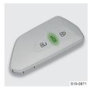
> Press the \infty button to open, close or stop the movement of the tailgate.
