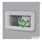
> Pull on the switch. The tow bar swings out. The indicator light → inside the switch illuminates.
