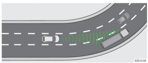
When cornering, a vehicle in the next lane may enter the detected area. Your vehicle will be controlled according to this vehicle.
