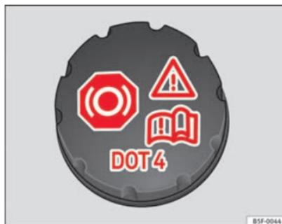
Fig. 157 Engine compartment: brake fluid reservoir, lid
