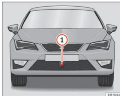
Fig. 131 On the front bumper: radar sensor. ►
