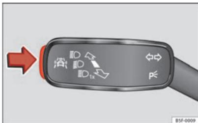
Fig. 44 On the turn signal and main beam headlight lever: button for the driving assistance systems
