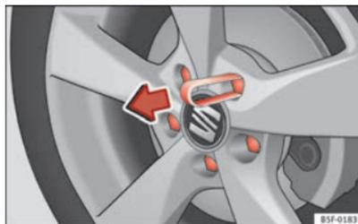
Fig. 166 Wheel: wheel bolts with caps
