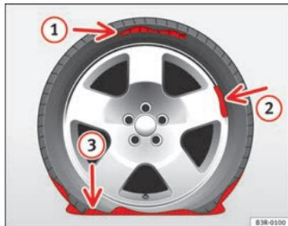
Fig. 163 Tyre: irreparable damage
