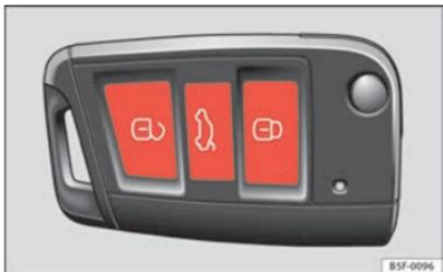
Fig. 50 Remote control key: Buttons
