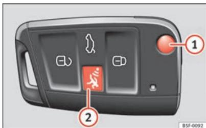
Fig. 46 Vehicle key with alarm button
