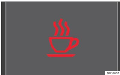
**Fig. 145** On the instrument panel display: Tiredness detection symbol
