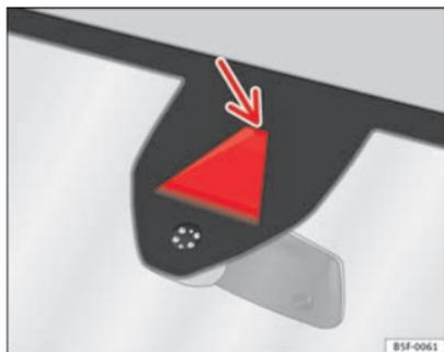
**Fig. 143** In the wind-screen: Field of vision of the Lane Assist system camera
