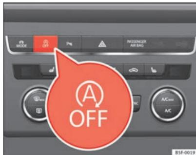
Fig. 120 Centre console: Start-Stop system button
