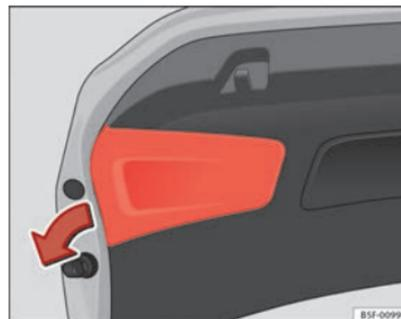
Fig. 195 Remove the cover from the rear lid
