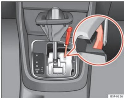
**Fig. 125 Selector lever: manual release from position P**
