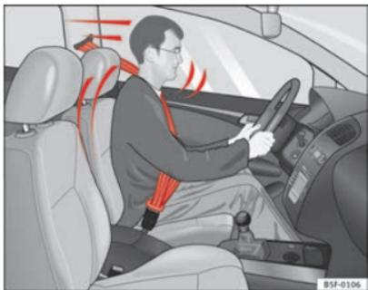
**Fig. 12** A driver wearing the seat belt properly is secured by the belt in sharp braking
