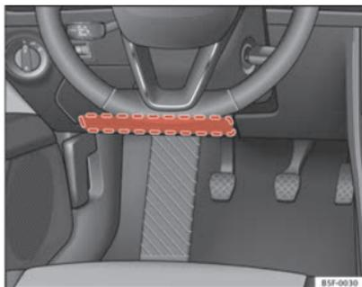
Fig. 23 On the driver side: location of the knee airbag
