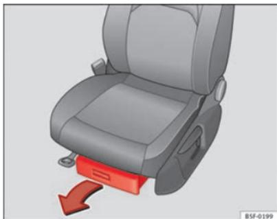
Fig. 83 Storage compartment under the front seats
