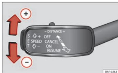
Fig. 133 On the left of the steering column: Third lever for using the adaptive cruise control.
