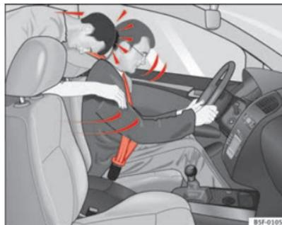
**Fig. 11** The unbelted passenger in the rear seat is thrown forward violently, hitting the driver wearing a seat belt
