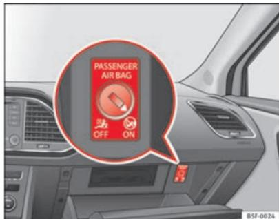
Fig. 28 Front passenger front airbag switch
