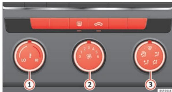
Fig. 115 In the centre console: heating system and fresh air controls
