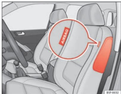
**Fig. 25 Side airbag in driver seat**
