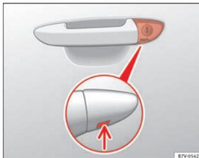
Fig. 55 Driver door lever: Hidden lock cylinder ▶
