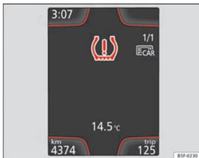
Fig. 146 Instrument panel: warning of loss of tyre pressure
