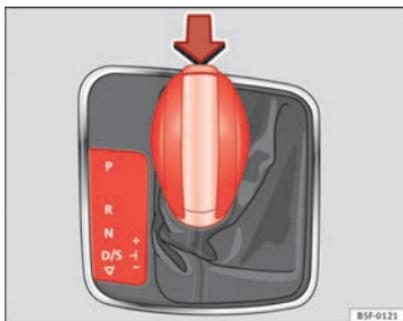
**Fig. 122 Selector lever lock**
