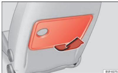
Fig. 84 Left-hand front seat: folding table
