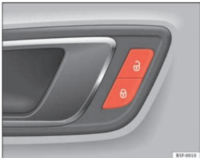
Fig. 52 Driver door: central locking switch
