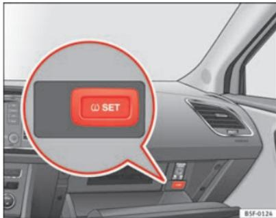
Fig. 147 Glove compartment: tyre control switch
