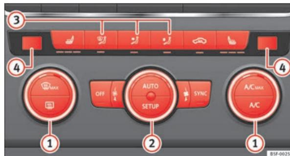
**Fig. 113** In the centre console: Climatronic controls
