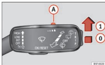
Fig. 72 Windscreen wiper lever: adjusting the rain sensor (A)
