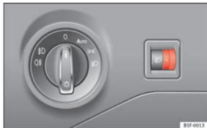
Fig. 67 Next to the steering wheel: Headlight range control
