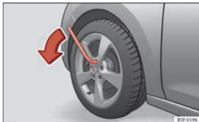
Fig. 168 Wheel: loosen the wheel bolts
