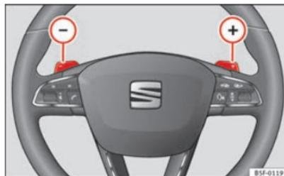
**Fig. 124** Steering wheel: automatic gearbox levers
