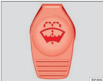
Fig. 158 Engine compartment: Windscreen washer reservoir top
