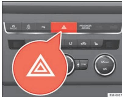
Fig. 66 Dash panel: switch for hazard warning lights
