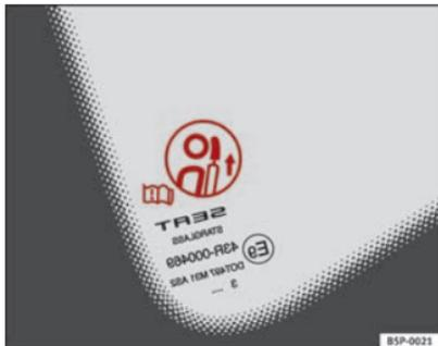
Fig. 6 Head restraint position warning label
