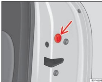
**Fig. 56 Locking the door manually**
