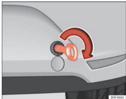
Fig. 176 Right side of the rear bumper: towline anchorage screwed in
