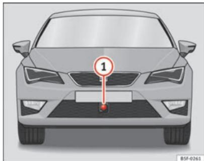
**Fig. 139** On the front bumper: radar sensor.
