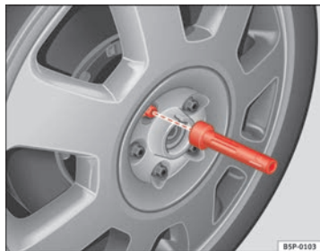
Fig. 131 Changing the wheel: Hexagonal socket in screwdriver handle to turn the wheel bolts
