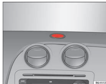
Fig. 76 Mounting bracket for navigator on dash panel.
