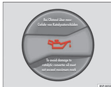
Fig. 119 In the engine compartment: Engine oil filler cap
