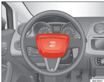
Fig. 16 Driver airbag located in steering wheel
