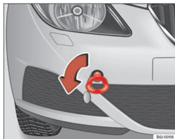
Fig. 155 Fitting the towing eye to front rear of the vehicle
