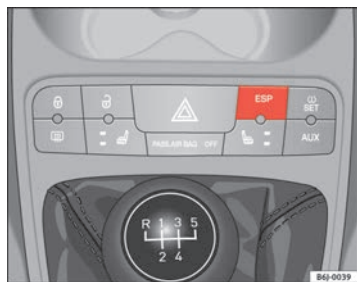
Fig. 95 Detailed view of the centre console: ESP button.
