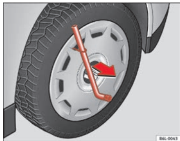
Fig. 127 Remove the complete hub cap
