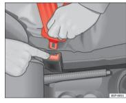
Fig. 15 Remove latch plate from buckle
