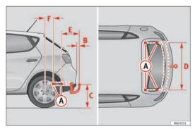
Fig. 118 Attachment points for towing bracket
