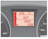
Fig. 106 Automatic gearbox: Instrument panel display
