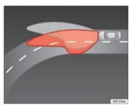
Fig. 57 Cornering lighting using adaptive headlights
