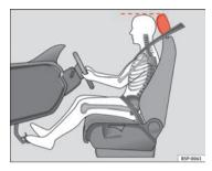
Fig. 2 Correct head restraint position for driver
