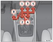
Fig. 103 Centre Console: gear shift pattern of a 5speed manual gearbox
