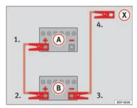
Fig. 168 Diagram of connections for vehicles without Start-Stop sys-
