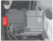
Fig. 142 Fuses in engine compartment
