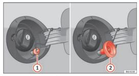
Fig. 120 Fuel tank open with LPG filler neck and adapter.
