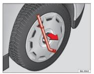
Fig. 136 Remove the complete hub cap
