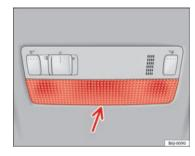
Fig. 165 Front reading light
