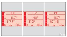
Fig. 102 Display on the instrument panel during Start-Stop function operation.
