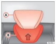
Fig. 5 Adjusting the rear head restraints
