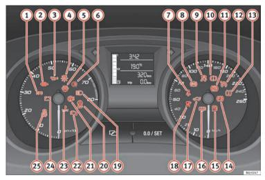
Fig. 38 Instrument panel warning and control lamps.
