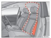
Fig. 20 Side airbag in driver seat
