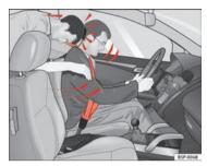
Fig. 9 The unbelted passenger in the rear seat is thrown forward violently, hitting the driver wearing a seat belt
