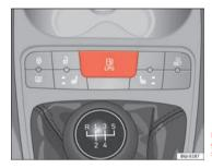
Fig. 100 Centre console: gas system control switch.
