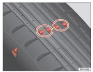
Fig. 134 Tyre tread wear indicators
