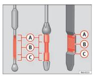
Fig. 125 Engine oil dipstick
