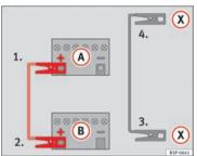
Fig. 169 Diagram of connections for vehicles with Start-Stop system
