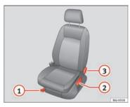
Fig. 72 Front left seat controls
