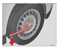
Fig. 137 Changing a wheel: loosen the wheel bolts
