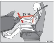
Fig. 1 The correct distance between driver and steering wheel
