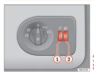
Fig. 56 Dash panel: regulation for instrument and switch lighting and headlight range control
