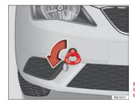
Fig. 170 Fitting the towline anchorage to front of the vehicle
