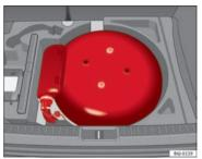
Fig. 121 LPG tank in spare wheel well
