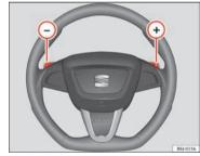
Fig. 109 Steering wheel with paddle levers for automatic gearbox
