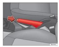
Fig. 111 Handbrake between the front seats
