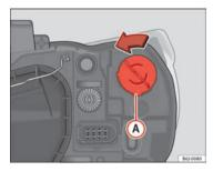
Fig. 144 Single turn signal lamp
