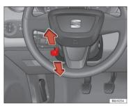
Fig. 97 Steering column height adjustment
