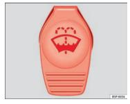
Fig. 128 In the engine compartment: Cap of windscreen washer fluid reservoir.
