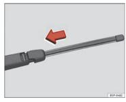
Fig. 132 Fitting the rear window wiper blade
