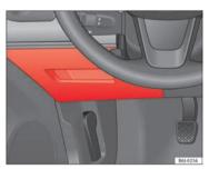
Fig. 141 Fuses in the dash panel
