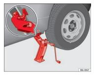
Fig. 139 Fitting the jack
