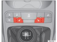
Fig. 73 Front seats heating switch
