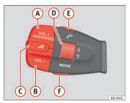
Fig. 42 Audio + Telephone Control
