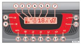
Fig. 96 Climatronic controls on the dash panel
