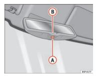
Fig. 67 Automatic antidazzle interior rear vision mirror.
