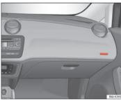
Fig. 17 Front passenger airbag located in dash panel
