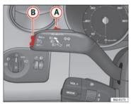
Fig. 115 Turn signal and main beam headlight lever: switch and rocker switch for the cruise con-
