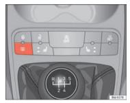
Fig. 58 Centre console: heated rear window
