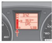
Fig. 31 Instrument panel: gas gauge.
