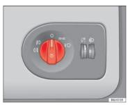
Fig. 54 Detailed view of the dash panel: lights, fog lights and rear fog light switch
