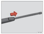
Fig. 131 Removing the rear window wiper blade
