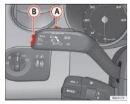
Fig. 116 Turn signal and main beam headlight lever: switch and rocker switch for the cruise con-
