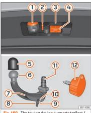
Fig. 169 The towing device supports trailers / tow hook / key
