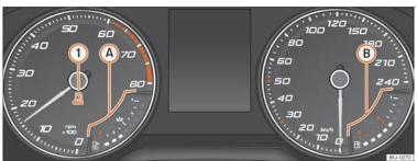
**Fig. 70** Analogue instrument panel: natural gas gauge
