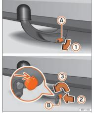
Fig. 175 Removing the tow hook
