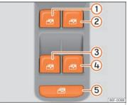
Fig. 95 Detail of the driver's door: window controls.
