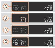
Fig. 149 Instrument panel display: GRA status indications.
