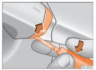
Fig. 90 Driver door handle: lever the cover off
