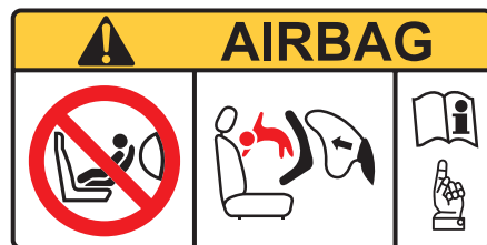
Warning label - Front passenger airbag
