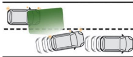
While the direction indicators are on and for a few seconds after switching them off, the system considers that any change of trajectory is intentional and no correction is triggered during this period.
