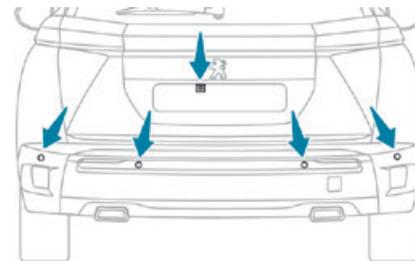
As soon as reverse gear is engaged with the engine running, this system displays views of your vehicle's close surroundings on the touch screen using a camera located at the rear of the vehicle.
