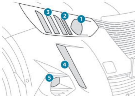
1. Dipped beam headlamps / Main beam headlamps
