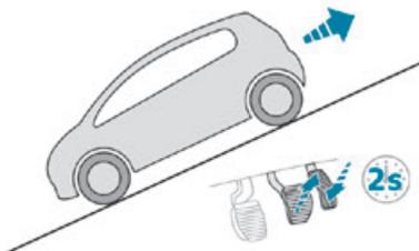
**On a descending slope, with the vehicle stationary and reverse gear engaged, the vehicle is held for a short time when you release the brake pedal.**
