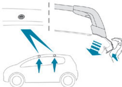
You must only attach the transverse bars to the four fixing points located on the roof frame. These points are concealed by the vehicle doors when the doors are closed. The roof bar fixings have a stud which must be inserted into the opening of each fixing point.
