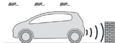
The system signals the presence of obstacles within the sensors' detection zone.
