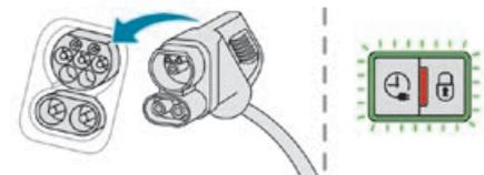
► Depending on version, remove the protective cover from the lower section.
