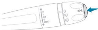
▶ Pressing the button located on the end of the **wiper control stalk** displays the following tabs in turn:
