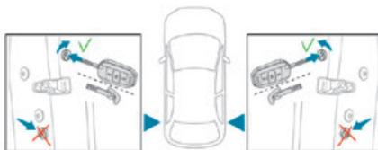
**!** Do not confuse the child lock control, which is red, with the back-up locking control, which is black.
