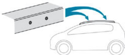
The transverse bars must be fixed at the engraved markings on the longitudinal bars.
