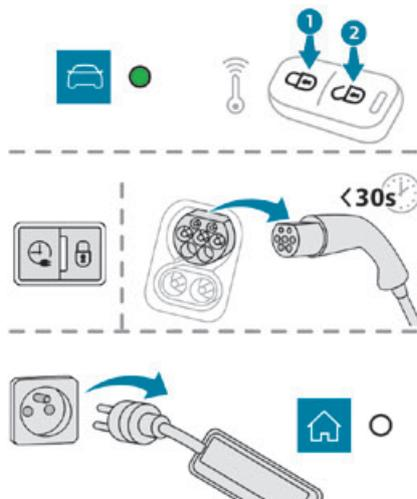
When charging is complete, the green **CHARGE** indicator lamp on the control unit comes on fixed.
