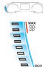
The gauge shows the consumption of electric power for thermal comfort functions.
