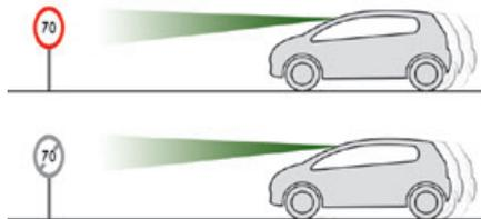
This system displays the maximum authorised speed in the instrument panel, according to the speed limits in the country in which you are driving, using:
