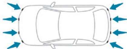
Using sensors located in the bumper, this system signals the proximity of obstacles (e.g. pedestrian, vehicle, tree, barrier) present in their field of detection.
