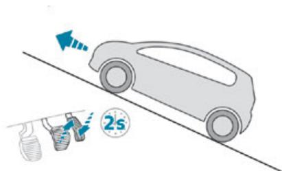
**On an ascending slope, with the vehicle stationary, the vehicle is held for a short time when you release the brake pedal:**
