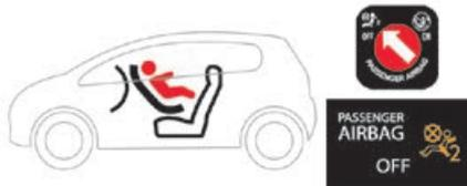
**!** The front passenger airbag must be deactivated before installing a rearward facing child seat. Otherwise, **the child risks being seriously injured or killed if the airbag deploys.**
