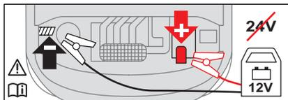
**!** If this label is present, use only a 12 V charger to avoid causing irreversible damage to the electrical components related to the Stop & Start system.
