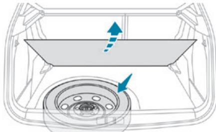
The spare wheel is stored under the boot carpet. To access the spare wheel, first refer to the **Tool kit** section.
