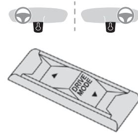
► Press the **DRIVE MODE** button to choose one of the three driving modes; the different modes are displayed in the instrument panel.
