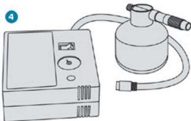
4. 12 V compressor with a cartridge of sealant and a speed limit sticker
