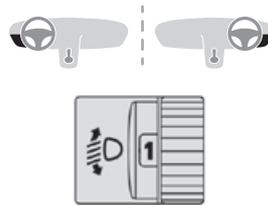
To avoid dazzling other road users, the height of these headlamp beams should be adjusted according to the load in the vehicle.
