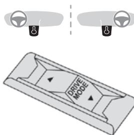
Pressing the control displays the modes on the instrument panel.
