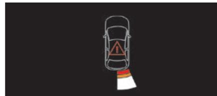
This supplements the audible signal by displaying bars on the screen that represent the distance between the obstacle and the vehicle (white: more distant, orange: close, red: very close).
