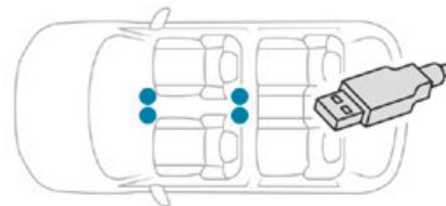
They allow the connection of a portable device in order to recharge it.
