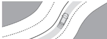
Using a camera located at the top of the windscreen, the system identifies lane markings and steers the vehicle inside this lane to keep it in the lateral position chosen by the driver. This function is primarily suitable for driving on motorways and main roads.
