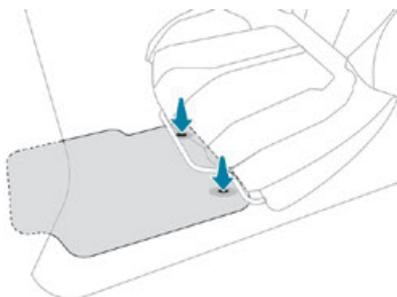
When fitting the mat for the first time, on the driver's side use only the fasteners supplied in the enclosed sachet. The other mats are simply laid over the carpet.
