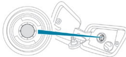
When a petrol filler nozzle is inserted into the fuel filler neck of a Diesel vehicle, it comes into contact with the flap. The system remains closed and prevents filling.
