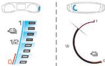
The traction battery charge status and remaining range are displayed continuously when the vehicle is started.
