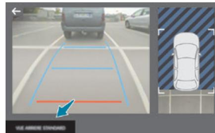
To activate the camera, located on the tailgate, engage reverse and keep the speed of the vehicle below 6 mph (10 km/h).
