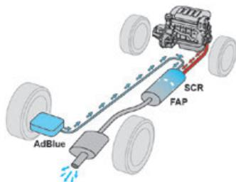
To respect the environment and ensure compliance with the Euro 6 standard, without adversely affecting the performance or fuel consumption of its Diesel engines, PEUGEOT has taken the decision to equip its vehicles with a system that associates SCR (Selective Catalytic Reduction) with a Diesel Particle Filter (DPF) for the treatment of exhaust gases.
