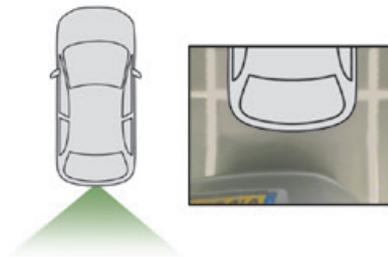
The camera records the vehicle's surroundings during the manoeuvre in order to create a view from above the rear of the vehicle in its near surroundings, allowing the vehicle to be manoeuvred around nearby obstacles. This view is available with AUTO mode or in the view selection menu.
