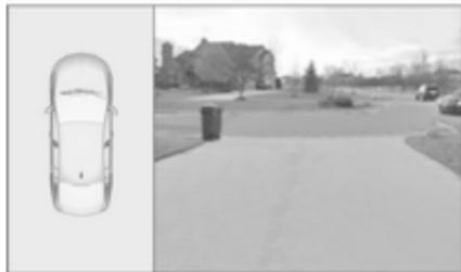
The screen in the Info Display is divided into two parts: on the left there is a view from above the vehicle, and
