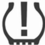
A detected low tyre pressure condition is indicated by the control indicator (⚠) ⇨ 108.
