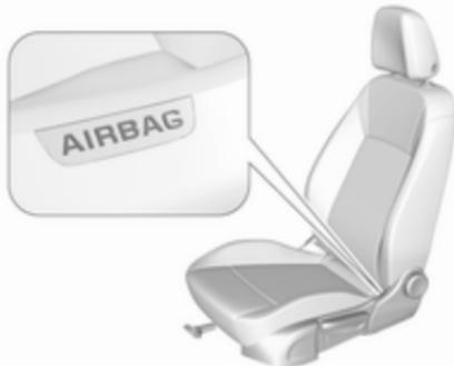
The side airbag system consists of an airbag in each front seat backrest and in the rear outer seat backrests. This can be identified by the word **AIRBAG**.
