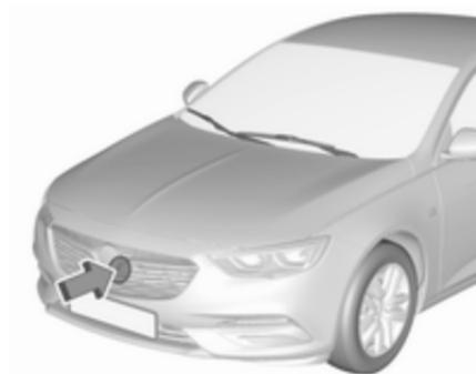
The radar unit is mounted behind the radiator grille or below the brand emblem.
