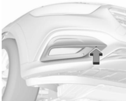
Undo the screw with a torx screwdriver.
