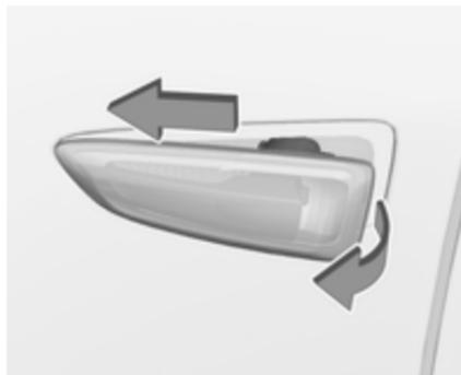
1. Slide the lamp housing forward and remove it at the back.
