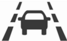
When the control indicator
