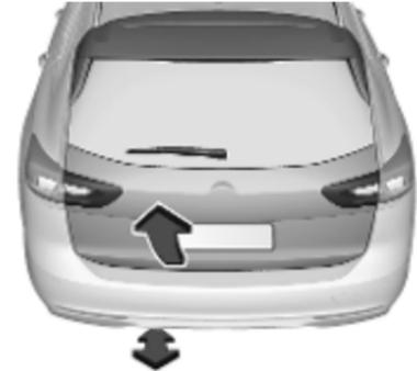
To open or close the tailgate, move the foot in the center area below the rear bumper back and forth quickly. Do not hold the foot under the bumper. The electronic key must be outside the vehicle, within a range of approx. 1 m of the tailgate. When foot
