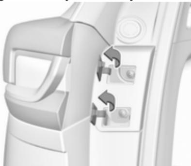
1. Open the covers with screwdriver. Unscrew and remove both screws.
