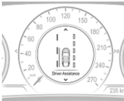
If the system is active but one or both lanes are not detected, they appear as a line of hollow dashes, as shown on the right side of the vehicle in the graphic above.
