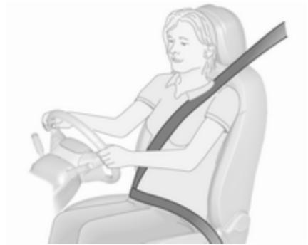
The seat belts are locked during heavy acceleration or deceleration of the vehicle, holding the occupants in the seat position. Thereby the risk of injury is considerably reduced.
