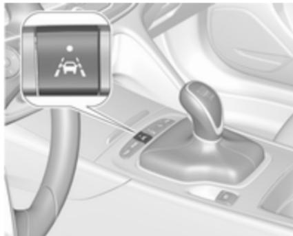
The lane keep assist is activated by pressing
