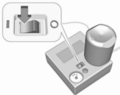
8. Set the rocker switch on the compressor to I. The tyre is filled with sealant.
