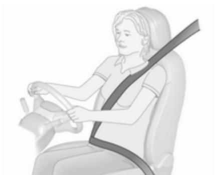
Pull out the seat belt and fasten in belt buckle. The seat belt must not be twisted and must fit close against the body. The backrest must not be tilted back too far (maximum approx. 25°).
