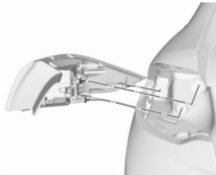
3. Carefully withdraw light assembly from recess and remove. Take care that the cable is not being pulled off.
