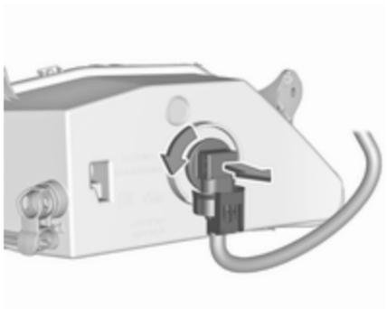
4. Turn the bulb socket anticlockwise and remove it from the light assembly.
