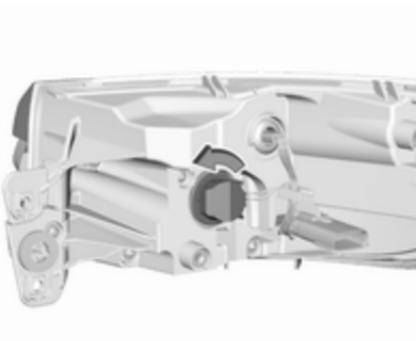
3. Turn the turn light bulb socket anticlockwise and remove it from the light assembly.
