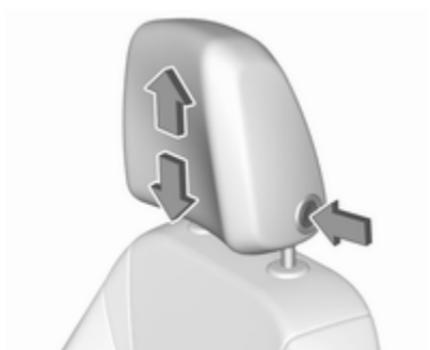
Press release button, adjust height, engage.
