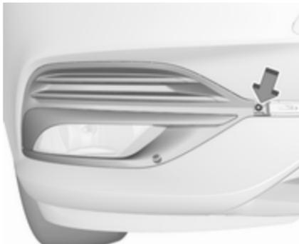
Undo screw with the torx screwdriver and remove the faceplate.
