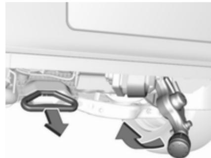
Pull the grip located left to the number plate under the rear bumper fascia at an angle of approx. 45° to the ground.
