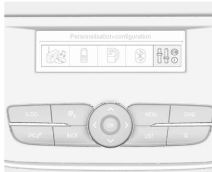
Press **MENU** to open the menu page. Use four-way button to operate the display:
