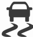
ESC and traction control system are operational after each engine start as soon as the control indicator
