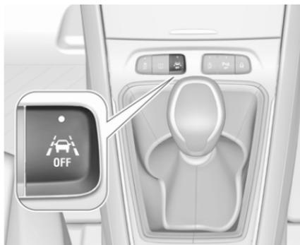
If the system is activated, the LED in the button
