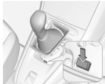
3. Push down the button and move the selector lever out of **P**. Have the cause of the power supply interruption remedied by a workshop.
