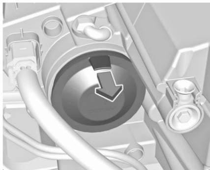
1. Remove the protective cover by pulling.
