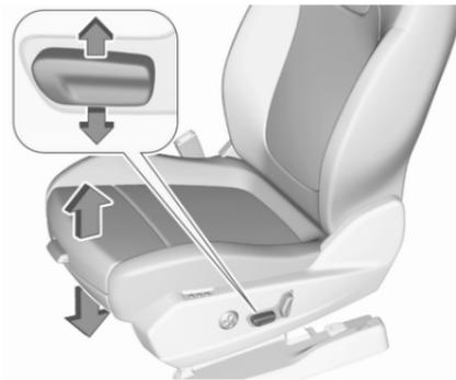
Move switch upwards / downwards.
