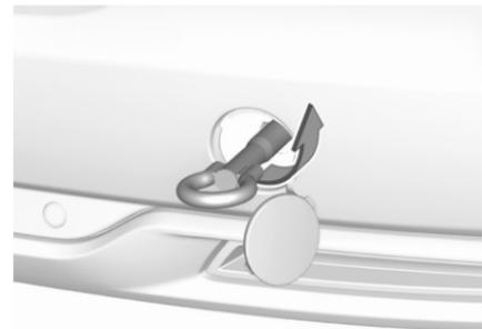
Screw in the towing eye as far as it will go until it stops in a horizontal position.
