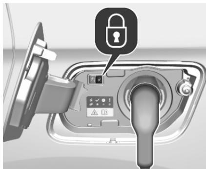
Once charging, the vehicle plug will be locked to the charge port and cannot be disconnected while charging is active.
