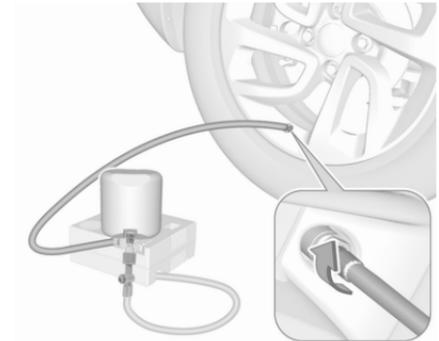
7. Screw the filler hose to the tyre valve.
