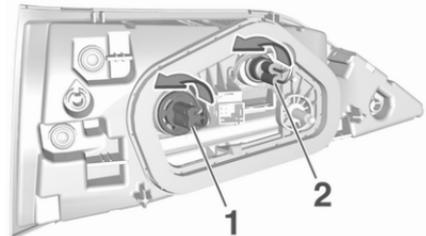
6. Turn the bulb socket anticlockwise and remove it from the light assembly.
