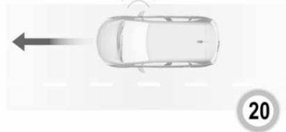
When a free slot is detected, a visual feedback on the Info Display and a first acoustic signal are given. Drive slowly forwards. When the second acoustic signal is given, stop the vehicle, select reverse gear, release the steering wheel and start moving slowly. A visual feedback is given on the Info Display.
