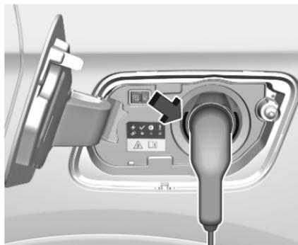
The start of charging is indicated by the green flashing of the status indicator at the charge port and at the control box of the charge cord.
