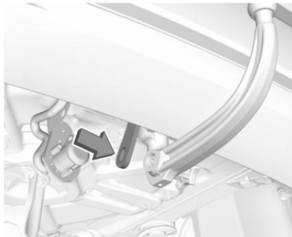
Attach breakaway stopping cable to eye.
