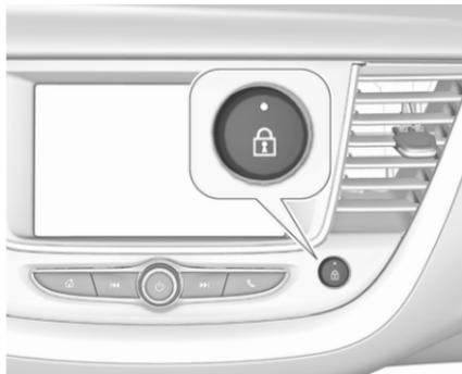
This function can be activated or deactivated at any time. With the ignition on, press
