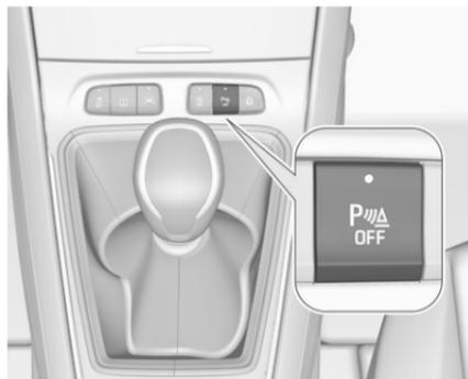
The system is ready to operate when the LED in the parking assist button
