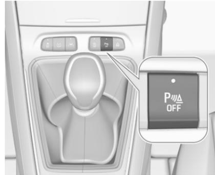
The system is switched off when reverse gear is disengaged. Press
