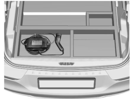
3. Open the tailgate. Lift the rear floor storage cover and remove the charge cord.
