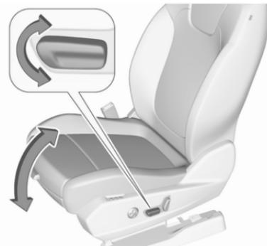
Move front of switch upwards / downwards.
