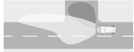
Activated at a speed of up to 25 mph when turning off. The light consists of particular LEDs which illuminate the direction of travel. These LEDs are triggered depending on the steering angle or the activation of the turn lights.
