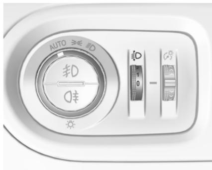
To adapt headlight range to the vehicle load to prevent dazzling, turn thumb wheel
