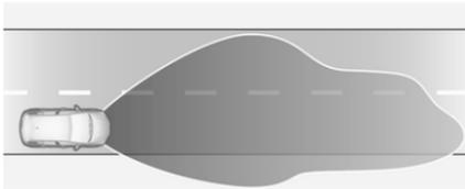
Activated automatically at a speed above 71 mph. Illumination is adapted to the higher speed driven on motorways. If there is no oncoming traffic, the visibility on the side of the vehicle is increased. The visibility range raises from 70 m to 140 m
