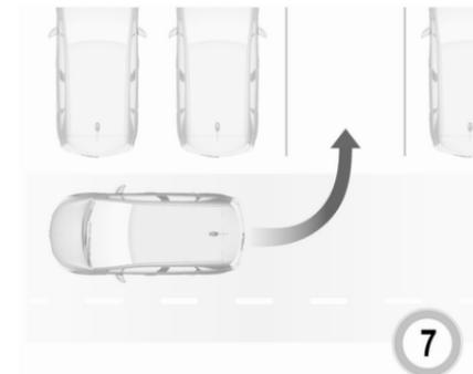
Move forwards and backwards as instructed by observing the warnings of the parking assist and paying attention to the acoustic signals until the end of manoeuvre is indicated. When finished,
