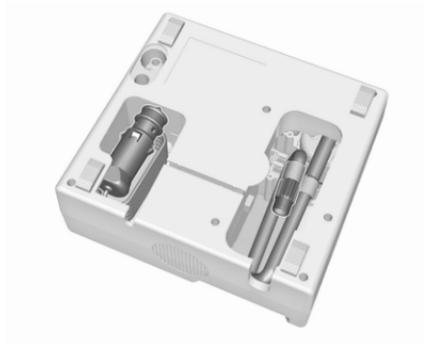
3. Remove the electrical connection cable and air hose from the storage compartments on the underside of the compressor.
