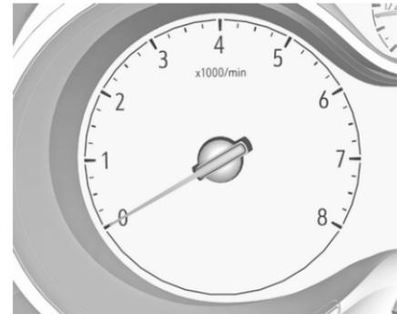
Displays the engine speed.
