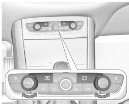
Set the preselected temperatures separately for the driver and the front passenger to the desired value using the left and right rotary ring. The rotary ring on the passenger side
