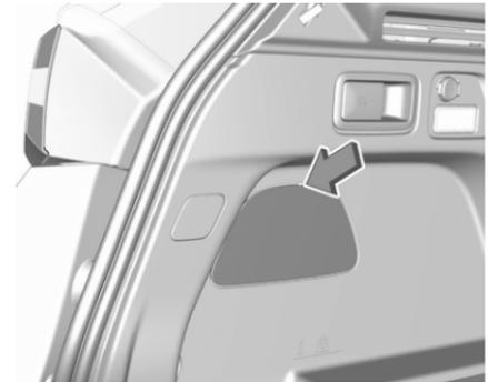
1. Open the tailgate then unclip the access cover on the relevant side.
