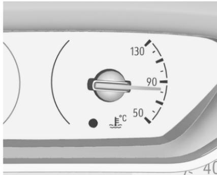
Displays the coolant temperature.
