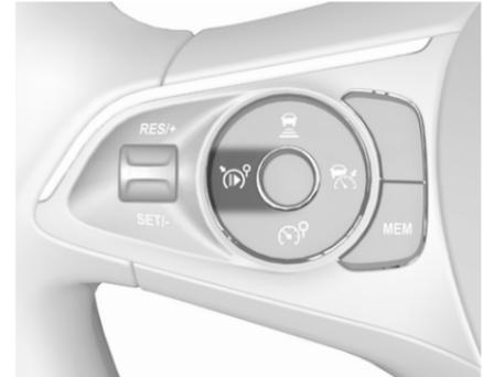
Press **RES+**, the adaptive cruise control is in pause mode and a message is displayed. The vehicle is driven without adaptive cruise control.
