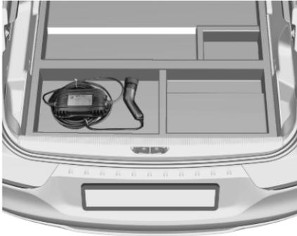
A portable charge cord used to charge the vehicle high voltage battery is stored under the rear floor storage cover in the load compartment ↗ 194. The charge cord is compatible with the domestic electrical outlet of the respective country. It includes a control box with charging status indicators.
