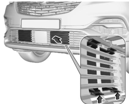
1. With your hand behind the grille, push the brackets of the protection cover upwards to release the protection cover.
