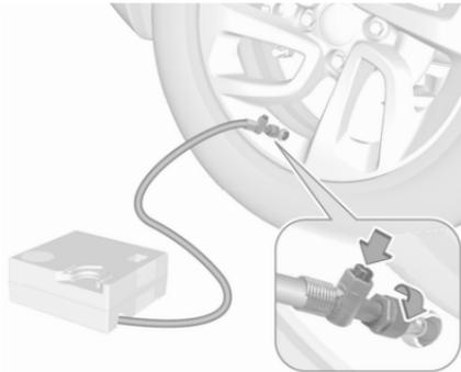
16. Continue driving immediately so that sealant is evenly distributed in the tyre. After driving approx. 3 miles but no more than 10 minutes, stop and check tyre pressure. Screw compressor air hose directly onto tyre valve when doing this. Fill tyre as described before. Drain excess tyre pressure with the button on the air hose.
