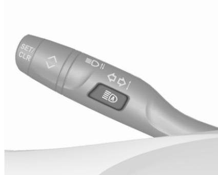
Activate the high beam assist by pressing
