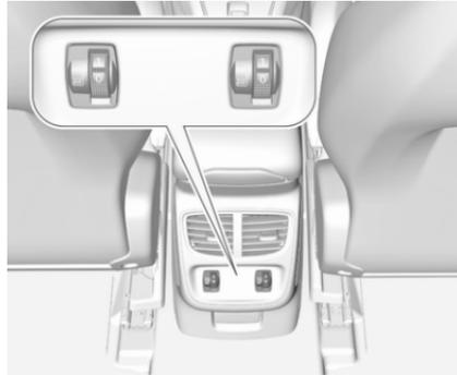
Adjust seat heating by turning thumb wheel
