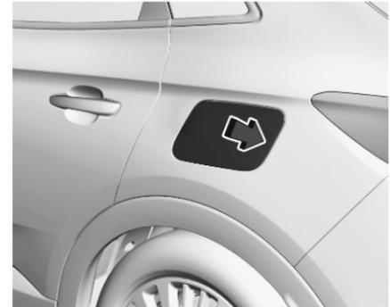
2. Push the rearward edge of the charge port door in and release to open the door.
