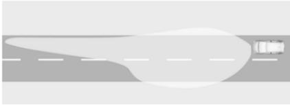
Activated automatically at a speed between 34 mph and 71 mph when driving in rural areas. The illumination of the current lane and the side of the road is improved. Oncoming and preceding vehicles are not dazzled.
