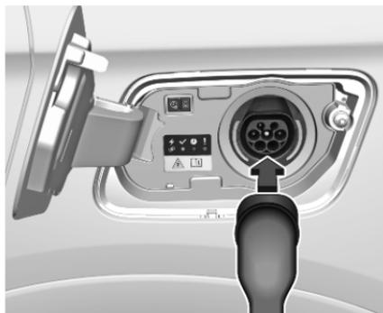
5. Plug in the vehicle plug of the charge cord into the charge port on the vehicle. Charging status ⇨ 198.
