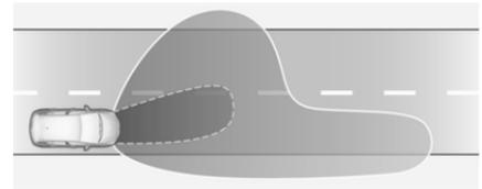
Controlled by wiper or rain sensor. The wide light distribution – slightly swiveled to the outside – enables improved orientation at the edge of the road. The intensity of the light in the far distance is increased in order
