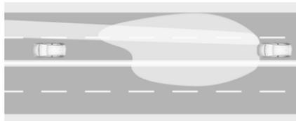
High beam assist includes a special motorway mode. When driving faster than 71 mph on motorways, the light beam becomes smaller to avoid dazzling of oncoming traffic. When following vehicles ahead or passing, dazzling for these vehicles is reduced.
