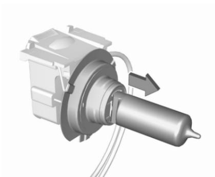
3. Detach the bulb from the bulb socket and replace the bulb.
