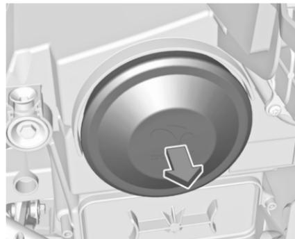
1. Remove the protective cover by pulling.
