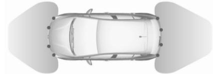
The system operates with ultrasonic parking sensors in the rear and front bumper.
