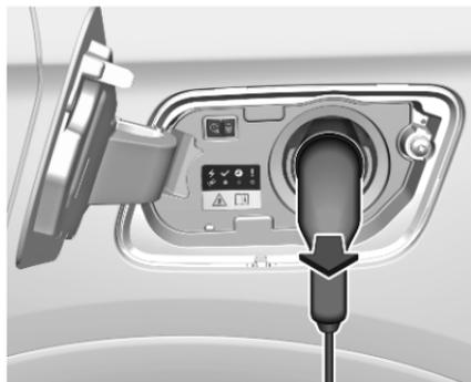
2. Disconnect the vehicle plug from the charge port within 30 seconds.
