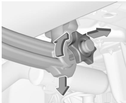
Open the protective flap and turn the key to position
