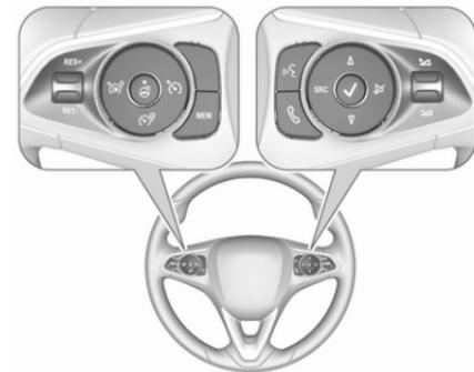
Cruise control and speed limiter are operated via the controls on the left side of the steering wheel.
