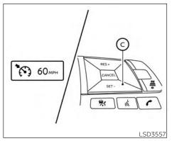
To set cruising speed, accelerate your vehicle to the desired speed, push the SET- © switch and release it. (The color of the cruise indicator changes to green and set vehicle speed indicator comes on.) Take your foot off the accelerator pedal. Your vehicle will maintain the set speed.
