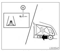
Operating vehicle-to-vehicle distance control mode
