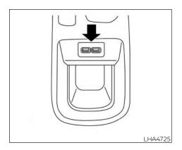
There are USB/iPod® charging ports located on the center console. These ports will charge compatible devices.
