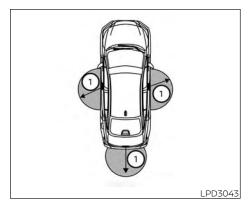
If the Intelligent Key is too close to the door glass, handle or rear bumper, the request switches (if so equipped) may not function.
