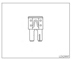
If any electrical equipment does not operate, check for an open fuse.
