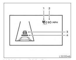
Vehicle-to-vehicle distance control mode display and indicators
