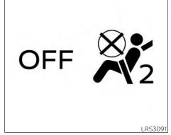
7. If the booster seat is installed in the front passenger seat, place the ignition switch in the ON position. The front passenger air bag status light of a may or may not illuminate, depending on the size of the child and the type of booster seat being used. For additional information, refer to "Front passenger air bag and status light" in this section.
