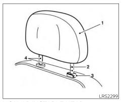
NON-ADJUSTABLE HEAD RESTRAINT/HEADREST **COMPONENTS**
