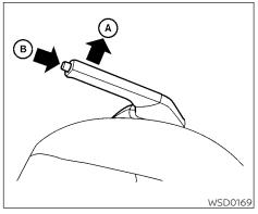
To engage: Pull the parking brake lever up (A)
