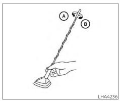
The rod antenna cannot be shortened, but can be removed. When you need to remove the antenna.turn the antenna rod counterclockwise (B).
