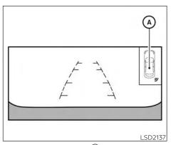
The system indicators (A) will appear when the vehicle moves closer to an object.
