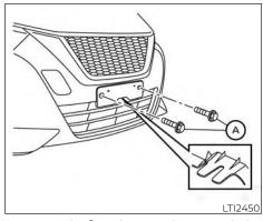
To mount the front license plate, attach the license plate bracket to the bumper fascia at the location marks (small dimples) using the two provided screws (A).
