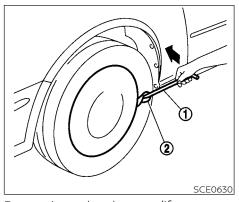
Removing wheel cover (if so equipped)
