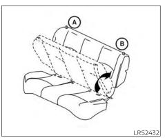
2. To return the rear seat to a seating position, lift up on the seatback and push it up to an upright position. Firmly press zones (A) and (B) to lock the seatback in place.
