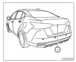
To display the rear view, the Rear View Monitor system uses a camera located just above the vehicle's license plate  $\widehat{\mathbf{1}}$ .
