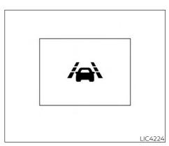
The Lane Departure Warning (LDW) switch is used to turn on and off the LDW system. When the LDW switch is pushed, the LDW system will turn on and the LDW indicator light on the switch will illuminate. When the LDW switch is pushed again, the LDW system will turn off and the LDW indicator light will turn off
