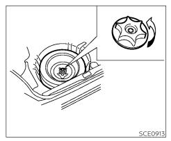
To remove the spare tire, loosen the bolt by turning counterclockwise. Once free, remove the bolt. Remove the spare tire.
