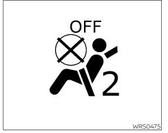
7. If the booster seat is installed in the front passenger seat, place the ignition switch in the ON position. The front passenger air bag status light images are not illuminate, depending on the size of the child and the type of booster seat being used. For additional information, refer to "Front passenger air bag and status light" in this section.
