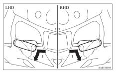
1- Firmly depress and hold the brake pedal, then pull the lever out slightly and turn it clockwise (LHD) or anticlockwise (RHD).
