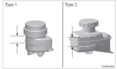
The brake fluid level is monitored by a float. When the brake fluid level falls below the "MIN" mark, the brake fluid warning lamp lights up.
