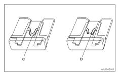
C- Fuse is OK D- Blown fuse
