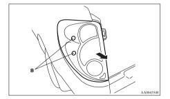
4. Remove each socket and bulb assembly by turning it anticlockwise.
