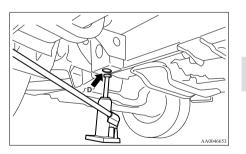
D- Front jacking point (2WD vehicles 16 inch wheels and 4WD vehicles)
