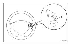
To slow down your speed in small amounts, press the "COAST SET" switch for less than about 1 second and release it.
