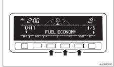
Press the "←" or "→" function button to select "km/L". Then press the "SET" function button. The display will flash twice, and the display unit will be updated to the selected one.
