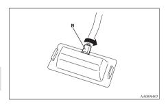
3. Remove the bulb by pulling out.
