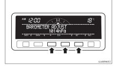
"+"- To adjust the barometer
