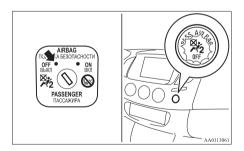
The front passenger's airbag OFF indication lamp will stay on to show that the front passenger's airbag is not operational. ("Front passenger's airbag OFF indication lamp" on page 2-30)
