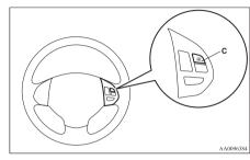
To increase your speed in small amounts, press the "ACC RES" switch for less than about 1 second and release it. Each time you press the "ACC RES" switch, your vehicle will go about 1.6 km/h (1 mph) faster.
