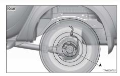
The ABS becomes operative after the vehicle has accelerated to a speed in excess of approximately 10 km/h (6 mph). It stops operating when the vehicle decelerates to a speed below approximately 7 km/h (4 mph).
