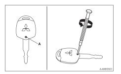
With the MITSUBISHI mark facing you, insert the cloth-covered tip of a straight blade (or minus) screwdriver into the notch in the remote control switch case and use it to open the case.
