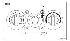
Push the switch again and the air conditioning compressor will stop and the indication lamp goes off.
