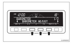
Adjust the barometer by pressing the function buttons
