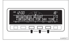
3. Use the function buttons to adjust the brightness.
