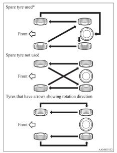
\*- If the spare tyre wheel differs from the standard tyre wheel, do not perform tyre rotation using a spare wheel.
