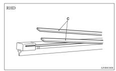
4. Insert the wiper blade into the arm, starting with the opposite end of the blade from the stopper. Make sure the hook (B) is fitted correctly in the grooves in the blade.
