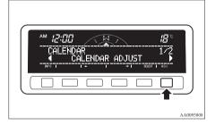
2. Press the "←" or "→" function button to select "CALENDAR ADJUST". Then press the "SELECT" function button.
