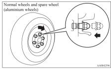
With a spare wheel, tighten the wheel nuts until the tapered parts of the wheel nuts make light contact with the seats of the wheel holes and the wheel is not loose.
