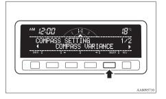
Press the function button for "←" or "→" to set the desired declination.
