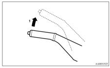
Firmly depress and hold the brake pedal, then pull the lever up without pushing the button at the end of hand grip.
