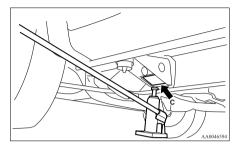
C- Front jacking point (2WD vehicles with 15 inch wheels)
