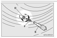
• When removing and screwing in the valve insert using the valve remover, turn the valve remover by hand. Using a tool to turn the valve remover could damage it.
