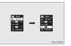
3. Press and hold the multi-information meter switch for approximately 2 seconds or more to switch in sequence from  $^{\circ}C \rightarrow ^{\circ}F \rightarrow ^{\circ}C$ .
