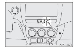
The system preparation time extends from the point at which all of the doors and the tailgate are locked by pressing the LOCK switch on the remote control switch or the keyless operation function to the point at which the system armed mode goes into effect.
