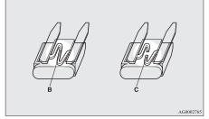
B- Fuse is OK C- Blown fuse
