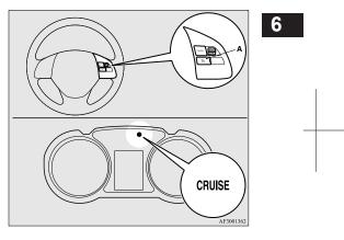
2. Accelerate or decelerate to your desired speed, then push down and release the SET - switch (B) when the "CRUISE" indication lamp is illuminated. The vehicle will then maintain the desired speed.
