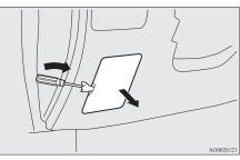
2. To put back the fuse lid, line up the fuse lid hook (A) with the clamp (B) on the instrument panel and push the lid back in.
