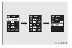
3. When you press and hold the multi-information meter switch for approximately 5 seconds or more, the buzzer sounds and all of the function settings are returned to the factory settings.
