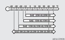
Use engine oil conforming to the following classification:
