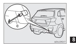
3. Use the wheel nut wrench (D) to firmly attach the towing hook.
