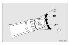
INT- The wiper operates continuously for several seconds then operates intermittently at intervals of about every 8 seconds
