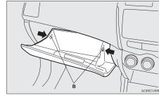
4. Remove the glove box fastener, and then remove the glove box.
