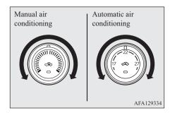
• While the engine coolant temperature is low, the temperature of the air from the heater will be cool/cold until the engine warms up, even if you have selected warm air with the dial.
