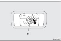
2. Move the lever (B) to open the tailgate.
