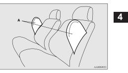
The label shown here is attached to the seatbacks with a side airbag.
