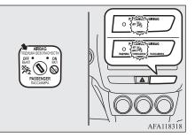
The front passenger's airbag is now deactivated and will not deploy until switched on again.
