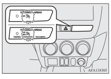
The indicator normally illuminates when the ignition switch is turned to the "ON" position or the operation mode is put in ON, and goes off a few seconds later.
