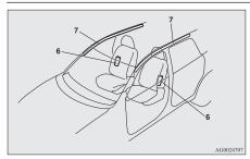
6- Side airbag modules\*7- Curtain airbag modules\*
