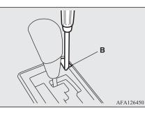
4. Insert a straight blade (or minus) screwdriver in the shift-lock release hole (A). Shift the selector lever to the "N" (NEU-TRAL) position while pressing the straight blade (or minus) screwdriver down.
