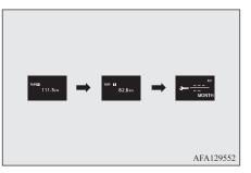
2. Press and hold the multi-information meter switch for approximately 2 seconds or more to display "—" and make it flash. (If there is no operation for approximately 10 seconds with flashing, the display returns to the previous screen.)
