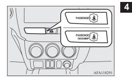
The lamp comes on when a person sits on the front passenger seat but does not fasten the seat belt. It goes off when the seat belt is subsequently fastened.
