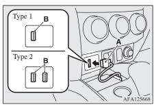
4. To remove the connector cable, turn the ignition switch to the "LOCK" position or put the operation mode in OFF first and perform the installation steps in reverse.
