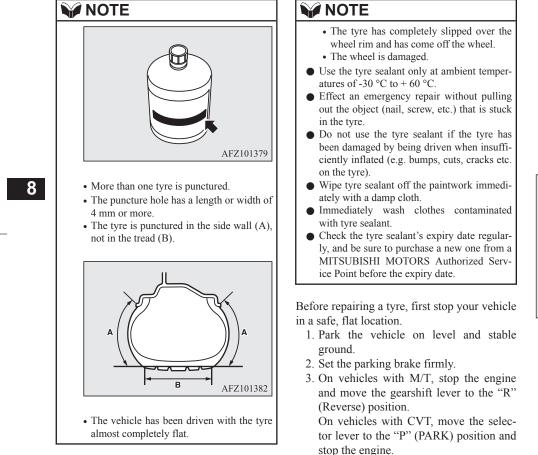
4. Turn on the hazard warning flashers and set up a warning triangle, flashing signal lamp, etc., at an adequate distance from the vehicle, and have all your passengers leave the vehicle.
