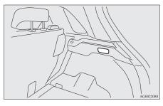
The lamp illuminates when the tailgate is opened, and goes out when the tailgate is closed.
