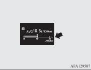
When the value of momentary fuel consumption surpasses the value of average fuel consumption, the momentary fuel consumption is displayed with a white bar graph. Be conscious of maintaining the value of mo-
