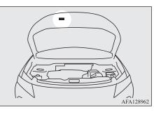
The plate shows model code, engine model, transmission model and body colour code, etc.
