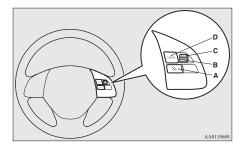
**A- CRUISE CONTROL ON/OFF switch** Used to turn on and off the cruise control.
