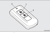
1- LOCK (A) switch 2- UNLOCK (A) switch 3- Indication lamp
