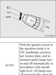
AUTOWith the ignition switch or<br/>the operation mode is in<br/>ON, headlamps, position,<br/>tail, licence plate, and in-<br/>strument panel lamps turn<br/>on and off automatically in<br/>accordance with outside<br/>light level. All lamps turn<br/>off automatically when the<br/>ignition switch is turned to<br/>"LOCK" position or the op-<br/>eration mode is put in OFF.≧D05Position, tail, licence plate<br/>and instrument panel lamps<br/>on<br/>Headlamps and other lamps<br/>go on
