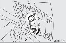
C- Stop lamp and tail lamp (LED) - cannot be replaced D- Rear turn-signal lamp
