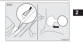
3. Remove the fuel cap. Open the fuel tank filler tube by slowly turning the cap anticlockwise.
