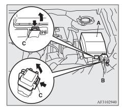
A- Main fuse block B- Sub fuse block\*
