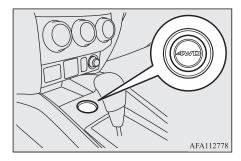
By pressing the drive mode-selector, the drive mode can be changed in order of "2WD", "4WD AUTO" and "4WD LOCK".
