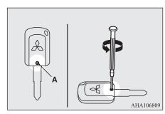
3. With the MITSUBISHI mark facing you, insert the cloth-covered tip of a straight blade (or minus) screwdriver into the notch in the remote control switch case and use it to open the case.
