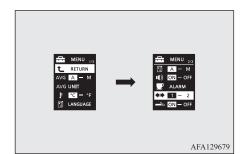
Press and hold the multi-information meter switch for approximately 2 seconds or more to switch in sequence from 1 (turn-signal sound 1) → (turn-signal sound 2) → 1 (turn-signal sound 1). The setting changes to the selected turnsignal sound.
