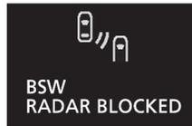
When the warning display appears, the sensor cannot detect a vehicle travelling side by side or an approaching vehicle, because foreign objects, such as dirt, snow or ice, adhere to the bumper surface around the sensor. Remove dirt, freezing or foreign material on the bumper surface around the sensor. When the warning display does not disappear after having cleaned the sensor, contact a MITSUBISHI MOTORS Authorized Service Point.
