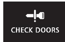
When the operation mode is in OFF, if you try to lock the doors and tailgate by pressing the driver's or front passenger's door lock/unlock switch, or the tailgate LOCK switch with one of the doors or the tailgate not completely closed, a warning is issued with the warning display and the buzzer buzzing for approximately 3 seconds and you cannot lock the doors and tailgate.
