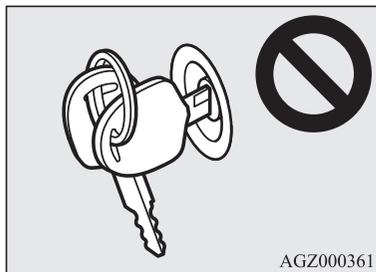
In cases like these, remove the object or additional key from the vehicle key. Then try again to start the engine. If the engine does not start, we recommend you to contact your MITSUBISHI MOTORS Authorized Service Point.
