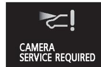
If the message remains even after the ignition switch is turned to the "LOCK" position and then turned back to the "ON" position or the operation mode is put in OFF, and then turned back to "ON", please contact a MITSUBISHI MOTORS Authorized Service Point.
