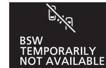
When the warning display appears, the sensor is temporarily not available for some reason such as the environmental condition or increase of the sensor temperature. When the warning display does not disappear after waiting for a while, contact a MITSUBISHI MOTORS Authorized Service Point.
