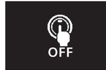
If the driver’s door is opened with the engine stopped and the operation mode in any position other than OFF, the operation mode ON reminder buzzer sounds intermittently to remind you to put the operation mode in OFF. In addition, the warning display will be displayed on the information screen in the multi-information display.
