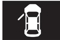
If any of the doors or the tailgate is not completely closed, this displays the open door or tailgate.
