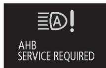
[When the sensor is malfunctioning]
