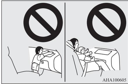
Use rearward facing child restraints in the rear seat or turn off the front passenger's airbag ON-OFF switch (if so equipped). (Refer to "To turn an airbag off" on page 4-27)
