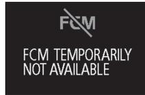
6 If the display keeps showing the message, there is a possibility that the FCM has a malfunction. Contact a MITSUBISHI MOTORS Authorized Service Point for inspection of the system.
