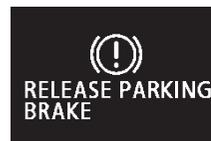
This warning is displayed if you drive with the parking brake still applied. The warning lamp in the instrument cluster only illuminates when the parking brake is applied.
