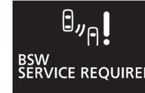
When the warning display appears, the BSW does not operate normally because there are some malfunctions in the system or the sensor. Have the vehicle inspected at a MITSUBISHI MOTORS Authorized Service Point as soon as possible.
