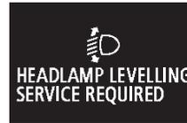
If there is a fault in the automatic headlamp levelling system, the warning display is displayed on the information screen in the multi-information display.
