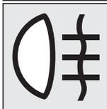
This lamp illuminates while the rear fog lamp is on.
