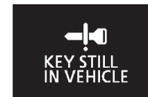
When the operation mode is in OFF, if you close all the doors and the tailgate with the keyless operation key left in the vehicle and you try to lock the doors and tailgate by pressing the driver’s or front passenger’s door lock/unlock switch, or the tailgate LOCK switch, a warning is issued with the warning display and the buzzer buzzing for approximately 3 seconds and you cannot lock the doors and tailgate.
