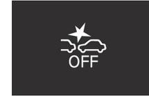
Cycling the ignition switch to the “ON” position or putting the operation mode in ON will set the FCM back ON.
