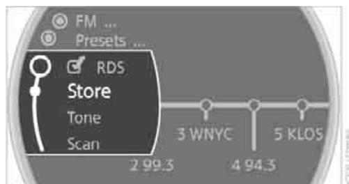
5. Turn the MINI joystick until the desired memory location is selected. The number of the memory location appears beside the name or frequency of the station.
