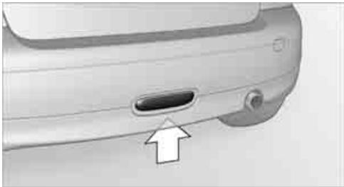
1. Screw out the bulb holder counterclockwise.
