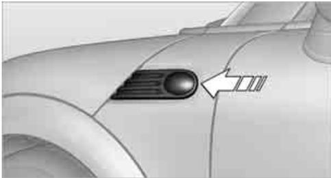
2. Screw out the bulb holder counterclockwise.
