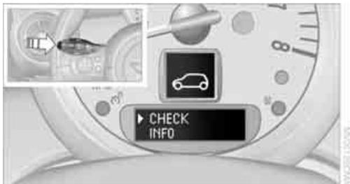
4. Hold the button down. "CHECK OK" appears if there are no Check Control messages. If a Check Control message has been stored, the corresponding message is displayed. In addition, the text message appears on the Control Display.
