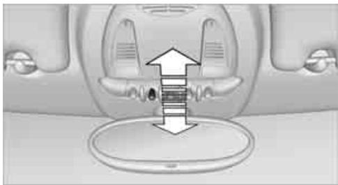
To switch the interior lamps on/off.
