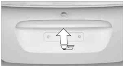
Press the button in the handle, arrow, or the
