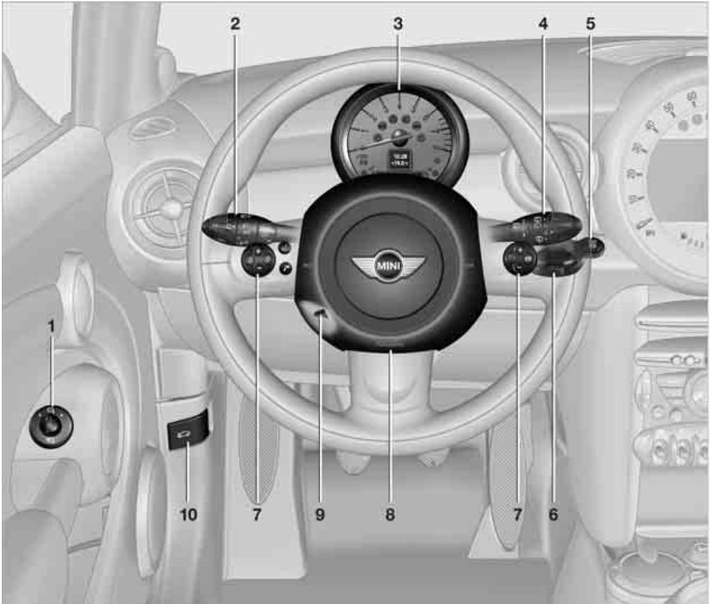
1 Adjusting the exterior mirrors, folding them in and out\* 40
