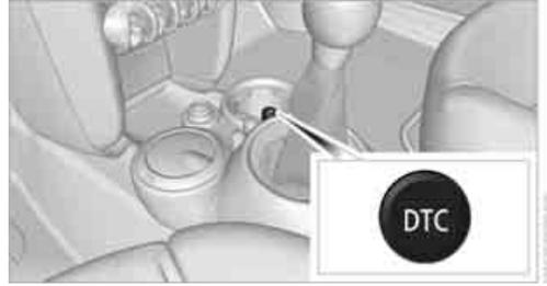
Press the button: the DTC indicator lamps come on.
