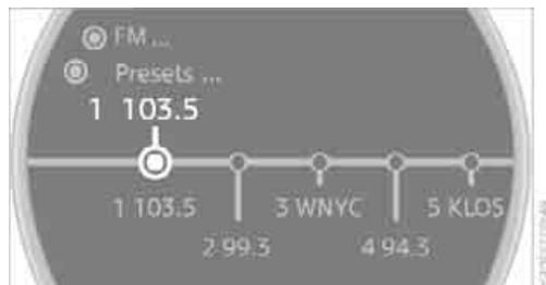
7. Press the MINI joystick. The station is stored.
