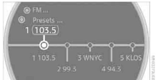
Some stations do not transmit the digital and analog signals simultaneously. If you are in an area in which digital reception of the selected station is not possible continuously, reception will alternate between analog and digital. This can cause repetitions or interruptions. In this case it may be preferable to switch off digital reception.
