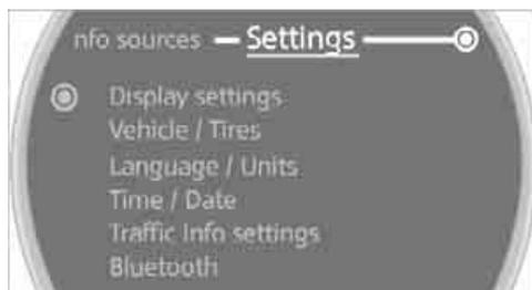
4. Turn the MINI joystick until "Time / Date" is selected and press the MINI joystick.
