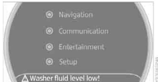
Text messages at the lower edge of the Control Display explain the meaning of the displayed indicator and warning lamps.
