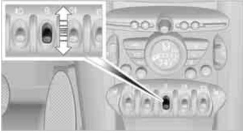
The switch locks or unlocks the doors and tailgate when the doors are closed, but the anti-theft system is not activated. The fuel filler door remains unlocked\*.
