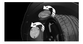
3. Unscrew the inner cover counterclockwise, and remove it.
