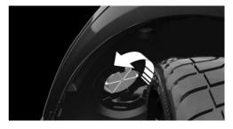
4. Turn the bulb socket counterclockwise and remove it from the bulb housing.
