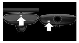
Photocells are used for control:
