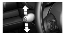
Press the lever past the resistance point. Canada: the lever returns into its starting position after actuation. To switch off manually, slightly tap the lever to the resistance point.
