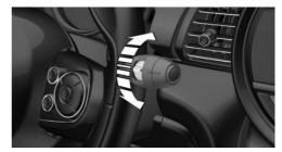
Turn the thumbwheel on the wiper lever.
