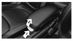
Press button, arrow 1, and swing center armrest upward or downward into the desired height, arrow 2.
