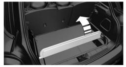
5-door models: To change the position of the cargo area floor, first fold up the rear part of the cargo area floor.
