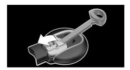
4. Push battery in the direction of the arrow using a pointed object and lift it 011f.
