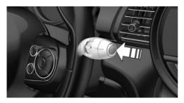
Press the button on the wiper lever.
