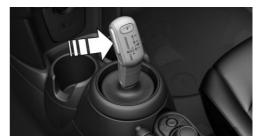
With the driver's safety belt fastened, briefly push the selector lever in the desired direction, past a resistance point,
