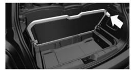
Fold up the cargo floor panel in the lower position and push it behind the locks, arrow. You've reached the maximum cargo height.
