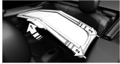
Press the wind deflector downward in the middle, until the handle engages, arrows 1.
