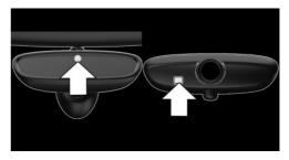
Photocells are used for control:
