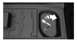
Unlock the locking hexagon of the emergency wheel well using the hexagon attached to retaining plate.
