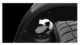
Turn the bulb socket counterclockwise and remove it from the bulb housing.
