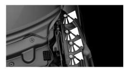
Turn the bulb socket counterclockwise and remove.
