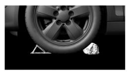
Place wheel chocks or other suitable objects in front and behind the wheel that is diagonal to the wheel to be changed.
