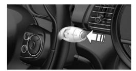
Press the button on the wiper lever.
