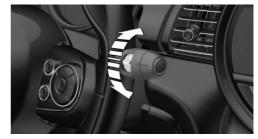
Turn the thumbwheel on the wiper lever.
