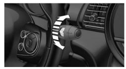
Turn the thumbwheel on the wiper lever.
