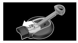
Push battery in the direction of the arrow using a pointed object and lift it out.
