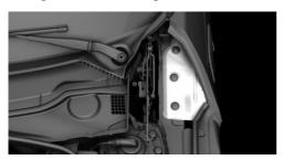
2. Loosen nuts of the cover by hand and remove the cover.
