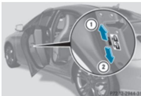
You secure each door individually with the child-proof locks on the rear doors. A door secured with a child-proof lock cannot be opened from inside the vehicle. When the
