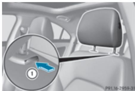
▶ **To raise:** pull the head restraint up to the desired position.
