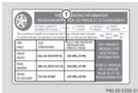
Option 2) **Tire pressure table** on the inside of the fuel filler flap.
