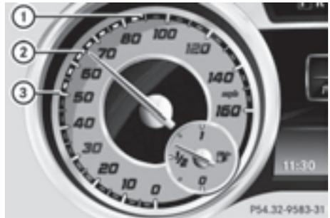
Example: DISTRONIC PLUS displays in the speedometer
