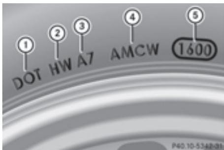
Canadian tire regulations prescribe that every new tire manufacturer or retreader has to imprint a TIN in or on the sidewall of each tire produced.
