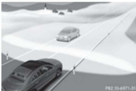
The extended range fog lamps reduce the glare experienced by the driver and improve the illumination of the edge of the road.
