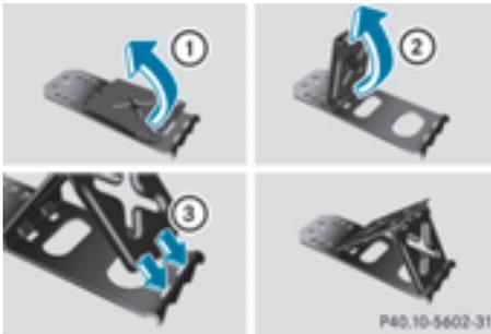
If your vehicle is equipped with a wheel chock, it can be found in the tire-change tool kit (▷ page 296).
