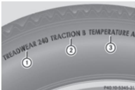
Uniform Tire Quality Grading Standards are U.S. government specifications. Their purpose is to provide drivers with uniform reliable information on tire performance data. Tire manufacturers have to grade tires using three performance factors: tread wear ①, tire traction ②, and heat resistance ③. These regulations do not apply to Canada. Nevertheless, all tires sold in North America are provided with the corresponding quality grading markings on the sidewall of the tire.
