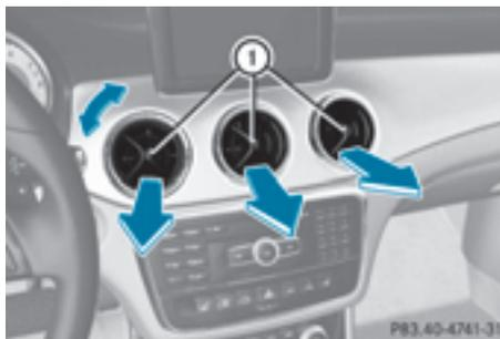
► **To open the center air vent:** turn the adjuster in one of center air vents ① counter-clockwise.
