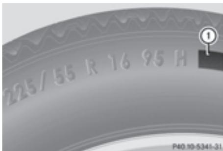
In addition to the load bearing index, load index ① may be imprinted after the letters that identify speed index ⑥ (▷ page 330) on the sidewall of the tire.
