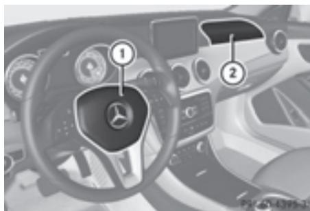
Driver's air bag ① deploys in front of the steering wheel; front-passenger front air
