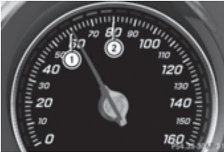
If DISTRONIC PLUS detects a vehicle in front, segments between the speed of the vehicle in front ① and stored speed ② light up.
