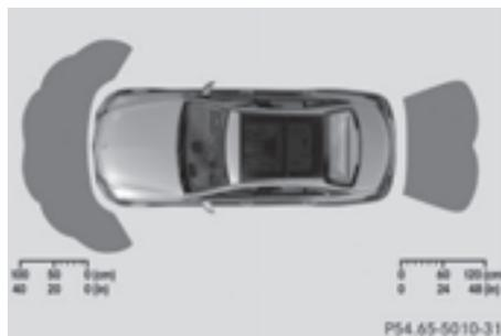
The sensors must be free from dirt, ice or slush. They can otherwise not function correctly. Clean the sensors regularly, taking care not to scratch or damage them (▷ page 339).
