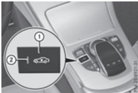
It is possible to choose between the "Normal" and "Raised" vehicle levels below a speed of 50 mph (80 km/h). Select the "Normal" setting for normal road surfaces and "Raised" for driving with snow chains or on particularly poor road surfaces. Your selection remains stored even if you remove the SmartKey from the ignition lock.
