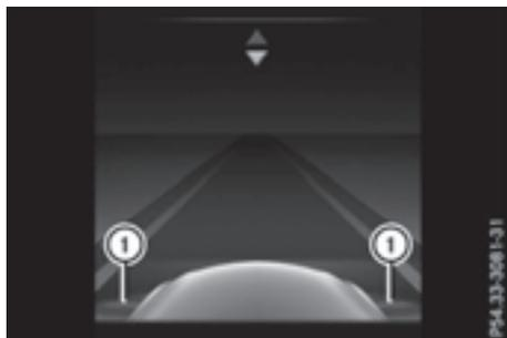
When Blind Spot Assist is activated, gray radar waves propagating backwards appear next to the vehicle in the assistance display in the multifunction display. Above a speed of 20 mph (30 km/h), the color of the radar waves in the assistance display changes to green ①. Blind Spot Assist is then ready for use.
