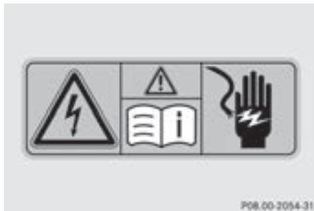
All components of the hybrid drive system are marked with yellow warning stickers that warn you of the danger of high voltage. The cables of the vehicle's high-voltage electrical system are orange in color.
