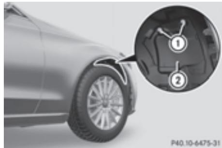
You must remove the cover of the front wheel housing before you can change the front turn signal lamp.
