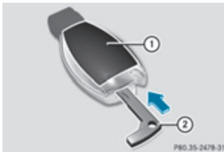
► Press mechanical key ② into the SmartKey opening in the direction of the arrow until battery compartment cover ① opens. Do not hold battery compartment cover ① closed while doing so.
