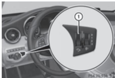
The lighting in the instrument cluster, in the displays and the controls in the vehicle interior can be adjusted using brightness control knob ①.
