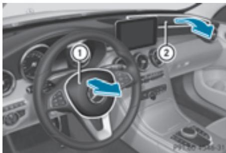
Driver's air bag ① deploys in front of the steering wheel. Front-passenger front air bag ② deploys in front of and above the glove box. When deployed, the front air bags offer additional head and thorax protection for the occupants in the front seats.
