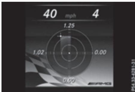
The G-Meter shows you the forces working on the driver in longitudinal and lateral direction while driving.
