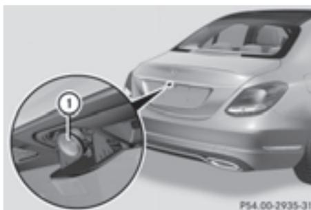
Rear view camera ① is an optical parking and maneuvering aid. It shows the area behind your vehicle with guide lines in the multimedia system.
