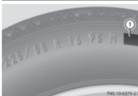
In addition to the load-bearing index, load index ① may also be imprinted on the sidewall of the tire. You will find this after the letter that identifies the speed rating (▷ page 374).
