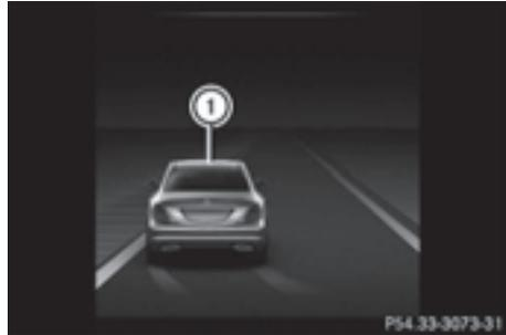
If a lane-correcting brake application occurs, display ① appears in the multifunction display. The brake application also slightly reduces vehicle speed.
