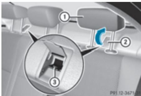
Top Tether anchorage points ③ are installed in the rear compartment behind the outer head restraints on the parcel shelf.
