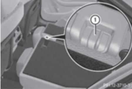
In order to prevent the trunk from being accessed by unauthorized persons, the center seat backrest can be locked using a catch. The center seat backrest can only be folded forward together with the left seat backrest.
