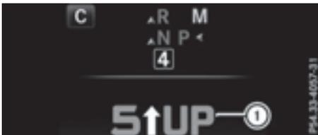
Before the engine speed reaches the red area, an upshift indicator will be shown in the multifunction display.
