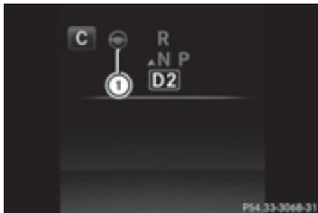
If Steering Assist and Stop&Go Pilot are activated but is not ready for a steering intervention, steering wheel symbol ① appears in gray. If the system provides you with support by means of steering interventions, symbol ① is shown in green.
