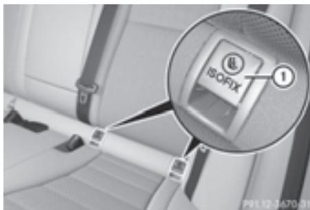
**Vehicles with rear seat armrest:** adjust the rear seat armrest so that LATCH-type (ISOFIX) securing rings ① for the LATCH-type (ISOFIX) child restraint system are accessible.
