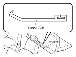
7. Set the hook on the support bar in the rear of the seatback.
