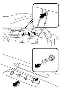
An unsecured high-mount brake lights will allow water to leak into the vehicle. Make sure the high-mount brake light is tightly fastened to the vehicle and if water still leaks, consult an Authorized Mazda Dealer.
