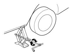
Remove the lug nuts by turning them counterclockwise; then remove the wheel.
