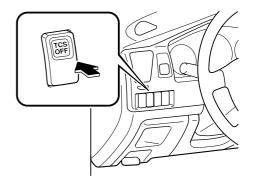
Press the switch again to turn the TCS back on. The TCS OFF indicator light will go out.
