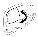
To lock either front door with the door-lock button from the outside, push its door-lock button and close the door.
