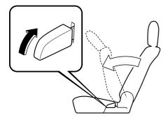
Raise the seatback to the most upright position. Make sure the seatback is securely latched by rocking the seatback.
