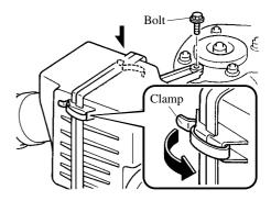
2. Separate the air cleaner housing and remove the filter.
