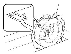
9. Secure the flat tire with the tire clamp and wing nut as shown below. Have the damaged tire repaired as soon as possible.
