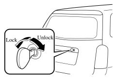
The liftgate can be locked/unlocked by inserting the key into the key slot of any door, refer to Power Door Locks (page 3-10).
