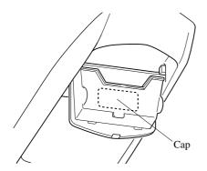
4. Store the garage door opener by adjusting the thickness with the urethane spacers.
