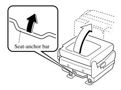
The seat is heavier than it looks, carefully pull up and detach the seat. Get assistance to lift it out of the vehicle.
