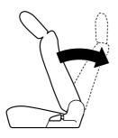
4. Expand the area between the seat bottom and the seatback slightly to verify the locations of the LATCH lower anchors.
