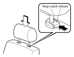
Adjust the head restraint so that the top is parallel with the top of the passenger's ears, never the passenger's neck.
