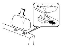
Adjust the head restraint so that the top is parallel with the top of the passenger's ears, never the passenger's neck.
