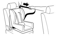
4. Push the child-restraint system firmly into the vehicle seat. Be sure the belt retracts as snugly as possible. Adjust the angle of the seat belt buckle so that the belt is not loose. Clicking from the retractor will be heard during retraction if the system is in the automatic locking mode. If the belt does not lock the seat down tight, repeat this step.
