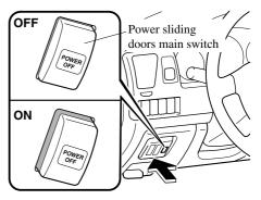
ON: Switches on electric power to power sliding doors.
