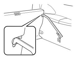
8. Pull the seatback towards the front of the vehicle until the opposite end of the support bar hooks onto the anchor loop in the side trim. Attempt to push the seatback towards the rear (liftgate) to make sure the support bar is securely latched.
