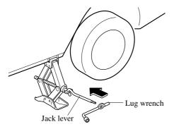
5. Turn the lug wrench clockwise and raise the vehicle high enough so that the spare tire can be installed. Before removing the lug nuts, make sure your Mazda is firmly in position and that it cannot slip or move.
