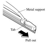
Remove the metal stiffeners from the blade rubber and install them in new blades.
