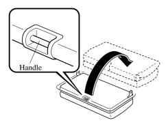
5. Pull strap A and raise the seatback upright. Attempt to move the seatback forward and backward to make sure it is locked.
