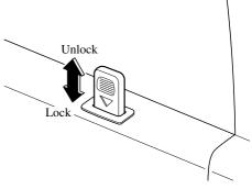
To lock a sliding door with the door-lock button from the outside, push down its door-lock button and close the door.
