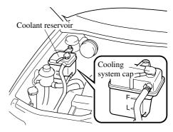
If you find no problems, the engine is cool, and no leaks are obvious, carefully add coolant as required (page 8-11).
