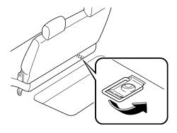
8. Install the flat tire with the tire securing bolt hooked in the anchor clip as shown below.
