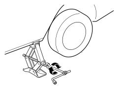
6. Remove the lug nuts by turning them counterclockwise; then remove the wheel.
