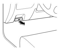
2. Pull the hood latch up and lift the hood.
