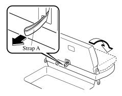
4. Pull strap B and lift the combined seatback and seat bottom up to vertical with your other hand. Gently lower the seat into the seat well.
