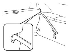
9. Pull the seatback towards the front of the vehicle until the opposite end of the support bar hooks onto the anchor loop in the side trim. Attempt to push the seatback towards the rear (liftgate) to make sure the support bar is securely latched.
