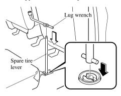
Slowly turn the lug wrench counterclockwise until the spare tire reaches the ground and the cable becomes loose.
