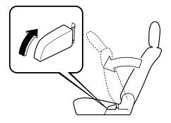
Raise the seatback to the most upright position. Make sure the seatback is securely latched by rocking the seatback.
