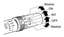
Turn the wiper on by turning the rear wiper/washer switch.
