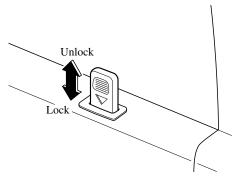
To lock a sliding door with the door-lock knob from the outside, push down the door-lock knob and close the door.
