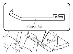
8. Set the hook on the support bar in the rear of the seatback.
