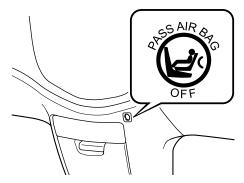
If the front passenger weight sensors are normal, the indicator light illuminates when the ignition switch is turned to the ON position. After about 6 seconds it goes out.
