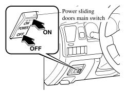
ON: Switches on electric power to power sliding doors.
