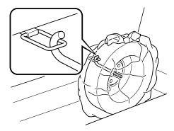
Secure the flat tire with the tire clamp and wing nut as shown below.
