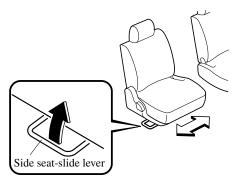
Make sure the lever returns to its original position and the seat is locked in place by attempting to push it from side to side.
