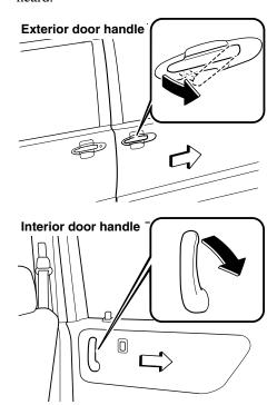
When the doors are completely open and a door is slid by the handle 5 cm (2 in) in the direction of closing, the doors will completely close automatically after the beep sound is heard.
