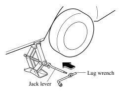
5. Turn the lug wrench clockwise and raise the vehicle high enough so that the spare tire can be installed. Before removing the lug nuts, make sure your Mazda is firmly in position and that it cannot slip or move.
