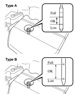
5. Pull it out again and examine the level. The level is normal if it is between Low and Full. If it is near or below Low, add enough oil to bring the level to Full.
