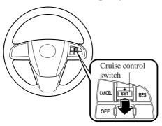
Your vehicle has a tap-down feature that allows you to decrease your current speed in decrements of 1.6 km/h (1 mph) by a momentary tap of the cruise control SET-switch. Multiple taps will decrease your vehicle speed 1.6 km/h (1 mph) for each tap.
