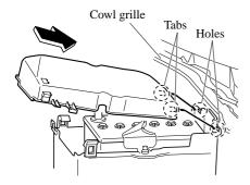
2 Attach the clips on both sides of the battery cover.
