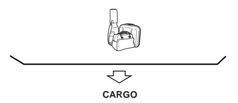
**Cargo Weight** includes all weight added to the Base Curb Weight, including cargo and optional equipment.
