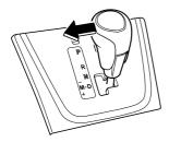
To return to automatic shift mode, shift the lever from M to D.
