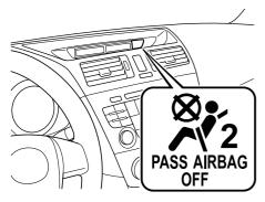
If the front passenger weight sensors are normal, the indicator light illuminates when the ignition is switched ON. The light turns off after a few seconds. Then, the indicator light illuminates or is off under the following conditions:
