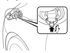
4. Turn the bulb assembly counterclockwise and remove it.
