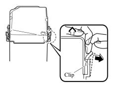
2 Detach the clip facing the vehicle interior first and pull it outward with your finger approx. 4 mm (0.2 in). Then, lift the cover slightly to clear the lock.
