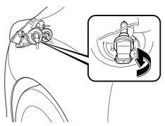
Install the new bulb in the reverse order of the removal procedure.
