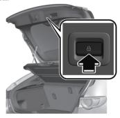
When locking using the door-lock switch, press the door-lock switch with all of the following conditions met and then close the liftgate.
