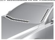
The windshield wiper de-icer operates in conjunction with the rear window defogger.
