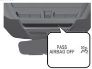
If the front passenger weight sensors are normal, the indicator light illuminates when the ignition is switched ON. The light turns off after a few seconds. Then, the indicator light illuminates or is off under the following conditions:
