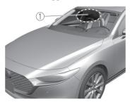
1. Forward Sensing Camera (FSC)
