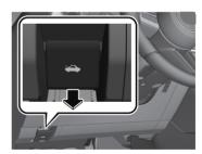
Insert your hand into the hood opening, slide the latch lever to the left, and lift up the hood.
