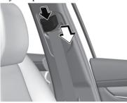
After adjusting, press the front shoulder belt adjuster downward and make sure that it is securely locked.
