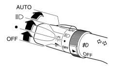
Turn the headlight switch to turn the headlights, other exterior lights and dashboard illumination on or off.
