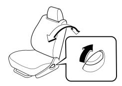
Make sure the lever returns to its original position and the seatback is locked in place by attempting to push it forward and backward.
