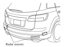
Always keep the bumper surface near the radar sensor area clean so that the BSM system operates normally. Refer to the Exterior Care (page 8-54).
