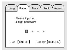
2. Press the ENTER button. If the password is confirmed, the Rating change mode is displayed.
