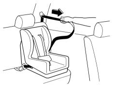
5. Push the child-restraint system firmly into the vehicle seat. Be sure the belt retracts as snugly as possible. Clicking from the retractor will be heard during retraction if the system is in the automatic locking mode. If the belt does not lock the seat down tight, repeat this step.
