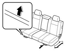
Make sure the bar returns to its original position and the seat is locked in place by attempting to push it forward and backward.
