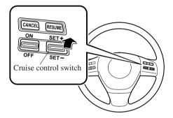
Your vehicle has a tap-up feature that allows you to increase your current speed in increments of 1.6 km/h (1 mph) by a momentary tap of the cruise control switch. Multiple taps will increase your vehicle speed 1.6 km/h (1 mph) for each tap.
