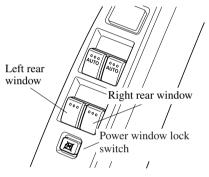
To open the power window to the desired position, hold down the switch. To close the power window to the desired
