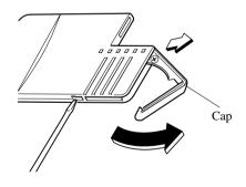
Do not turn the cap excessively. The cap may be damaged.
