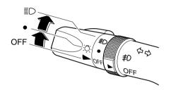
Turn the headlight switch to turn the headlights, other exterior lights and dashboard illumination on or off.
