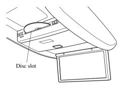
Insert the disc with its label-side (decorated side) facing upward. If the disc is inserted upside-down, it may cause a malfunction.
