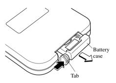
2. Remove the old battery and install a new one with the plus pole pointed up.
