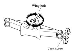
3. Turn the wing bolt completely to secure the jack.
