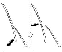
To prevent damage to the windshield let the wiper arm down easily, don't let it slap down on the windshield. 5. Pull down the blade rubber and slide it out of blade holder.
