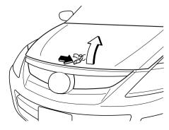
3. Grasp the support rod in the padded area and secure it in the stay hole indicated by the arrow to hold the hood open.
