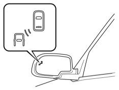
This warning light illuminates for a few seconds when the ignition switch is turned to the ON position.
