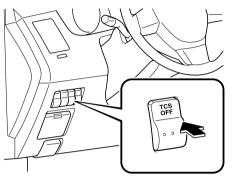
Press the switch again to turn the TCS back on. The TCS OFF indicator light will go out. If the vehicle speed is more than 15 km/h (9 mph), the TCS OFF indicator light will not illuminate even if the switch is pressed.
