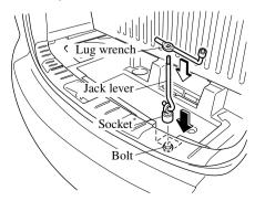
5. Slowly turn the lug wrench counterclockwise until the spare tire reaches the ground and the cable becomes loose.
