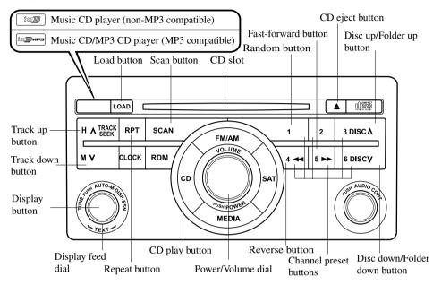
There are two types of In-dash CD changers. Check which In-dash CD changer your vehicle is equipped with.
