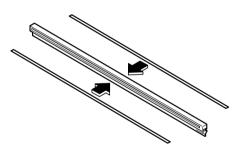
5. Carefully insert the new blade rubber. Then install the blade assembly in the reverse order of removal.
