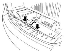
3. Turn the wing bolt and jack screw counterclockwise.
