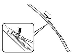
**NOTE** Using a soft cloth-wrapped flathead screwdriver.
