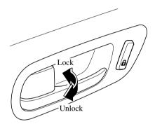
To lock any door with the door-lock knob from the outside, push the door-lock knob to the lock position and close the door. This does not operate the other door locks.
