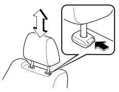
Adjust the head restraint so that the top is even with the top of the passenger's ears, never the passenger's neck to prevent injury.
