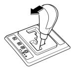
To return to automatic shift mode, shift the lever from M to D.
