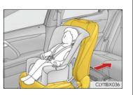
If the head restraint interferes with the installation of the child restraint system, and the head restraint can be removed, remove the head restraint. If the head restraint cannot be removed, raise it to the uppermost position.
