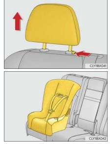
**4** Run the seat belt through the child restraint system and insert the plate into the buckle. Make sure that the belt is not twisted.
