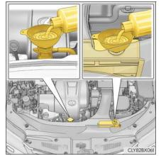
**6** Start the hybrid system and turn the air conditioning system on to check that the radiator cooling fans operate and to check for coolant leaks from the radiator or hoses.
