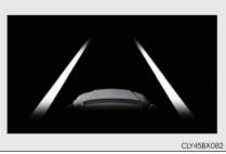
Indicates that the system is recognizing white (yellow) lines. When the vehicle departs from its lane, the white line displayed on the side the vehicle departs
