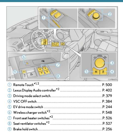
\*1: For vehicles with a navigation system, refer to "NAVIGATION SYSTEM OWNER'S MANUAL". \*2: If equipped
