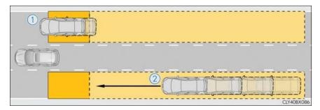
(1) Vehicles that are traveling in areas that are not visible using the outside rear view mirrors (the blind spots)
