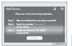
A PIN code are not required for SSP (Secure Simple Pairing) compatible Bluetooth  $^{\textcircled{R}}$  devices. Depending on the device, you may need to select Yes to register, or No to cancel on the device.
