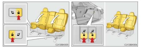
When using the seatback angle adjustment switch: If the rear seatback is reclined, adjust it to the most upright position and then press the switch again.
