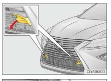
3 Insert the towing eyelet into the hole and tighten partially by hand.
