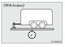
Additional optional equipment, passengers and cargo in the vehicle will reduce the trailer weight rating so as not to exceed GCWR, GVWR and GAWR. If the gross trailer weight exceeds 3000 lb. (1360 kg), it is recommended to use a trailer with 2 or more axles.
