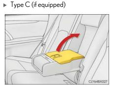
Pull up the lever to release the lock, and lift the lid.
