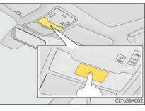
Turns the door position on/off ① On ② Off
