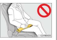
• The SRS front passenger airbag also deploys with considerable force, and can cause death or serious injury especially if the front passenger is very close to the airbag. The front passenger seat should be as far from the airbag as possible with the seatback adjusted, so the front passenger sits upright.
