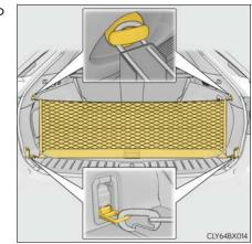
To hang the cargo net, use the cargo net hooks and rear cargo hooks.
