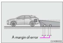
The estimated course lines target a flat surfaced objects (such as the road). It is not possible to determine the position of three-dimensional objects (such as vehicles) using the estimated course lines and distance guide lines. When approaching a three-dimensional object that extends outward (such as the flatbed of a truck), be careful of the following.
