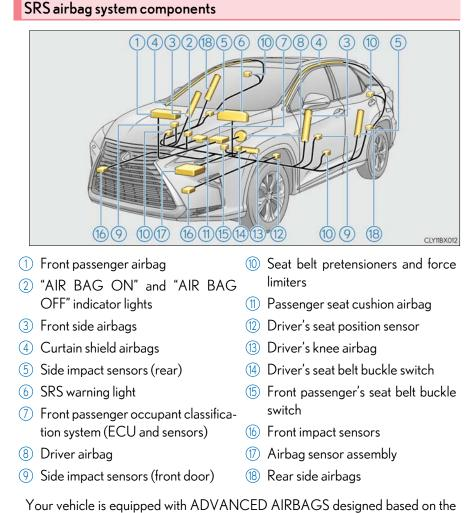
US motor vehicle safety standards (FMVSS208). The airbag sensor assembly (ECU) controls airbag deployment based on information obtained from the sensors etc. shown in the system components diagram above. This information includes crash severity and occupant information. As the airbags deploy, a chemical reaction in the inflators quickly fills the airbags with non-toxic gas to help restrain the motion of the occupants.
