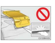
Use caution when using the back door closer as it still operates when the power back door system is disabled.
