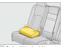
4 Sit the child in the child restraint system. Fit the seat belt to the child restraint system according to the manufacturer's instructions and insert the plate into the buckle. Make sure that the belt is not twisted.
