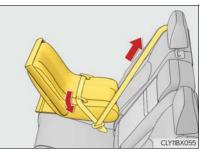
6 After installing the child restraint system, rock it back and forth to ensure that it is installed securely. (→P. 66)
