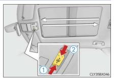
\*: Quickly slide and release the is switch in either direction to stop the electronic sunshade partway.
