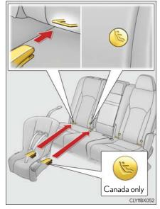
If the child restraint has a top tether strap, follow the child restraint manufacturer's operation manual regarding the installation, using the top tether strap to latch onto the top tether strap anchor. (→P. 70)
