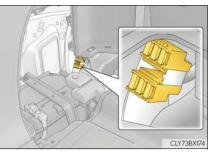
Remove the deck board and side auxiliary box cover and 12-volt battery cover. ( $\rightarrow$ P. 606)
