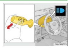
**2** Press the Automatic High Beam switch.
