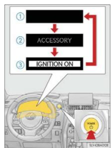
If the hybrid system is stopped with the shift lever in a position other than P, the power switch will not be turned off but instead be turned to ACCESSORY mode. Perform the following procedure to turn the switch off:
