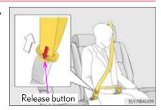
Insert the mechanical key ( $\rightarrow$ P. 118) or plate B into the notch of buckle A and remove the belt.
