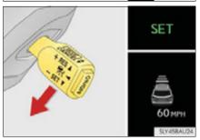
While the vehicle is in vehicle-to-vehicle distance control mode, if the lever is released when vehicle speed is less than 30 mph (50 km/h) and a vehicle ahead can be detected, the vehicle will start following the vehicle ahead at a set speed of 30 mph  $(50 \, \text{km/h})$ .
