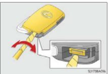
3 Remove the depleted battery.
