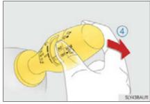
■ The rear window wiper and washer can be operated when The power switch is in ON mode.
