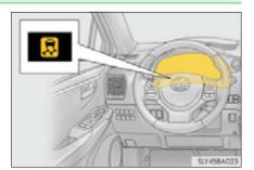
If the vehicle gets stuck in mud, dirt or snow, the TRAC system may reduce power from the hybrid system to the wheels. Pressing to turn the system off may make it easier for you to rock the vehicle in order to free it.
