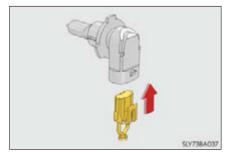
Align the 3 tabs on the light bulb with the mounting, and insert. Turn it clockwise to set.
