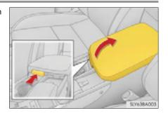
Vehicles with the wireless charger: Lift the wireless charger.
