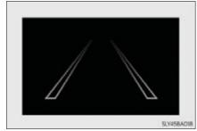
In steering control, the steering control indicator will come on.
