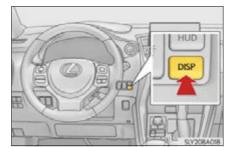
On and off will be switched between each time the button is pressed. If the button is left alone without being operated for a short time, setting will be finished automatically.
