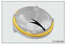
6 Replace the light bulb, and set the connector
