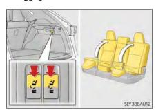
2 Check that the plate for the seat belt is on the front side of the seat. When using the seat belt for the rear center seat (→P. 33)
