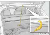
When attaching the side deck board, attach it so that the "TFRONT" mark points to the front side of the vehicle.
