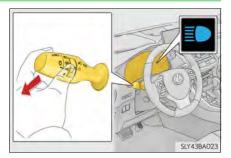
**2** Press the Automatic High Beam switch.
