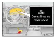
4 Press the power switch shortly and firmly.
