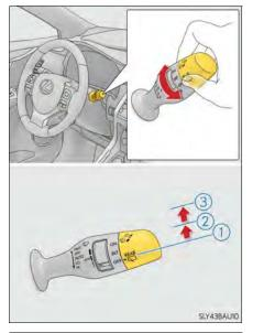
Washer/wiper dual operation The wipers will automatically operate a couple of times after the washer squirts.
