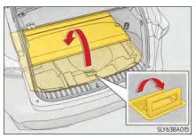
4 Lift the deck board and remove the hook on the backside of the deck board.
