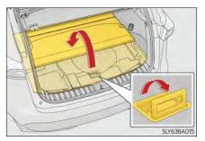
When the seatback for the rear seat is collapsed to the rear, remove the cover after the cover most upright position.  $(\rightarrow P.152)$
