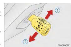
In the vehicle-to-vehicle distance control mode, the set speed will be increased or decreased as follows:
