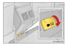
The power outlet can be used when the power switch is in ON mode.
