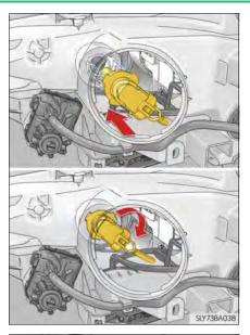
**8** Confirm the installation of the bulb base.
