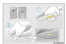
2 Touch the lock sensor (the indentation on the surface of the door handle) to lock all the doors.
