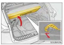
5 Attach the hook to the upper edge of the back door opening as shown.
