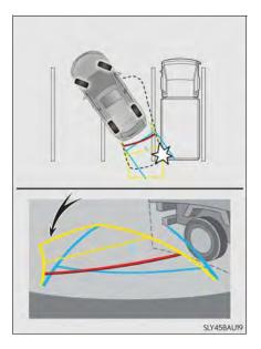
Visually check the surroundings and the area behind the vehicle. On the screen, it appears that a truck is parking at point ②. However, in reality if you back up to point ①, you will hit the truck. On the screen, it appears that ① is closest and ③ is farthest away. However, in reality, the distance to ① and ③ is the same and ② is farther than ① and ③.
