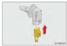
Align the 3 tabs on the light bulb with the mounting, and insert. Turn it clockwise to set.
