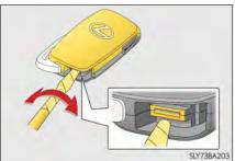
Remove the depleted battery.
