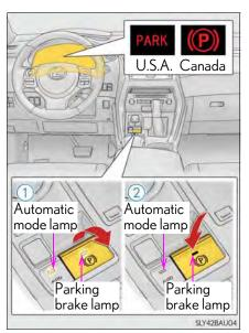
The parking brake can be set and released manually.
