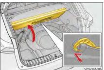
**5** Attach the hook to the upper edge of the back door opening as shown.
