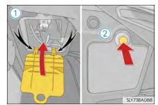
9 Install the engine compartment cover.  $(\rightarrow P.533)$
