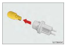
Replace the light bulb, and install the bulb base.
