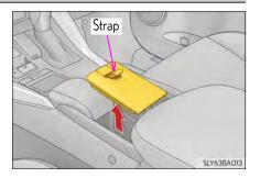
• The removed the lid of the sunglass holder can be stored on the tray in the console box.
