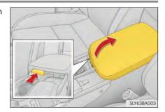
**2** Vehicles with the wireless charger: Lift the wireless charger.
