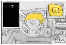
Press or v of the meter control switch, select the "TPMS" screen and then press and hold the □.
