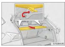
**5** Stow the luggage cover in the deck under tray while lifting the deck board.
