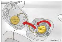
Remove the cover inside the luggage compartment by inserting a screwdriver. After removing the cover, pull the lever to unlock the fuel filler door and it will be ready to open as usual.
