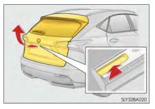
While carrying the electronic key on your person, press the back door opener switch.
