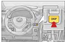
On and off will be switched between each time the button is pressed.
