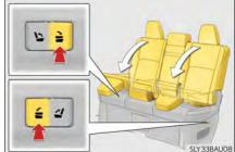
When the seatback is collapsed to the rear, put the seatback in the most upright position and press the switch once again.
