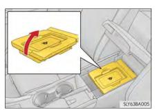
Vehicles without the wireless charger: The tray slides forward/backward and can be removed.
