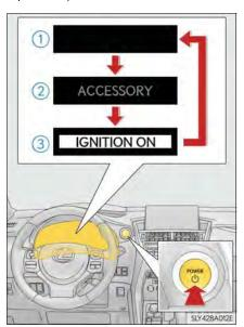
If the hybrid system is stopped with the shift lever in a position other than P, the power switch will not be turned off but instead be turned to ACCESSORY mode. Perform the following procedure to turn the switch off:
