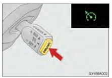
Accelerate or decelerate, with accelerator pedal operation, to the desired vehicle speed (above approximately 25 mph [40 km/h]) and push the lever down to set the speed.
