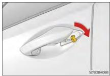
3 Remove the key, return the handle, and then pull the handle again.
