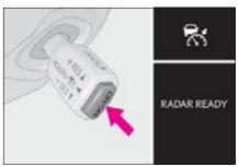
2 Accelerate or decelerate, with accelerator pedal operation, to the desired vehicle speed (at or above approximately 30 mph (50 km/h)) and push the lever down to set the speed.
