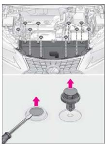
■ Installing the clips
