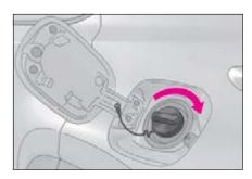
2 Close the fuel filler door, and press the center of the rear edge of the fuel filler door.
