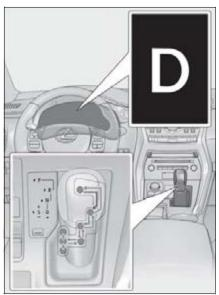
While the power switch is in ON mode, move the shift lever with the brake pedal depressed.
