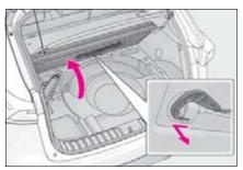
4 Use the hook to secure the deck board as shown in the illustration.
