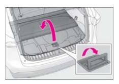
3 Lift the deck board and remove the hook on the backside of the deck board.
