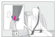
2 Insert the mechanical key (→P.100) or plate B into the notch of buckle and remove the belt.
