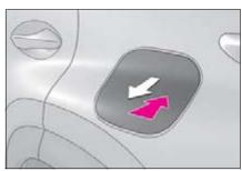
2 Turn the fuel tank cap slowly to open and put it into the holder on the fuel filler door.
