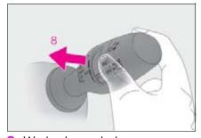
8 Washer/wiper dual operation The wipers will automatically operate a couple of times after the washer squirts.
