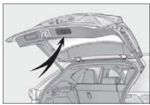
Opening/closing the back door using the kick sensor (vehicles with hands free power back door)
