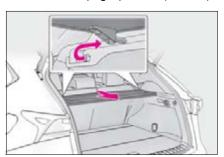
Stow the luggage cover in the deck under tray while lifting the deck board.
