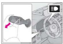
2 Press the Automatic High Beam switch.
