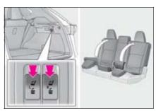
Check that the plate for the seat belt is on the front side of the seat.
