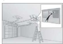
Press and release the "Learn" or "Smart" button. Perform 3 within 30 seconds after performing 2.
