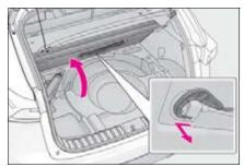
**4** Use the hook to secure the deck board as shown in the illustration.
