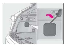
2 After removing the cover, pull the lever to unlock the fuel filler door and it will be ready to open as usual.
