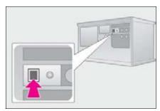
3 Press and hold the desired Home-Link<sup>®</sup> button (inside the vehicle) for 2 seconds and release it. Repeat this sequence (press/hold/release) up to 3 times to complete programming.
