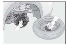
2 Install the spare tire and loosely tighten each wheel nut by hand by approximately the same amount.
