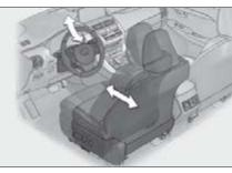
When all of the following have been performed, the driver's seat and steering wheel are automatically adjusted to a position that allows driver to enter and exit the vehicle easily.
