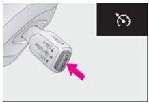
Accelerate or decelerate, with accelerator pedal operation, to the desired vehicle speed (at or above approximately 25 mph [40 km/h]) and push the lever down to set the speed.
