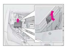
► Engine compartment: type B fuse box
