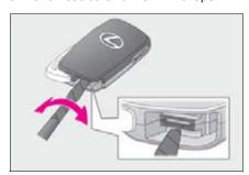
3 Remove the depleted battery.
