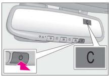
3 Drive the vehicle at 5 mph (8 km/ h) or less in a circle until a direction is displayed. If there is not enough space to drive in a circle, drive around the block until a direction is displayed.
