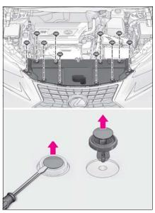
■ Installing the clips
