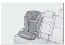
4 Sit the child in the child restraint system. Fit the seat belt to the child restraint system according to the manufacturer's instructions and insert the plate into the buckle.
