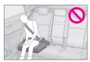
When a booster seat is installed, always ensure that the shoulder belt is positioned across the center of the child's shoulder. The belt should be kept away from the child's neck, but not so that it could fall off the child's shoulder.
