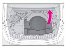
2 Loosen the center fastener that secures the spare tire.
