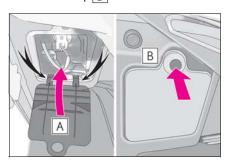
Install the engine compartment cover. (→P.347)
