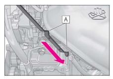
5 Holding a rag under the end, pull the dipstick out and check the oil level.
