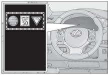
When a tab other than the driving assist system information is selected, only a recognized speed limit sign or do not enter sign (when notification is necessary) will be displayed.  $(\to P.89)$
