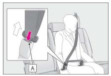
2 Insert the mechanical key (→P.106) or plate B into the notch of buckle and remove the belt.
