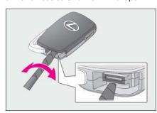
3 Remove the depleted battery.
