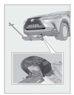
1 Remove the bolt **A** and then remove the cover **B**.
