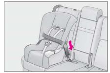
5 Fully extend the shoulder belt and allow it to retract to put it in lock
