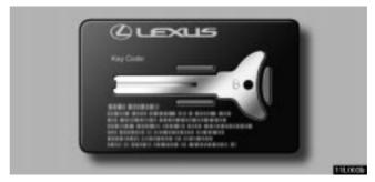
Since a transponder chip is not built in this flat key, you cannot start the engine with this key. Use this key to release the lock in case you accidentally lock your keys inside the vehicle or trunk.
