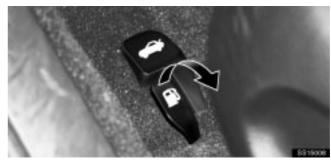
1. To open the fuel filler door, pull the lever up. When refueling, turn off the engine.
