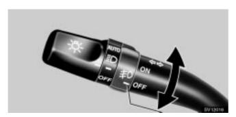
To turn on the fog lights, turn the switch to the "ON" position. The fog lights come on only when the headlights are on low beam.
