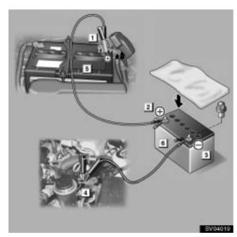
**▶** 5 Discharged battery 6 Booster battery
