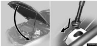
3. Hold the hood open by inserting the support rod into the slot.
