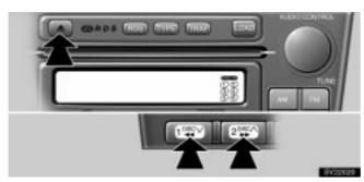
3. When ejecting one disc, select the disc you want to eject by the function button "DISC [2]" or "DISC [2]", and push the "EJECT" button briefly. When ejecting more than one disc, push and hold the "EJECT" button until a beep sounds and take out the disc ejected from the slot.
