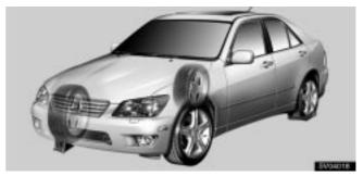
2. Block the wheel diagonally opposite the flat tire to keep the vehicle from rolling when it is jacked up.
