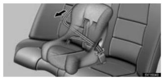
2. Fully extend the shoulder belt to put it in the lock mode. When the belt is then retracted slightly, it cannot be extended.
