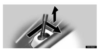
In case of unlocking the support rod, lift up the hood a little, move the support rod and unlock it as shown by the arrow marks in the illustration.
