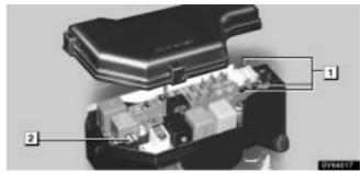
▶ Engine compartment 1 Spare fuses 2 Pull–out tool
