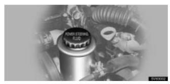
Check the fluid level on the dipstick. If necessary, add automatic transmission fluid DEXRON  $^{\rm @}{\rm II}$  or III.
