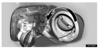
2. To remove the fuel tank cap, turn the cap slowly counterclockwise, then pause slightly before removing it. After removing the cap, hang the tether as shown in the illustration.
