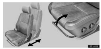
Hold the center of the lever and pull it up. Then slide the seat to the desired position with slight body pressure and release the lever.
