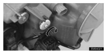
2. Turn the vertical movement adjusting bolt 2 the same number of turns and in the same direction at step 1.
