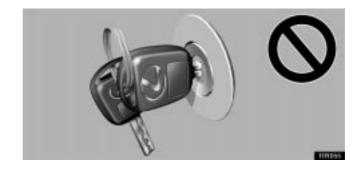
• When starting the engine, do not use the key with other transponder keys around (including keys of other vehicles) and do not press other key plates against the key grip. Otherwise the engine may not start, or may stop soon after it starts. If this happens, remove the key once and then insert it again after taking off other transponder keys (including keys of other vehicles) from the ring or while gripping or covering them with your hand to start the engine.
