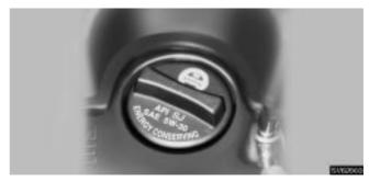
If the oil level is below or only slightly above the low level mark, add engine oil of the same type as already in the engine.
