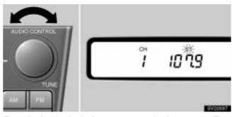
Turn the knob clockwise to step up the frequency. Turn the knob counterclockwise to step down the frequency.
