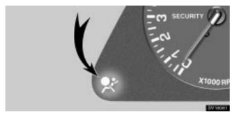
This front seat belt pretensioner system has a service reminder indicator to inform the driver of operating problems. If either of the following conditions occurs, this indicates a malfunction of the airbags or pretensioners. Contact your Lexus dealer as soon as possible to service the vehicle.
