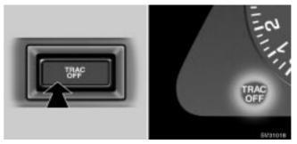
You can turn off the traction control system by pushing the "TRAC OFF" switch. The "TRAC OFF" indicator/warning light will then come on. Pushing the "TRAC OFF" switch a second time turns the system back on and extinguishes the "TRAC OFF" indicator/warning light.
