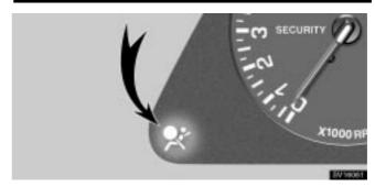
The indicator comes on when the ignition key is turned to the "ACC" or "ON" position. It goes off after about 6 seconds. This means the SRS airbags are operating properly.
