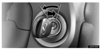
"LOCK" – Engine is off and the steering wheel is locked. The ignition key can be removed only at this position.
