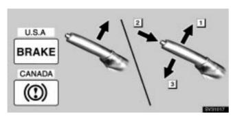
To set: Pull up the lever. For better holding power, first depress the brake pedal and hold it while setting the parking brake.
