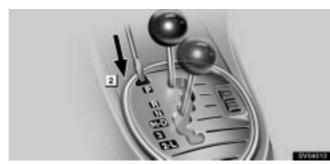
2 Insert your finger, the screwdriver or equivalent into the hole to push down the shift lock override button. You can shift the selector lever while pushing the button.
