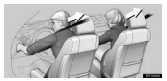
The driver and front passenger's seat belt pretensioners are designed to be activated in response to a severe frontal impact.
