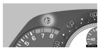
As the headlight beam level is always maintained automatically at the proper level in all loading conditions, your headlights do not dazzle other road users.
