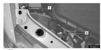
► 1 Vertical movement adjusting bolt 1
