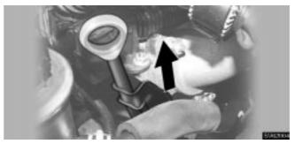
With the engine at operating temperature and turned off, check the oil level on the dipstick.
