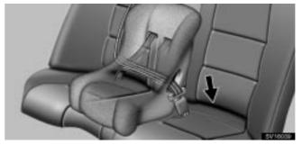
1. Run the lap and shoulder belt through or around the convertible seat following the instructions provided by its manufacturer and inserting the tab into the buckle taking care not to twist the belt. Keep the lap portion of the belt tight.
