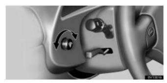
To adjust the brightness of the instrument panel lights, turn the knob.
