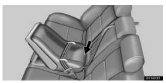
2. Fully extend the shoulder belt to put it in the lock mode. When the belt is then retracted even slightly, it cannot be extended.
