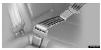
To connect the extender to the seat belt, insert the tab into the seat belt buckle so that the "PRESS" signs on the buckle release buttons of the extender and the seat belt are both facing outward as shown.
