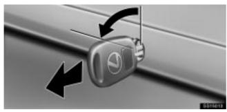
After closing the trunk lid, insert the master key and turn it counterclockwise to deactivate the lock release lever.
