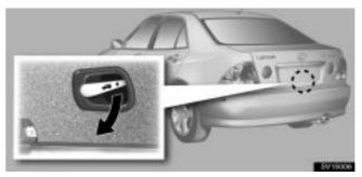
If a person is locked in the trunk, pull down the phosphorescent handle (illuminated for a while) on the inside of trunk lid in case of emergency to open the trunk lid.
