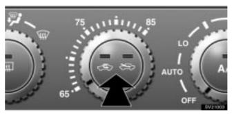
The air intake control button is used to switch the air intake between the OUTSIDE AIR mode and RECIRCULATED AIR mode.
