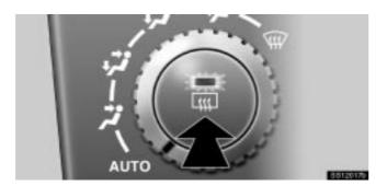
To turn the electric rear window defogger on, push the switch.
