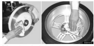
Before putting on the wheel, remove any corrosion on the mounting surfaces with a wire brush or such. Installation of wheels without good metal—to—metal contact at the mounting surface can cause wheel nuts to loosen and eventually cause a wheel to come off while driving.
