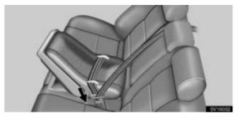
1. Run the lap and shoulder belt through or around the infant seat following the instructions provided by its manufacturer and inserting the tab into the buckle taking care not to twist the belt. Keep the lap portion of the belt tight.
