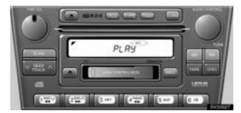
When you insert a cassette tape, the exposed tape should be to the right.
