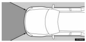
The SRS airbag system is designed to activate in response to a severe frontal impact within the shaded area between the arrows in the illustration.
