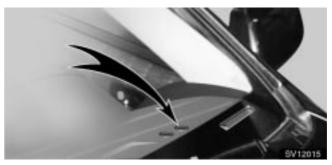
The automatic light control sensor is on top of the driver's side instrument panel.
