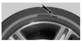
The spare tire with turning direction indicators is of a uni-directional type and is intended for use on the passenger side of the vehicle.
