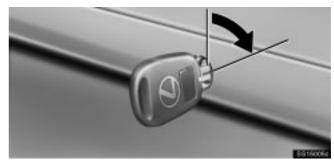
To unlock the trunk lid, insert the master key and turn it clockwise.
