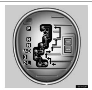
★ Shift while pressing the brake pedal. (Ignition switch must be in the "ON" position.)
