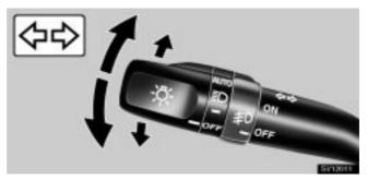
For signaling turns, move the lever up or down in the conventional manner.
