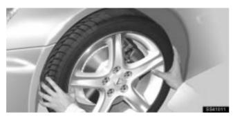
**7.** Remove the wheel nuts and remove the flat tire. Lift the flat tire straight off and put it aside.
