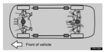
When jacking up your vehicle with the jack, position the jack correctly as shown in the illustration.
