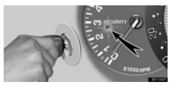
The engine immobiliser system is a theft prevention system. When you insert the key in the ignition switch, the transponder chip in the key's head transmits an electronic code to the vehicle. The engine will start, only when the electronic code in the chip corresponds to the registered ID code for the vehicle.
