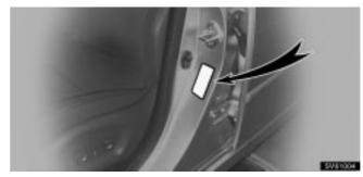
The recommended cold tire pressures, tire size and the vehicle capacity weight are given on the label.
