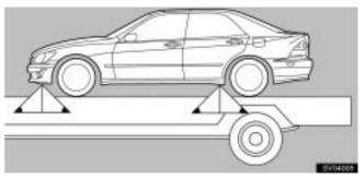
If you use chains or wires to tie down your vehicle, the angles shaded black must be at  $45^{\circ}.$
