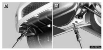
If your Lexus is transported by a flat bed, it should be tied down at locations A and B as shown above.
