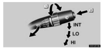
▶ 1 Interval adjuster 2 Washer on
