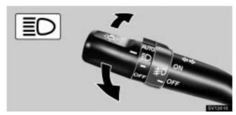
For high beam, push the lever forward. Pull it back for low beam. For the headlight flasher, pull it further back.
