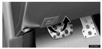
1. To open the hood, pull the hood lock release lever under the instrument panel. The hood will spring up slightly.
