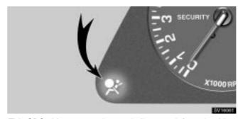
This SRS airbag system has an indicator to inform the driver of operating problems. If either of the following conditions occurs, this indicates a malfunction of the airbags. Contact your Lexus dealer as soon as possible to service the vehicle.
