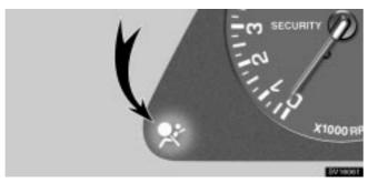
This indicator comes on when the ignition key is turned to the "ACC" or "ON" position. It goes off after about 6 seconds. This means the front seat belt pretensioners are operating properly.
