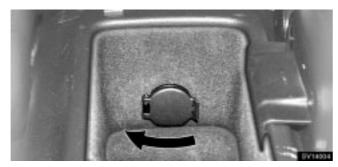
The power outlet is designed for power supply for car accessories.
