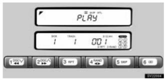
In the "TAPE" or "CD" mode, the applicable functions are shown in the lowest part of the display. Push the switch just below to turn on each function.
