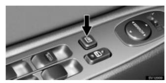
With the window lock switch pressed in, only the driver's window can be raised or lowered.
