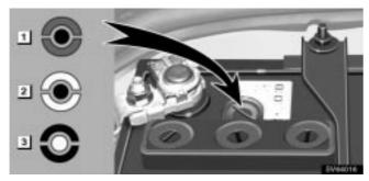
Check the battery condition by the hydrometer color.
