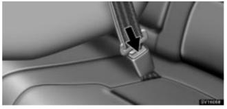
4. To remove the convertible seat, press the buckle–release button and allow the belt to retract completely. The belt will move freely again and be ready to work for an adult or older child passenger.
