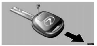
1. Remove the screw, and then the cover while pushing it in the arrow direction.
