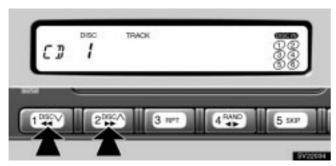
Push the "DISC  $\[ \]$ " or "DISC  $\[ \]$ " button to select the disc number.
