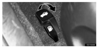
To open the trunk lid from the driver's seat, pull up on the lock release lever.
