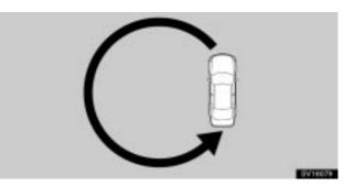
Drive the vehicle slowly (at 8 km/h (5 mph) or lower) in a circle until the direction is displayed. If there is not enough space to drive in a circle, drive around the block until the direction is displayed.
