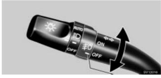
To turn on the front fog lights, turn the switch to the "ON" position. The front fog lights come on only when the headlights are on low beam.
