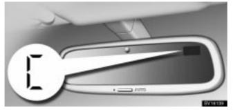
"C" appears on the display in case the circling calibration is required due to a drastic change in the magnetic field. To rectify this, follow the calibration procedure below.
