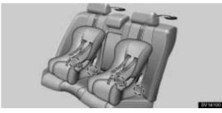
The lower anchorages for the child restraint system interfaced with the FMVSS225 specification are installed in the rear seat.
