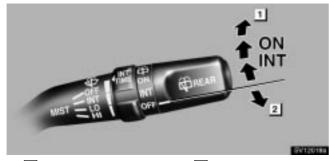
▶ 1 Washer on during wiping 2 Washer on
