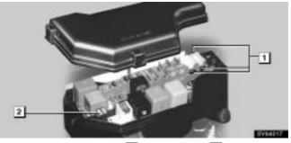
► Engine compartment 1 Spare fuses 2 Pull-out tool
