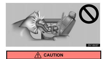
• Never install a rear-facing child restraint system on the front passenger seat. In the event of an accident, the force of the rapid inflation of the front passenger airbag can cause death or serious injury to the child if the rear-facing child restraint system is installed on the front passenger seat.
