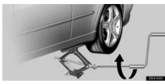
5. After making sure no one is in the vehicle, raise it high enough so that the spare tire can be installed.
