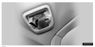
Insert these tabs in the hollow of the seat belt cover, pull it up and hook it while pressing the "Push" mark. 3
