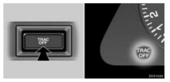
If your wheels get stuck in a ditch when you are driving on a severe off road and sand, turn off the traction control system. This system that controls engine performance interferes with the process of freeing your wheels.
