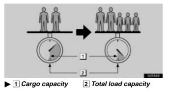
In case that 2 people with the combined weight of 166 kg (366 lb.) are riding in your vehicle with the total load capacity of 390 kg (860 lb.), the available amount of cargo and luggage load capacity will be as follows:
