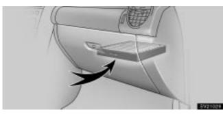
The air conditioning filter is behind the glove box.
