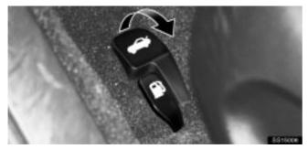
To open the trunk lid from the driver's seat, pull up on the lock release lever.
