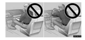
• Do not sit on the edge of the seat or lean against the dashboard when the vehicle is in use, since the front passenger airbag could inflate with considerable speed and force. Anyone who is up against, or very close to, an airbag when it inflates, can be killed or seriously injured. Sit up straight and well back in the seat, and always use your seat belt properly.
