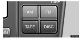
Push "AM", "FM", "TAPE" or "DISC" to turn on that mode. The selected mode turns on directly.
