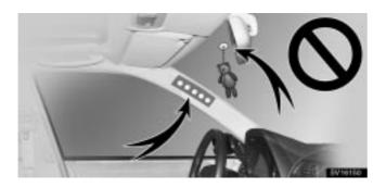
Do not attach a microphone or any other device or object around the area where the curtain shield airbag activates such as on the windshield glass, side door glass, front and side pillars, roof side rail and assist grips. When the curtain shield airbag inflates, the microphone or other device or object will be thrown away with great force or the curtain shield airbag may not activate correctly, resulting in death or serious injury.
