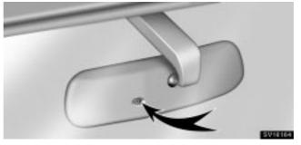
To ensure correct functioning of an anti-glare mirror sensor located on the back side of the mirror, do not touch or cover the sensor with your finger or a piece of cloth, etc.
