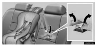
8. Fix the child restraint system with the seat belt.
