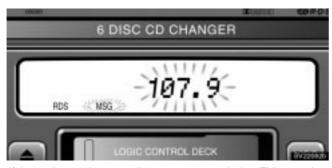
If the radio receives a radio text message during FM reception, "MSG" and a text message appears on the display. After the text message goes off, "MSG" also goes off.
