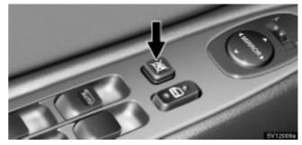
With the window lock switch pressed in, only the driver's window can be raised or lowered.
