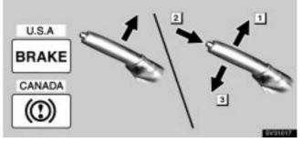
To set: Pull up the lever. For better holding power, first depress the brake pedal and hold it while setting the parking brake.
