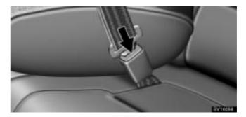
2. To remove the child restraint system, press the buckle-release button and allow the belt to retract.
