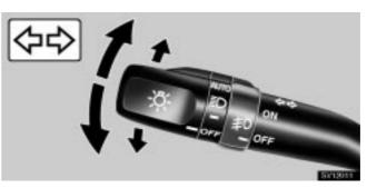
For signaling turns, move the lever up or down in the conventional manner.
