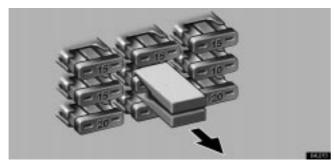
2. Make sure the inoperative component is turned off. Pull the suspected fuse straight out with the pull-out tool and check it. If it has blown, push a new fuse into the clips.
