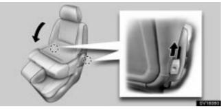
Return the seatback to the up-right position. Pull up the side levers and fold the seatback down.
