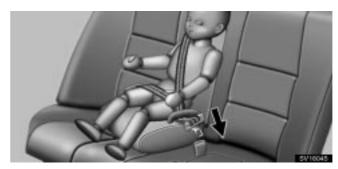
1. Sit the child on a booster seat. Run the lap and shoulder belt through or around the booster seat and child following the instructions provided by its manufacturer and insert the tab into the buckle taking care not to twist the belt.
