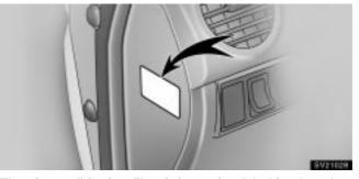
The air conditioning filter information label is placed on the driver side of the instrument panel as shown and indicates that a filter has been installed.
