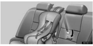
3. Fix the child restraint system with the seat belt.
