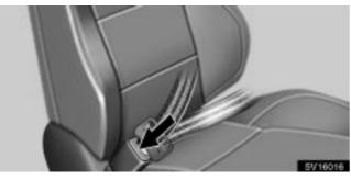
To release the belt, press the buckle release button and allow the belt to retract.
