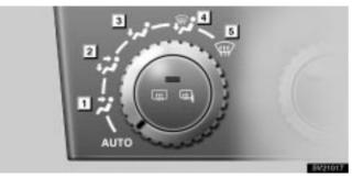
The outlets from which air is delivered can be selected manually by pushing the button. The function of each mode is as follows:
