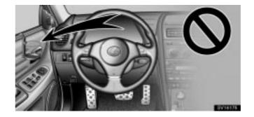
• Do not attach a cup holder or any other device or object on or around the door. When the side airbag inflates, the cup holder or any other device or object will be thrown with great force, or the side airbag may not activate correctly, resulting in death or serious injury. Likewise, the driver and front passenger should not hold objects in their arms or on their knees.
