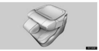
You can use the front passenger's seatback as a temporary table only when the vehicle is stopped.
