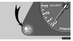
The indicator comes on when the ignition switch is turned to the "ACC" or "ON" position. It goes off after about 6 seconds. This means the SRS side airbags and curtain shield airbags are operating properly.
