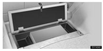
The warning reflector is in the auxiliary box.
