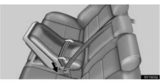
1. Run the lap and shoulder belt through or around the infant seat following the instructions provided by its manufacturer and insert the tab into the buckle taking care not to twist the belt. Keep the lap portion of the belt tight.
