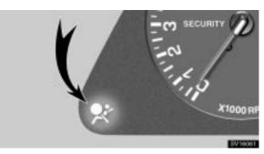
This indicator comes on when the ignition switch is turned to the "ACC" or "ON" position. It goes off after about 6 seconds. This means the seat belt pretensioners are operating properly.
