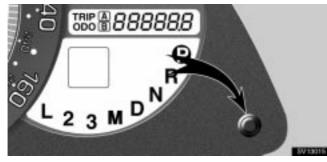
This meter displays the odometer and two trip meters. To change the mode indication, push the "ODO/TRIP" knob briefly. Each time you push the knob, the mode changes in order from the odometer to trip meter A to trip meter B, then back to the odometer, etc.
