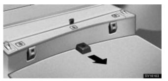
**TO USE THE CENTER ANCHOR BRACKET** 1. Remove the cover of the center anchor bracket.
