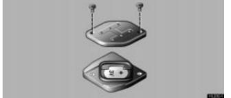
3. Remove the 2 screws to take out the lid of the module.
