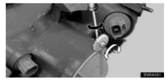
1. Turn the vertical movement adjusting bolt 1 in either direction. At this time, keep the turning direction and number of turns in mind.
