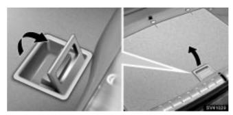
TO USE THE ANCHOR BRACKET 1. Pull up the deck board.
