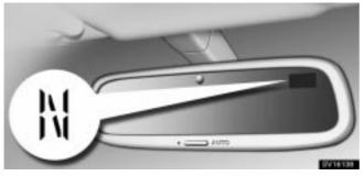
The compass indicates the direction in which the vehicle is heading. The illustration shown above indicates the vehicle is heading north.
