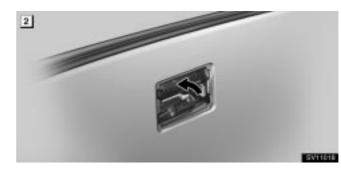
2. Pull up the lever and open the back door.
