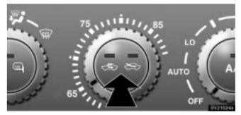
The air intake control button is used to switch the air intake between the OUTSIDE AIR mode and RECIRCULATED AIR mode.
