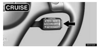
To operate the cruise control, push the main switch. This turns the system on. The indicator light in the instrument cluster shows that you can now set your desired cruising speed. Another push on the switch will turn the system completely off.
