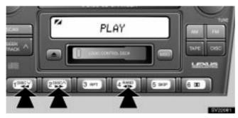
"Program" button: Push the "  $\triangleleft \mid \triangleright$  " button to select the other side of a cassette tape. The display indicates which side is currently selected ( $\blacktriangle$  indicates top side,  $\blacktriangledown$  indicates bottom side).
