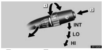
▶ 1 Interval adjuster 2 Washer on
