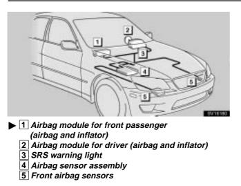
The SRS front airbag system consists mainly of the above components, and their locations are shown in the illustration.
