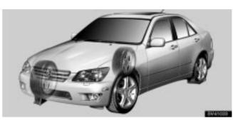
2. Block the wheel diagonally opposite the flat tire to keep the vehicle from rolling when it is jacked up.
