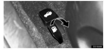
1. To open the fuel filler door, pull the lever up.
