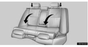
Lower the head restraints to the lowest position, unlock the seatbacks by pushing the lock release button on the side of the seatback and fold them down.
