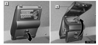
2. Pull the lever, lift the cover (b) up and fix it to the upper part of the trunk using the magnet attached on the cover (b).
