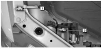
1 Vertical movement adjusting bolt 1
