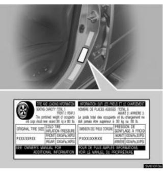
The recommended cold tire inflation pressure, tire size and the combined weight of occupants and cargo (vehicle capacity weight) are described on the tire and loading information label.
