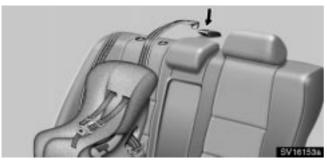
2. Fix the child restraint system with the seat belt.
