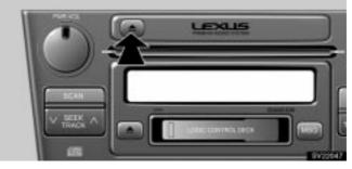
To eject the compact disc, push the "EJECT" button.
