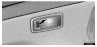
To turn on the luggage compartment light, open the back door or push the switch. Closing the back door will turn the light off.
