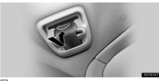
3 Insert these tabs in the hollow of the seat belt cover, pull it up and hook it while pressing the "PUSH" mark.
