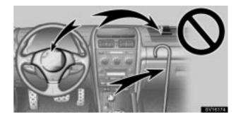
• Do not put anything or any part of your body on or in front of the dashboard or steering wheel pad that houses the front airbag system. They might restrict inflation or cause death or serious injury as they are projected rearward by the force of the deploying airbags. Likewise, the driver and front passenger should not hold objects in their arms or on their knees.
