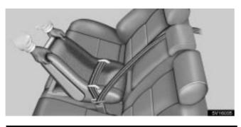
Push and pull the child restraint system in different directions to be sure it is secure. Follow all the installation instructions provided by its manufacturer.
