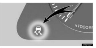
The slip indicator light comes on for a few seconds when the ignition key is turned to "ON". If the indicator light does not come on when the ignition is turned on, contact your Lexus dealer.
