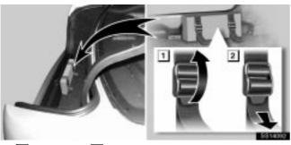
▶ 1 To loosen 2 To tighten
