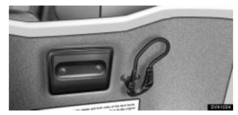
When closing the board, replace the hook also in its original position as shown.
