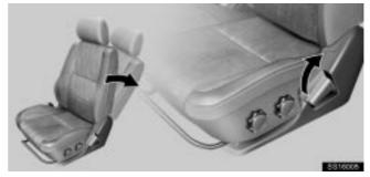
Lean forward and pull the lever up. Then lean back to the desired angle and release the lever.
