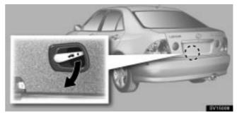
If a person is locked in the trunk, he/she can pull down the phosphorescent handle on the inside of trunk lid to open the trunk lid.
