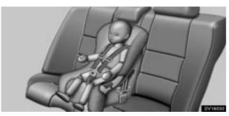
A convertible seat must be used in forward-facing or rear-facing position depending on the age and size of the child. When installing, follow the manufacturer's instructions about the appropriate age and size of the child as well as directions for installing the child restraint system.
