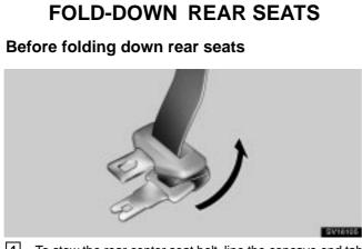
1 To stow the rear center seat belt, line the concave end tab upon the round end tab.
