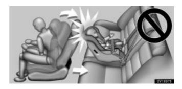
If the driver's seat position does not allow sufficient space for safe installation, install the child restraint system on the rear right seat.
