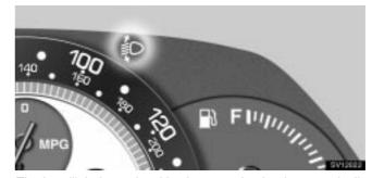
The headlight beam level is always maintained automatically at the proper level in all loading conditions so that your headlights do not dazzle other road users.
