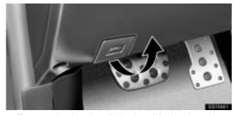
1. To open the hood, pull the hood lock release lever under the instrument panel. The hood will spring up slightly.
