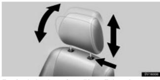
To raise the head restraint, pull it up. To lower it, press the lock release button and push the head restraint down. To move the head restraint forward or rearward, pull or push on the top.
