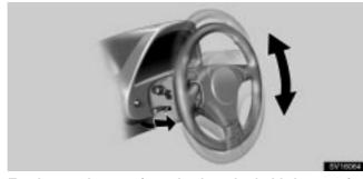
To change the steering wheel angle, hold the steering wheel, pull the lock release lever toward you, tilt the steering wheel to the desired angle and release the lever.
