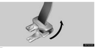
1 To stow the rear center seat belt, line the concave end tab upon the round end tab.
