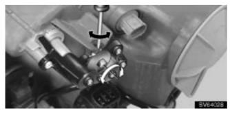
2. Turn the vertical movement adjusting bolt 2 the same number of turns and in the same direction as step 1.
