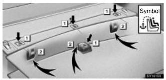
▶ 1 Symbol mark 2 Anchor bracket Use the anchor bracket located behind the rear seat on the
