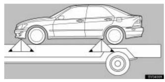
If you use chains or wires to tie down your vehicle, the angles shaded black must be at 45°.
