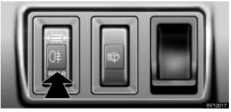
To turn on the rear fog lights, push the switch. They will come on when the headlights are turned on.
