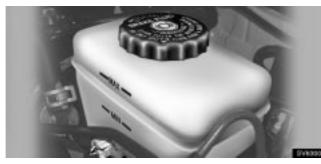
To check the fluid level, simply look at the see-through reservoir. The level should be between the "MAX" and "MIN" lines on the tank.
