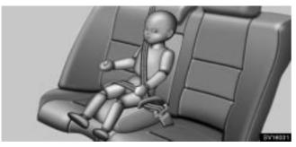
A booster seat must be used in forward-facing position only.
