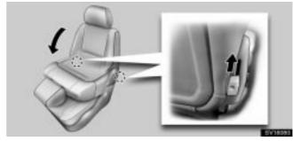
Return the seatback to the up-right position. Pull up the side levers and fold the seatback down.
