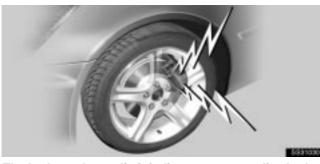
The brake pad wear limit indicators on your disc brakes give a warning noise when the brake pads are worn to the extent that replacement is required.
