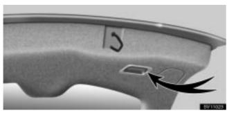
When closing the back door, the inside handle can be used to make the reach easier.
