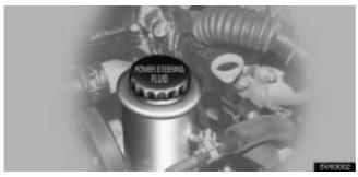
Check the fluid level on the dipstick. If necessary, add automatic transmission fluid  $\text{DEXRON}^{\textcircled{B}}\text{II}$  or III.
