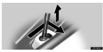
In case of unlocking the support rod, lift up the hood a little, move the support rod and unlock it as shown by the arrow marks in the illustration.
