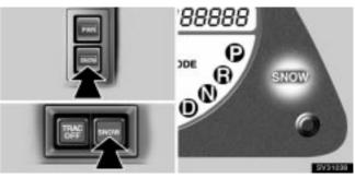
You can select the snow mode by pushing the "SNOW" switch. The "SNOW" indicator light will come on.
