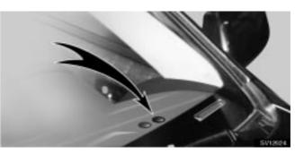
The automatic light control sensor is on top of the driver's side instrument panel.
