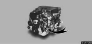
The engine number is stamped on the engine block as shown.
