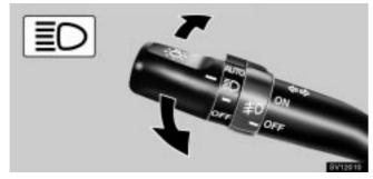
For high beam, push the lever forward. Pull it back for low beam. For the headlight flasher, pull it further back.
