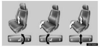
Move the control switch in the desired direction. Releasing the switch will stop the seat cushion in that position. Folding down front passenger's seatback
