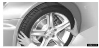
**6.** Remove the wheel nuts and remove the flat tire. Lift the flat tire straight off and put it aside.
