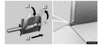
5. Remove the lock pins fixed on both sides of the center deck board in the order shown above, and lower the center deck board to the lowest position. Then fix the lock pin.
