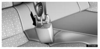
To release the concave end tab, insert the key into the hole on buckle (with light gray buckle-release button ) and allow the belt to retract.
