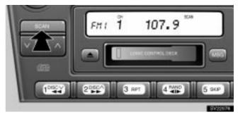
**To scan the preset stations:** Push the "SCAN" button until you hear a beep. "SCAN" appears on the display. The radio will tune in the next preset station up the band, stay there for a few seconds, and then move to the next preset station. To select a station, push the "SCAN" button a second time.
