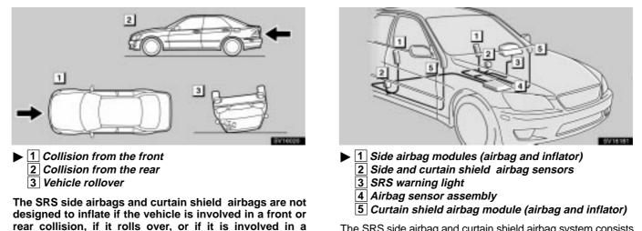
The SRS side airbag and curtain shield airbag system consists mainly of the above components, and their locations are shown in the illustration.
