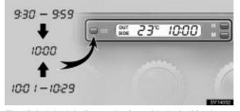
The digital clock indicates the time with the ignition key at the "ACC" or "ON" position. To reset the hour, press the "H" button. To reset the minutes, press the "M" button. To adjust the time to the nearest hour, press the ":00" button.
