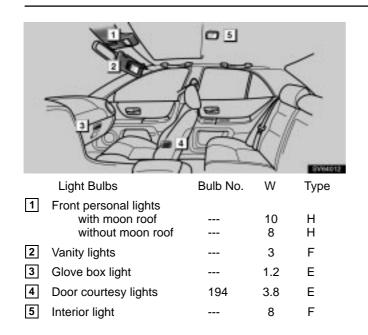
A: HB3 halogen bulbs B: D2R discharge bulbs C: H3 halogen bulbs D: Wedge base bulbs (amber) E: Wedge base bulbs F: Double end bulbs G:Single end bulbs (amber) H: Single end bulbs 03 07.09
