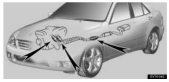
Three-way catalytic converters are emission control devices installed in the exhaust system.
