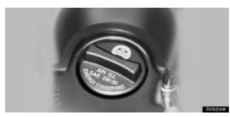
If the oil level is below or only slightly above the low level mark, add engine oil of the same type as already in the engine.
