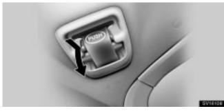
To use the rear center seat belt, press "PUSH" mark and pull out the tabs.
