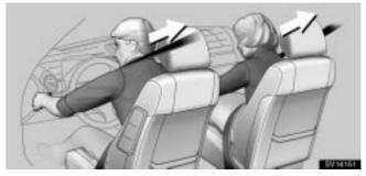
The driver and front passenger's seat belt pretensioners are designed to be activated in response to a severe frontal impact.
