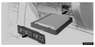
2. Remove the cover and take out the air filter
