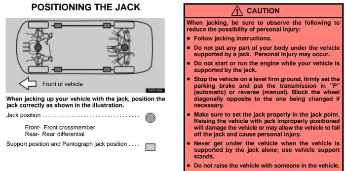
• When raising the vehicle, do not place any objects on top of or underneath the jack.
