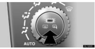
To turn the electric rear window defogger on, push the switch.
