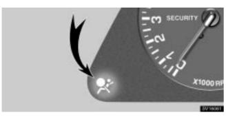
The indicator comes on when the ignition switch is turned to the "ACC" or "ON" position. It goes off after about 6 seconds. This means the SRS front airbags are operating properly.
