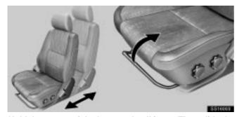
Hold the center of the lever and pull it up. Then slide the seat to the desired position with slight body pressure and release the lever.
