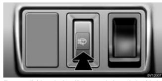
To spray fluid on the headlights, push the switch with the headlights on.
