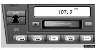
**To scan all the frequencies:** Push the "SCAN" button briefly. "SCAN" appears on the display. The radio will find the next station up the band, stay there for a few seconds, and then scan again. To select a station, push the "SCAN" button a second time.
