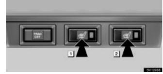
▶ 1 For driver's seat 2 For front passenger's seat
