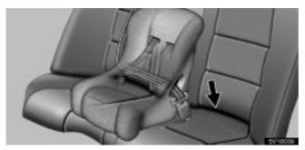
1. Run the lap and shoulder belt through or around the convertible seat following the instructions provided by its manufacturer and insert the tab into the buckle taking care not to twist the belt. Keep the lap portion of the belt tight.
