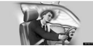
The SRS (Supplemental Restraint System) side airbags and curtain shield airbags are designed to provide further protection for the driver and front passenger in addition to the primary safety protection provided by the seat belts.
