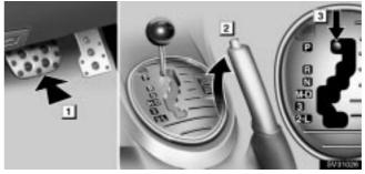
1 Brake pedal 2 Parking brake lever
