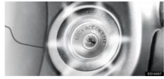
For easy access to the ignition switch, the ignition switch light comes on when any of the doors are opened.
