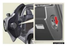
The door cannot be opened from inside the vehicle when the locks are set.
