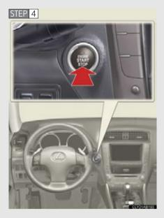
Press the "ENGINE START STOP" switch.
