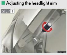
Turn bolt A in either direction using a Phillips-head screwdriver.
