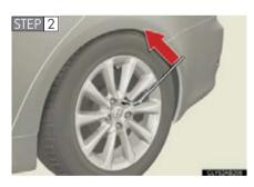
Slightly loosen the wheel nuts (one turn).
