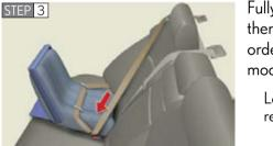
Fully extend the shoulder belt and then allow it to retract slightly in order to activate the ALR lock mode.
