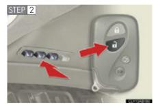
While the desired button ("1", "2" or "3") press **3** on the wireless remote control until the signal beeps.
