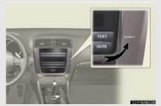
Close the doors, trunk and hood, and lock all doors. The system will be set automati-
