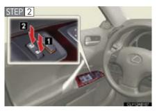
Shift the shift lever to P or N, and press and hold the driver's door lock switch (■ or ⊇) for approximately 5 seconds and then release.
