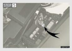
Remove the fuse with the pullout tool.
