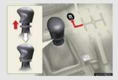
Shift the shift lever into the R position while lifting up the ring section.
