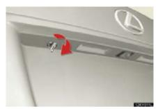
Turn the mechanical key clockwise to open.
