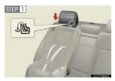
Secure the child restraint using a seat belt or a lower anchors, and lock the head restraint in place at the original position.
