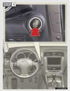
Press the "ENGINE START STOP" switch.
