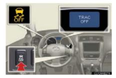
Push and hold the button for more than 3 seconds while the vehicle is stopped to turn off TRAC and VSC.
