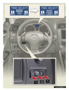
Tire pressure warning valve and transmitter ID code settings display
