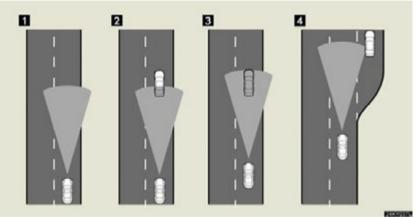
Example of constant speed cruising (when there are no vehicles ahead): When set to 62 mph (100 km/h)
