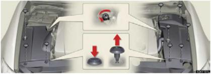
Installing the clips
