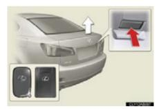
Press the button to unlock the trunk.
