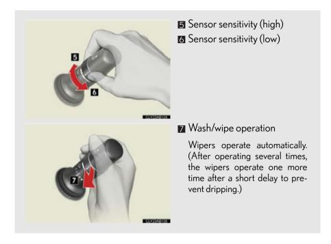
The windshield wiper and washer can be operated when
