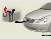
Lift the auxiliary catch lever and lift the hood.
