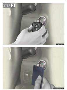
Touch the Lexus emblem side of the electronic key to the "ENGINE START STOP" switch.
