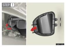
Release the lock and remove the cover.
