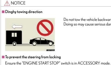
Do not tow the vehicle backwards. Doing so may cause serious damage.
