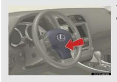
To sound the horn, press on or close to the **b** mark.
