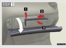
Open the glove box. Lift and remove the partition.
