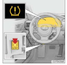
**5** Wait for a few minutes with the engine switch in IGNITION ON mode and then turn the engine switch off.
