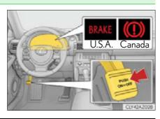
■ Parking brake engaged warning buzzer →P. 464
