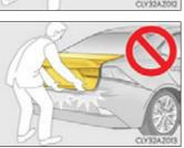
Do not attach any accessories other than genuine Lexus parts to the trunk lid. Such additional weight on the trunk lid may cause the lid to suddenly shut again after it is opened.
