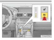
The seat ventilators can be used when the engine switch is in IGNITION ON mode.
