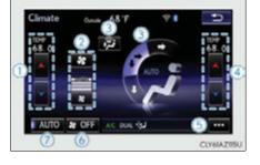
To adjust or select settings, move the Remote Touch knob to select the screen button, and then press the Remote Touch knob to enter the selected function.
