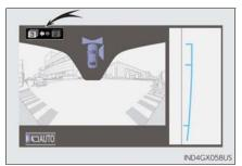
When in 3 screen mode, you can change the display from the simultaneous display to each individual display.
