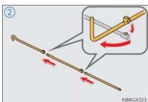
3 Assemble the jack handle extension bar and the jack handle and tighten the screw.
