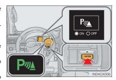
When the sensors detect an obstacle, a graphic is shown on the multi-information display, multimedia screen (if equipped) and navigation system screen (if equipped) depending on the position and distance to the obstacle.
