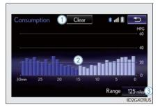
Average fuel consumption for the past 30 minutes is divided by color into past averages and averages attained since the engine switch was last turned to IGNITION ON mode. Use the displayed average fuel consumption as a reference.
