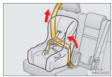
6 If the child restraint has a top tether strap, the top tether strap should be latched onto the top tether strap anchor.  $(\rightarrow P. 67)$
