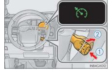
When in constant speed control mode, to return to vehicle-to-vehicle distance control mode, push the lever forward again and hold for approximately 1 second.
