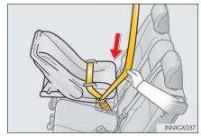
While pushing the child restraint system down into the seat, allow the shoulder belt to retract until the child restraint system is securely in place.
