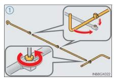
2 Assemble the jack handle extension bar and the jack handle bar and tighten the bolts.
