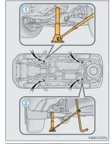
6 Raise the vehicle until the tire is slightly raised off the ground.
