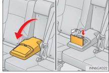
Pull the armrest down, and then press in and release the button.
