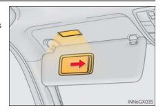
If the vanity lights remain on when the engine switch is turned off, the lights will go off automatically after  $20 \, \text{minutes}$ .
