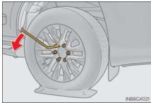
Remove the jack handle, jack handle extension bar and jack handle bar from the tool box and assemble by following these steps.
