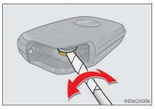
Remove the depleted battery.
