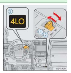
Lock the center differential when your vehicle's wheels get stuck in a ditch or when driving on a slippery or bumpy surface.
