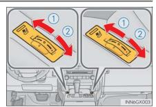
The seat heaters and ventilators can be used when the engine  $\overline{\text{switch}}$  is in IGNITION ON mode.
