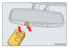
Programming has completed when the indicator light changes to a rapid flash.
