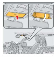
To use the overhead console when the conversation mirror is open, further extend the lid.  $(\rightarrow P.414)$
